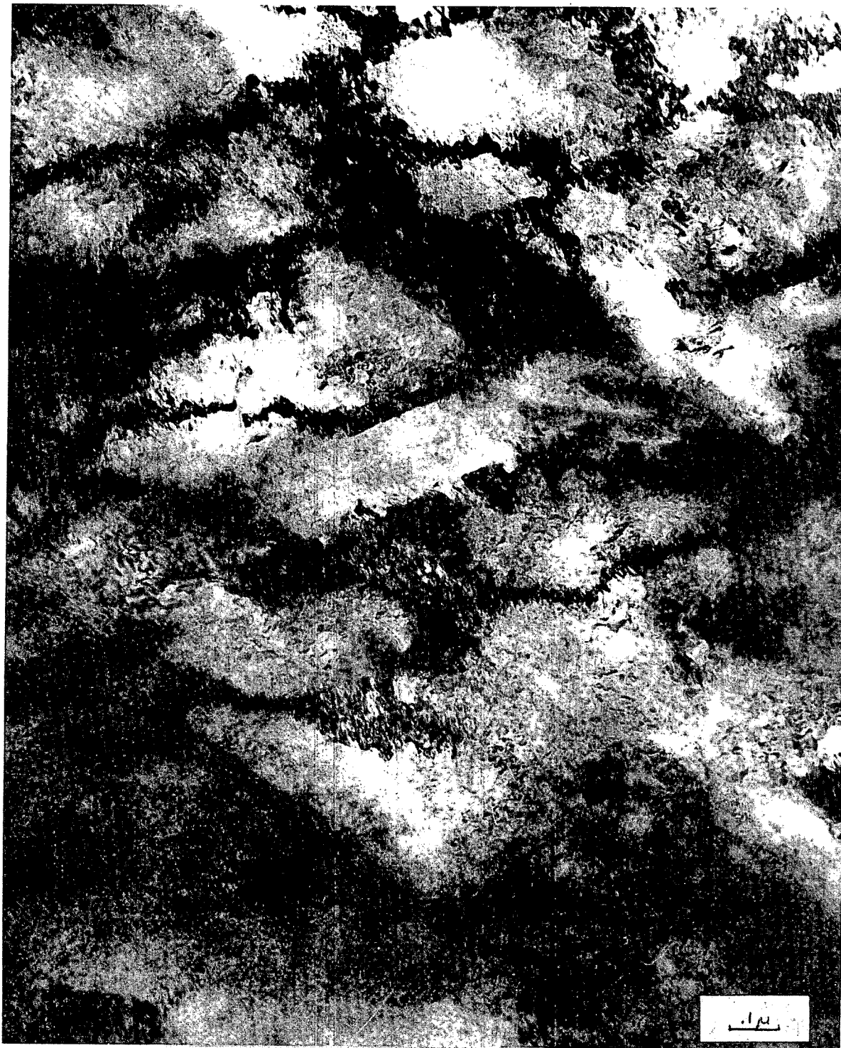
FIGURE 157. Highly damaged surface of annealed 316 stainless steel specimen resulting from mechanical abrasion.
