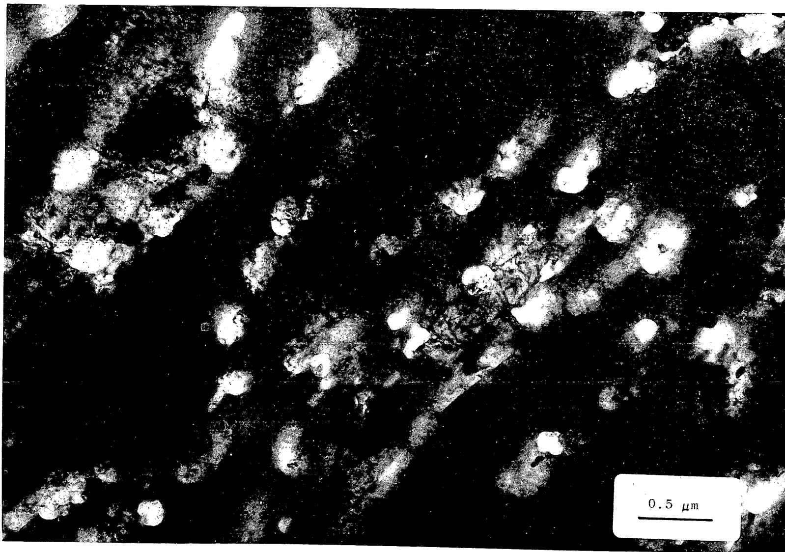
FIGURE 115. Micrograph of specimen of HT-9 ion bombarded to 400 dpa at 500°C showing dislocation structure precipitates and voids in a thin section of the specimen. Note the frequent association between precipitates and voids.
