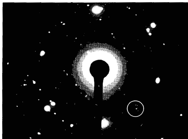
FIGURE 104. A typical diffraction pattern obtained from D21 STA irradiated (~55 dpa) at 750°C.
