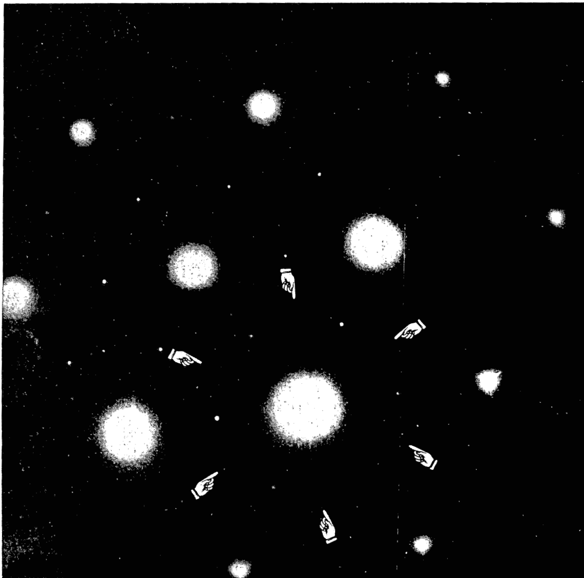
FIGURE 35. Selected area \langle 111 \rangle electron diffraction pattern from STA Inconel 718 after neutron irradiation to 5 \times 10^{22} \text{ n/cm}^2 ( E > 0.1 \text{ MeV} ) at 454^\circ\text{C} . The weak reflections indicated correspond to \{20\bar{2}0\} planes of hexagonal eta phase platelets in the plane of the specimen. Compare with Figure 20.
