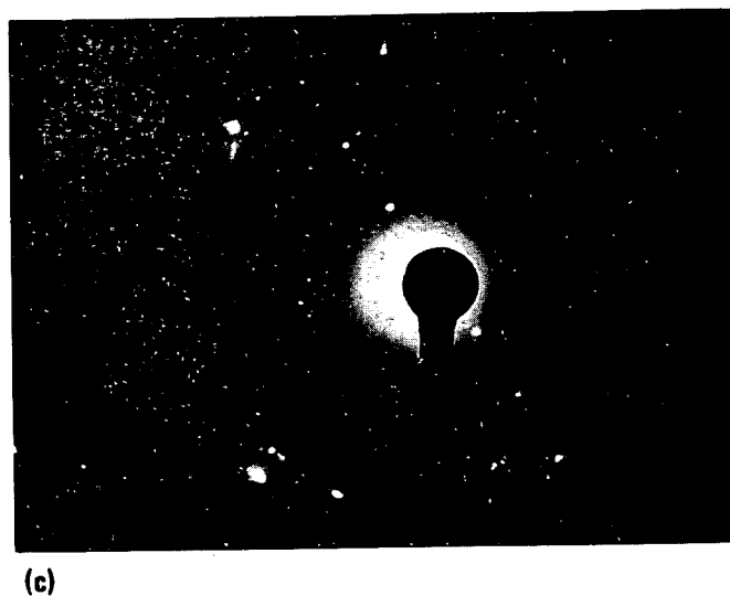
FIGURE 107(c). Diffraction pattern of a typical area in D25 STA irradiated ( \sim 55 dpa) at 750^{\circ}\text{C} .
