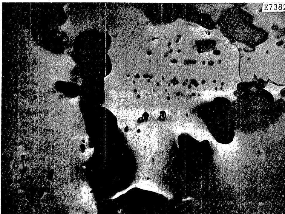
FIGURE 114. Alloy D9: 1100°C, 15 minutes, 25% CW, 750°C, 100 hours. TEM micrograph (Magn. X45,000).
