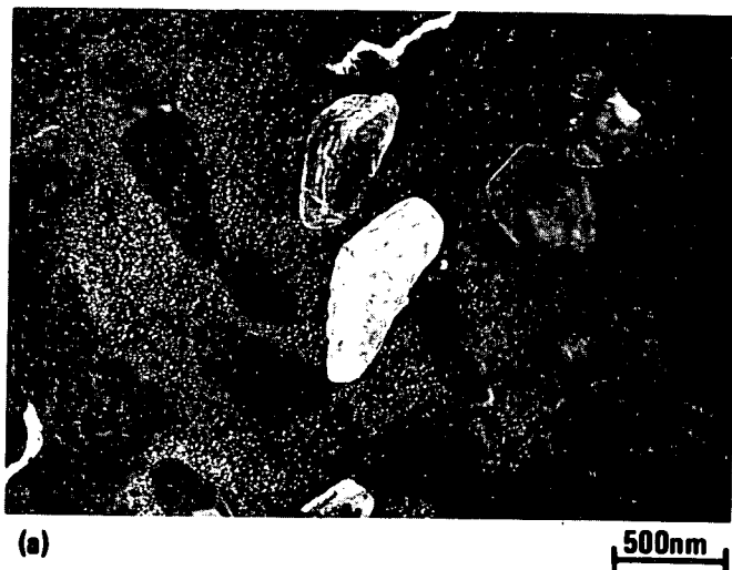
FIGURE 105(a). Dark field micrograph of precipitates in D21 STA irradiated (~55 dpa) at 750°C imaged by using spot under circle in Fig. 105(b).
