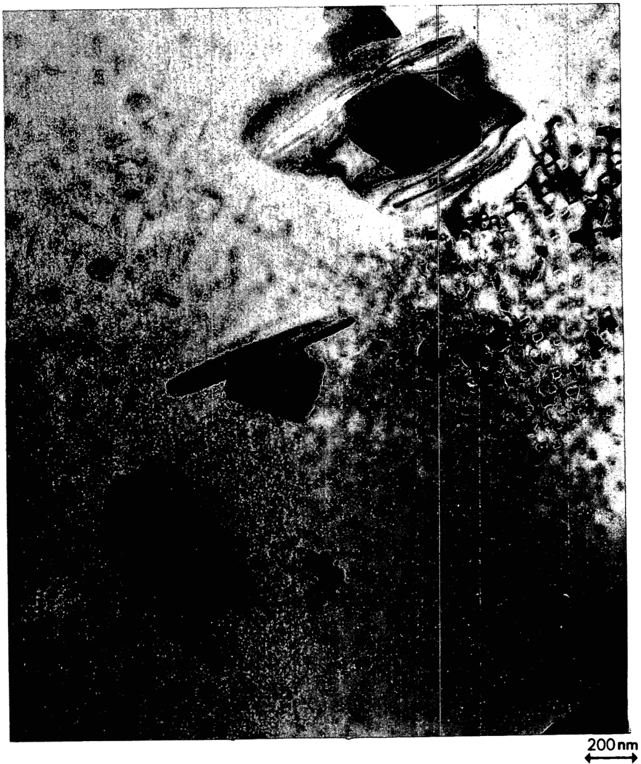
FIGURE 130. Delta phase precipitation on carbides in the \gamma'/\gamma'' class of alloys.
