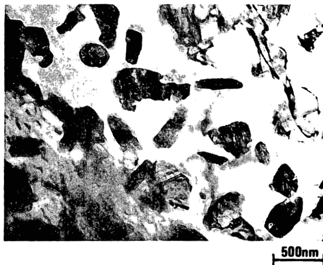
FIGURE 103. Dark field micrograph of precipitates in D21 STA irradiated (~55 dpa) at 750°C.
