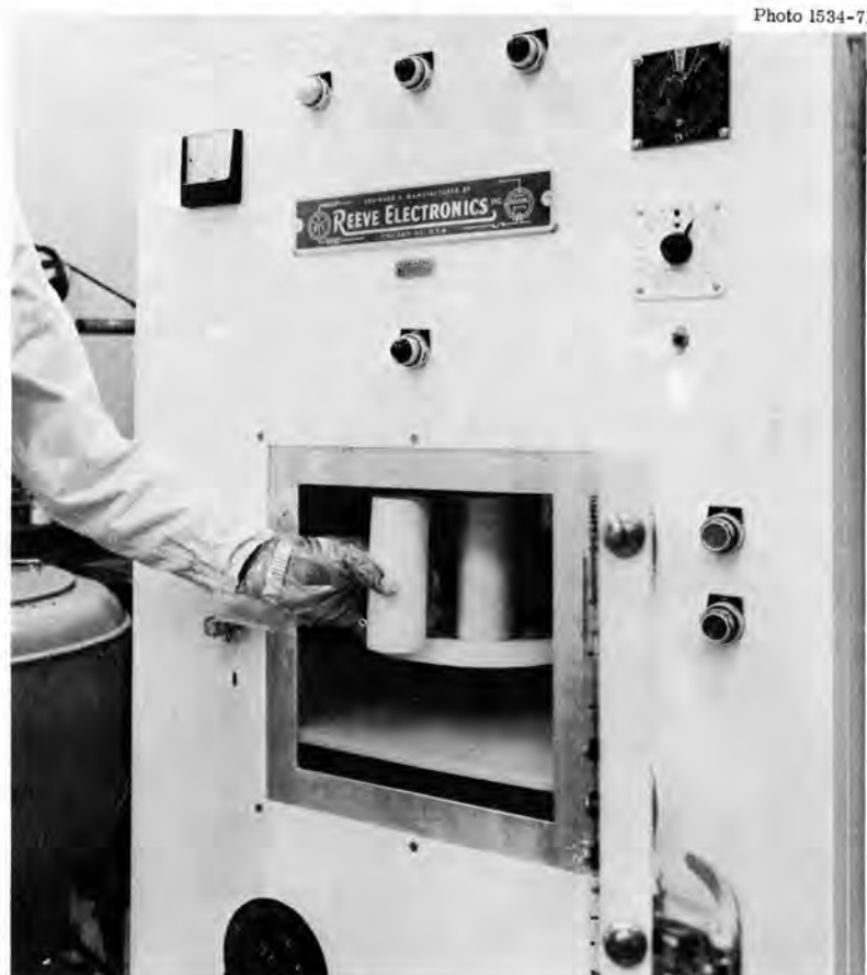
Fig. 6. Microwave Oven Used to Dry Uranate Samples. A sample is being removed from the rotating table.
