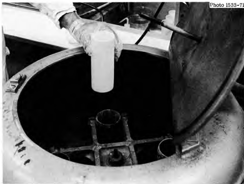
Fig. 5. Centrifuge Used for Separating Uranate from Another Liquor.
