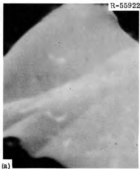
Fig. 10. Sample A-5331-97A. (a) Smooth crystalline portion. 8500X. (b) Fluffy portion. 30,000X.
