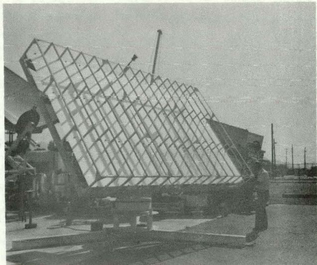
Fig. 6 The array without the Fresnel lenses or the liquid coolant manifold mounted. The large alumi- num sheet is the heat sink for the passive coolant mode; the cells are bonded directly to this sink.
