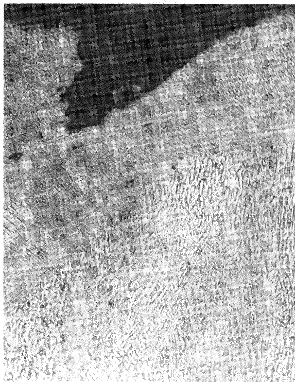
Figure D-22 Macrograph of Section Through Pore at 14.75 in. ID in 10K17L, 100x
