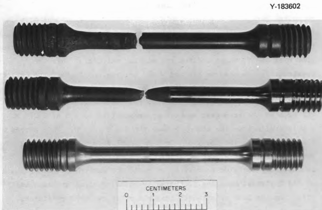
Fig. 10. Different fracture modes. Bottom specimen is untested, middle one is a high-ductility fracture in the 2 1/4 Cr-1 Mo steel base metal, and the top is a low-ductility failure near the fusion line.
