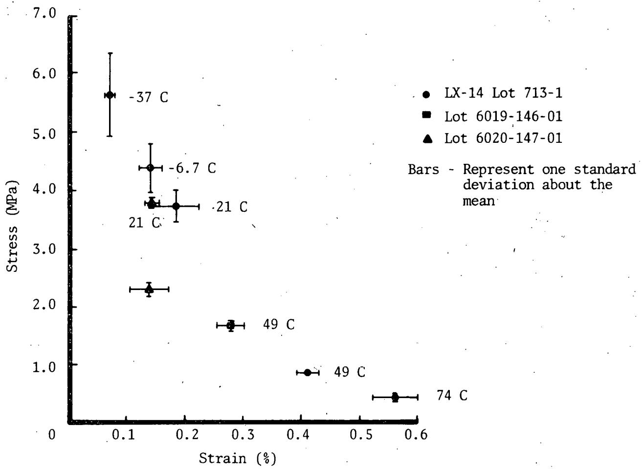
Fig. 1. Stress/Strain at Failure
