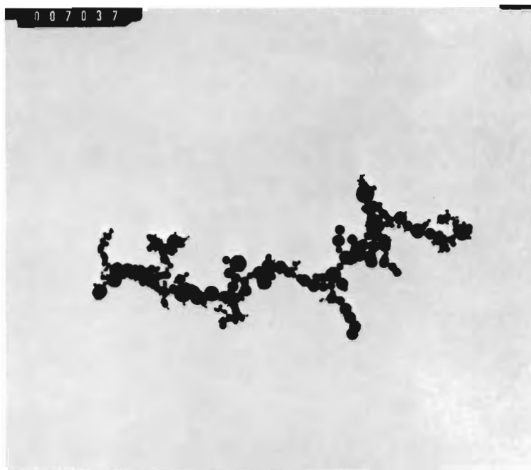
FIGURE 2.4. Transmission Electron Micrograph Showing the Structure of a \text{PuO}_2\text{-UO}_2 Aggregate Which has been Deposited on a Carbon-Coated Copper Grid by a Point-to-Plane Electrostatic Precipitator. The chain-like structure is typical of the condensation aerosols of metal oxides.
