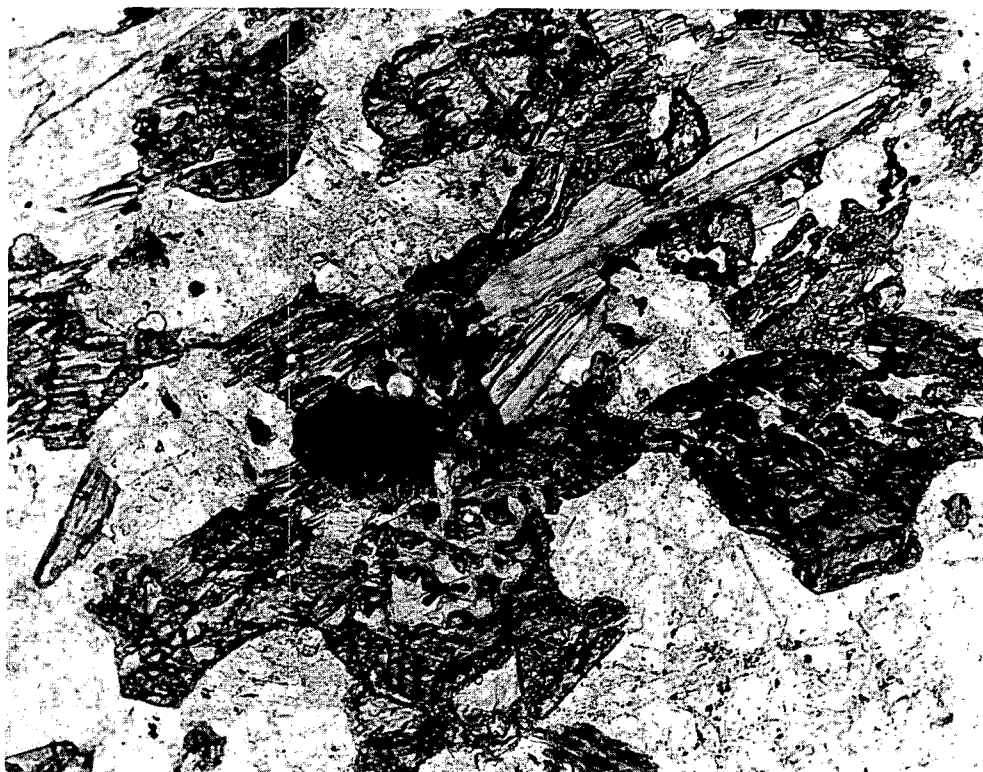
Fig. 7. Euhedral amphibole altered along cleavages to chlorite or talc, in mafic schist from the 1824-m (5985-ft) depth in GT-2; plane light. (Bar equals 0.5 mm).
