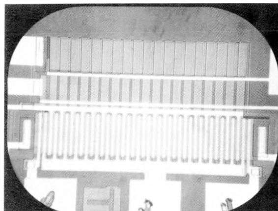
Figure 3. Linear photodiode imaging array coupled to a two phase, overlapping gate CCD.
