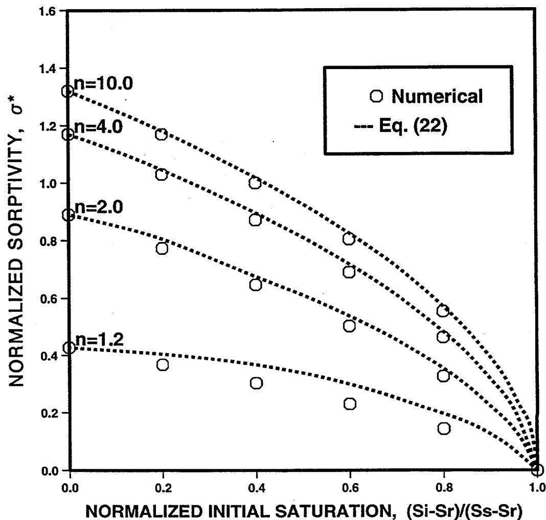
Fig. 4. Normalized sorptivity  $\sigma^* = \sigma[\mu(S_s - S_r)/k\phi|\psi_a|]^{1/2}$  of a van Genuchten medium, as calculated exactly by numerical integration of eq. (5), and from the approximate expression (22).
