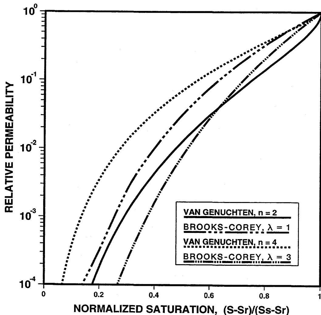
Fig. F2. Relative permeability curves of the van Genuchten and Brooks-Corey type. The choice  $\lambda = n - 1$ , which causes the capillary pressure curves to agree at low saturations, does not cause the relative permeability curves to coalesce.
