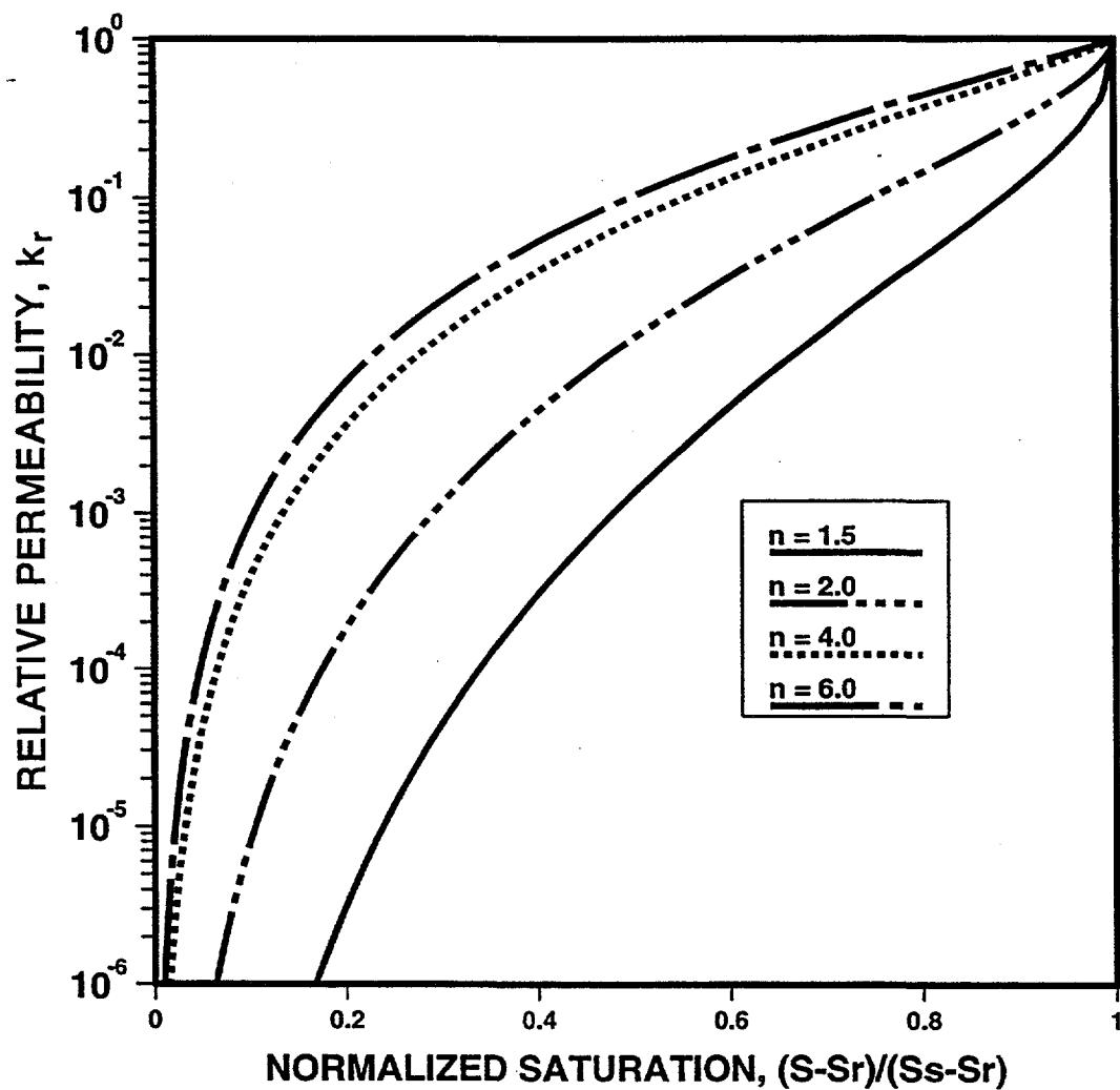
Fig. 2. Relative permeability curves of Mualem - van Genuchten media, as functions of normalized saturation. The parameters  $n$  and  $m$  are related by  $n = 1/(1-m)$ . The equation of the curves, and the definition of normalized saturation, are given in eq. (10), and the adjoining text.
