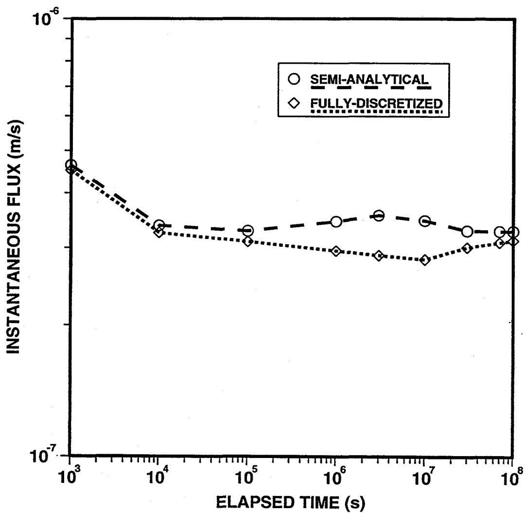
Fig. 7. Instantaneous flux into the fracture, per unit depth perpendicular to the page in Fig. 6, for the horizontal fracture flow problem.
