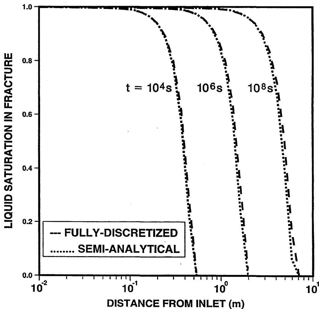
Fig. 8. Saturation profile in the fracture, during flow along a single horizontal fracture, after elapsed times of  $10^4$  s,  $10^6$  s, and  $10^8$  s. Parameters used in the simulations are listed in the text.
