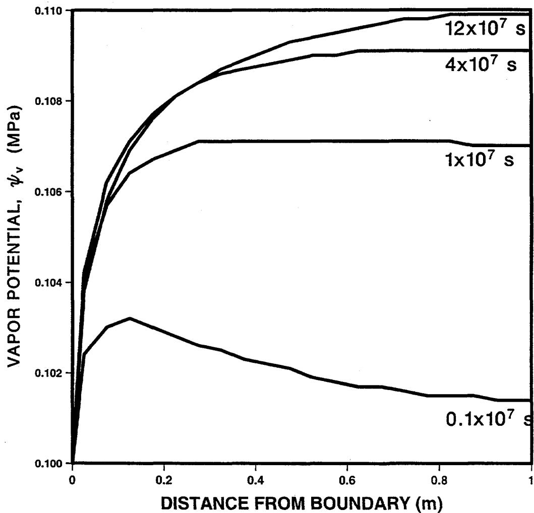
Fig. E2. Pressure profile in the air phase, for same problem as shown in Fig. E1. For the case in which the air is allowed to escape from each gridblock, the air phase pressure is essentially constant at  $1.0 \times 10^5$  Pa. Note that the air phase pressure reaches its maximum value at a point slightly ahead of the location of the wetting front (compare Figs. E1 and E2).
