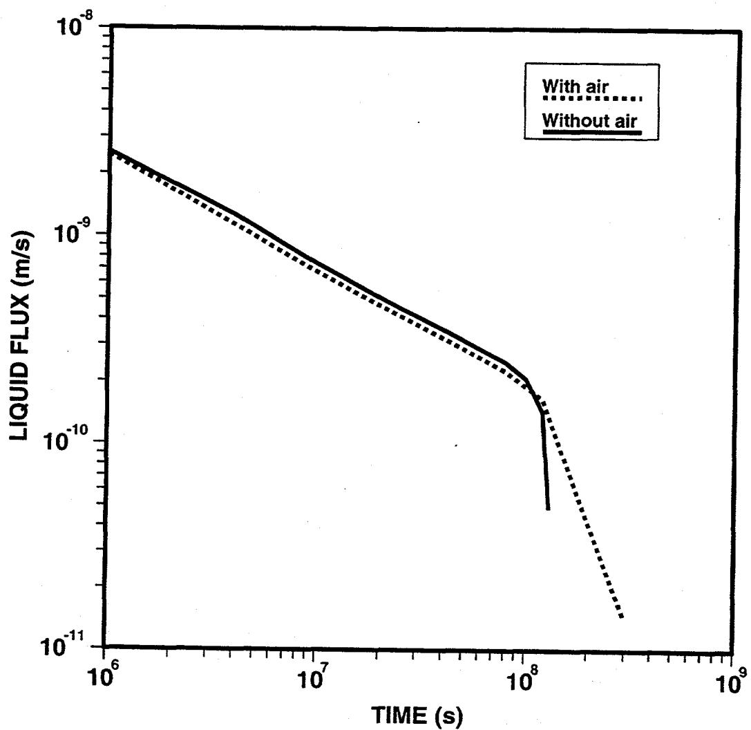
Fig. E3. Imbibition rates of liquid into the slab, for the two cases described in text and Figs. E1 and E2. At early times, the imbibition rate are proportional to  $t^{-1/2}$ , as described in Appendix G. At later times, as the block fills with water, the imbibition rate declines to zero. Except at very large times, the presence of air has a minimal effect on the liquid imbibition rate.
