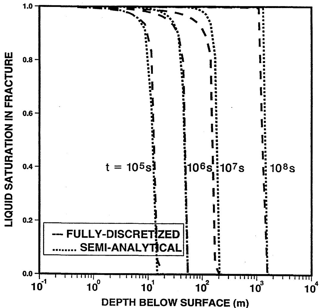
Fig. 10. Saturation profile in the fracture network, during vertical infiltration into a fractured formation, after elapsed times of  $10^5\text{ s}$ ,  $10^6\text{ s}$ ,  $10^7\text{ s}$  and  $10^8\text{ s}$ . Parameters used in the simulations are listed in the text.
