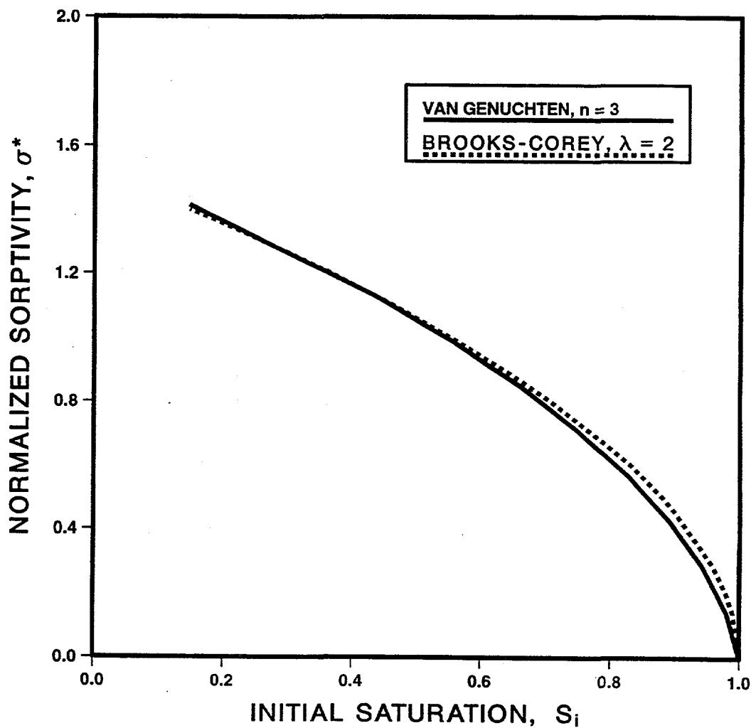
Fig. F3. Normalized sorptivities of van Genuchten and Brooks-Corey media, computed using the Boltzmann transformation method described in Appendix A. Normalized sorptivity is defined by eq. (F9). By choosing  $\lambda = n - 1$ , the sorptivities agree closely, particularly at low-to-moderate values of the initial saturation. At high initial saturations, where the sorptivities are very low, the two curves have different power-law behaviors.
