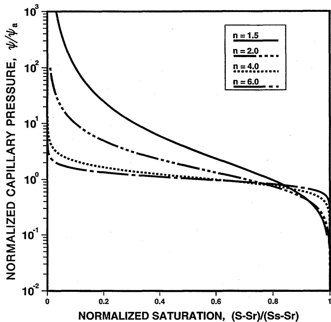
Fig. 1. Normalized capillary pressure curves of Mualem - van Genuchten media, as functions of normalized saturation. The parameters  $n$  and  $m$  are related by  $n = 1/(1-m)$ . The equation of the curves, and the definition of normalized saturation, are given by eq. (9), and the adjoining text.
