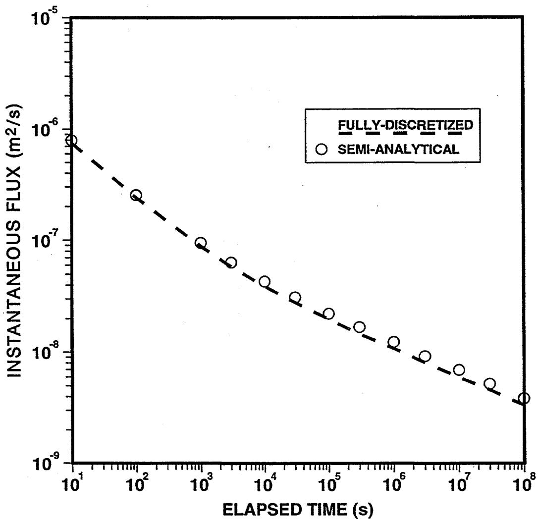
Fig. 11. Instantaneous flux at the surface of the fractured/porous formation, for the vertical infiltration problem.
