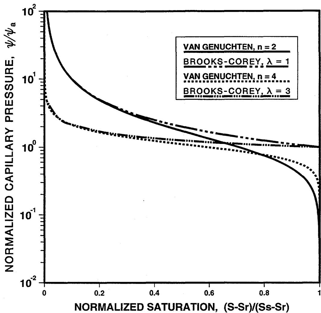
Fig. F1. Normalized capillary pressure curves of the van Genuchten and Brooks-Corey type. The Brooks-Corey curves exhibit an abrupt air-entry pressure at  $\psi = \psi_a$ , whereas the van Genuchten curves are continuous functions of  $\psi$ . If the van Genuchten  $n$  parameter and the Brooks-Corey  $\lambda$  parameter are related by  $\lambda = n - 1$ , the curves will coincide asymptotically at low saturations.
