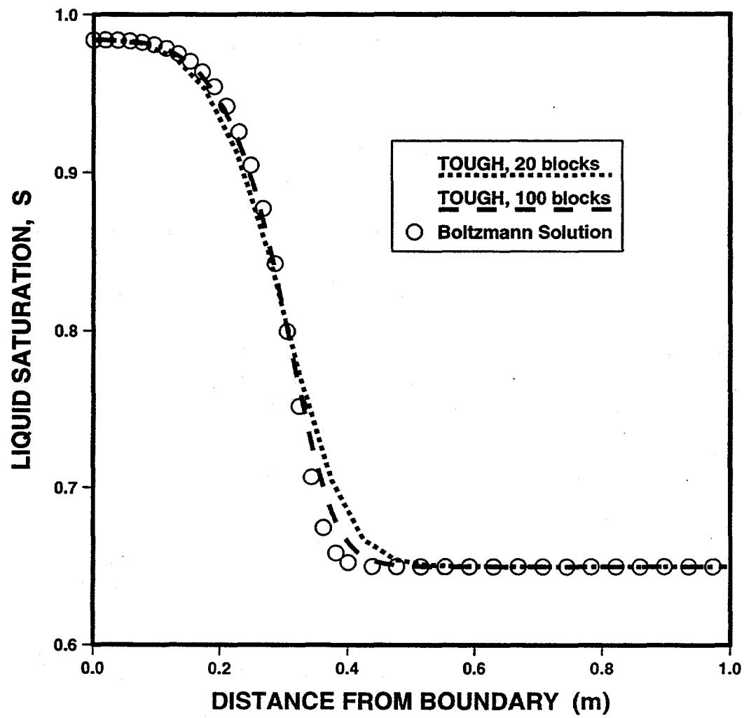
Fig. A4. Saturation profiles computed for one-dimensional absorption of water into a slab of Topopah Spring welded tuff. Properties and parameters are listed in Table A1. The elapsed time is  $10^7$  s.
