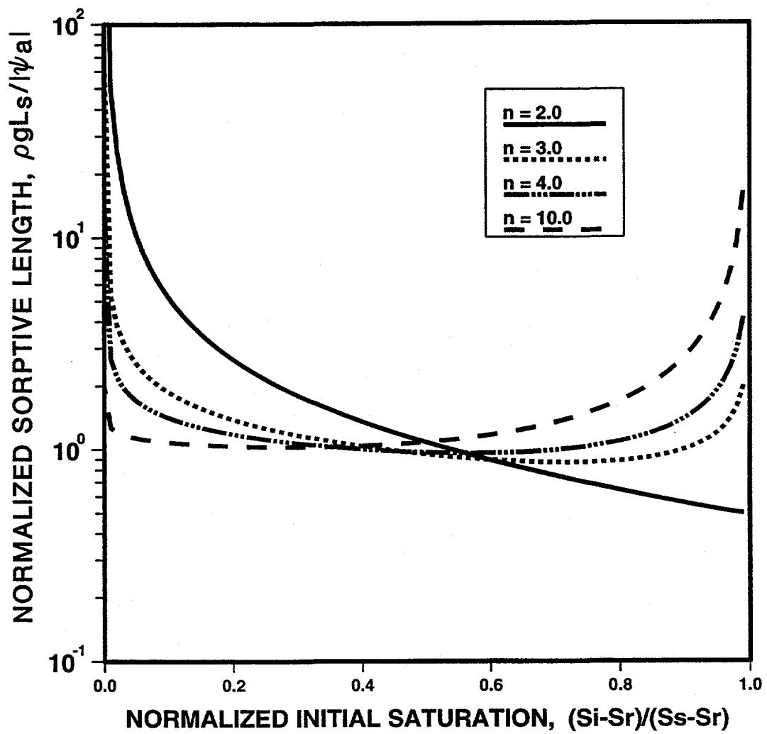
Fig. B1. Sorptive length of a van Genuchten medium, as a function of the initial saturation and the van Genuchten  $n$  parameter, normalized with respect to the approximate value  $|\psi_a|/pg$ . The curves are found from numerical integration of eq. (B6).
