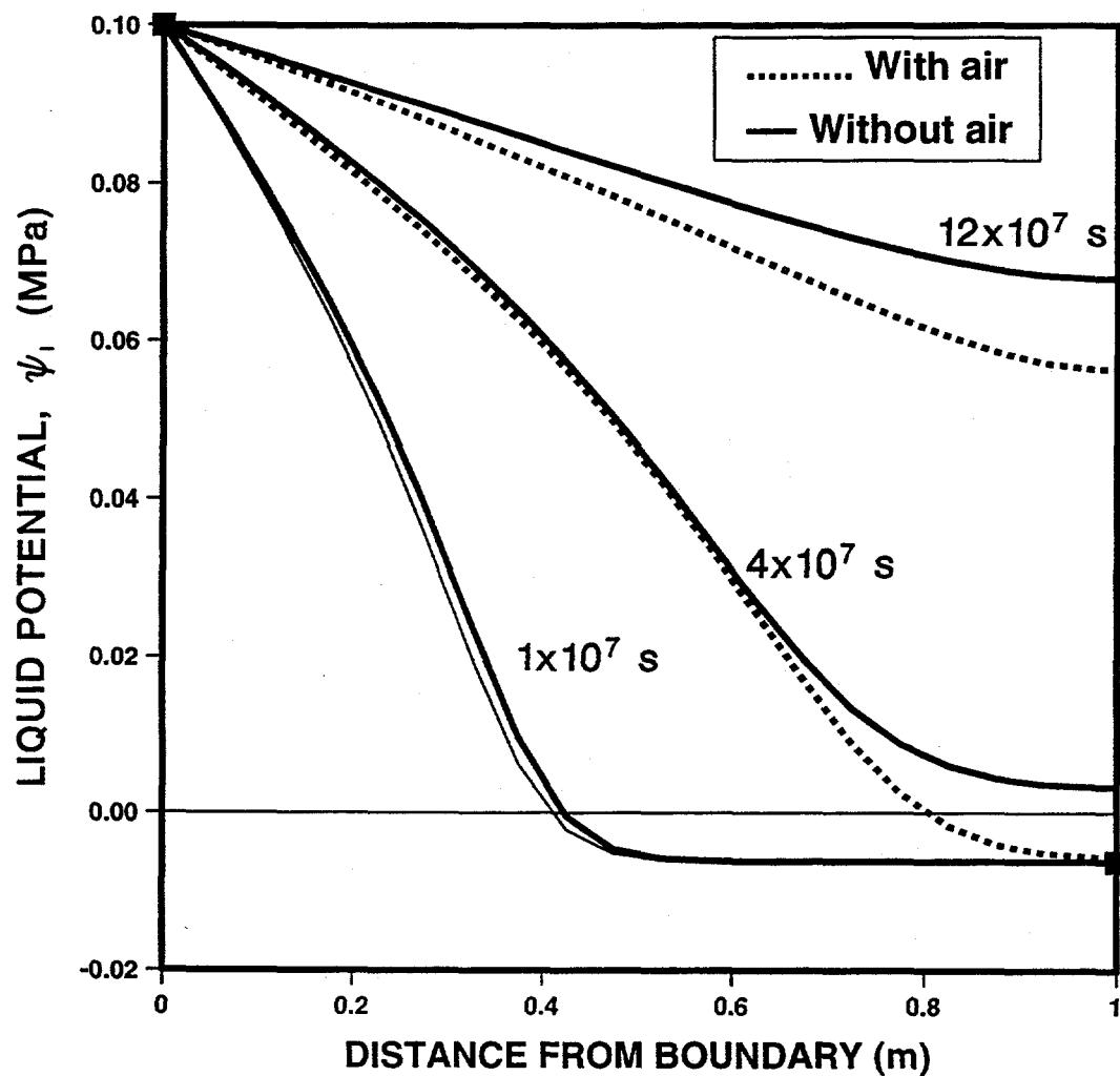
Fig. E1. Pressure profile in the liquid phase, during one-dimensional horizontal imbibition into a slab of Topopah Spring welded tuff. The parameters, initial conditions, etc., are shown in Table A1. There is a no-flow boundary at  $x = 1.0$  m, which models simultaneous imbibition from both faces into a 2.0 m-thick slab. The individual grid-blocks are each of width 5 cm. In one simulation the air-phase pressure is maintained at  $1.0 \times 10^5$  Pa, as described in the text.
