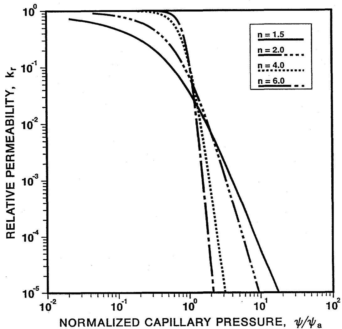
Fig. 3. Relative permeability curves of Mualem - van Genuchten media, as functions of normalized capillary potential. The parameters  $n$  and  $m$  are related by  $n = 1/(1-m)$ . The equation of the curves is given by eq. (8).
