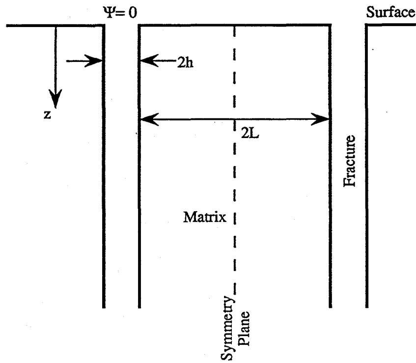
Fig. 9. Schematic diagram of vertical infiltration into a medium containing a set of parallel, equally-spaced fractures of aperture  $2h$  and spacing distance  $2L$ .
