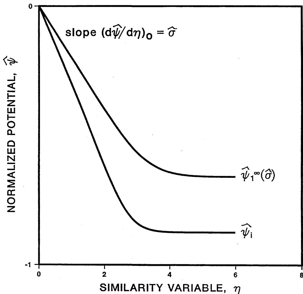
Fig. A1. Schematic diagram of solution procedure for Richards equation. The initial slope  $d\hat{\psi}/d\eta$  at  $\eta=0$  is equal to the normalized sorptivity,  $\hat{\sigma}$ . Different choices of  $\hat{\sigma}$  will lead to different asymptotic values of  $\hat{\psi}^\infty$ . Only one choice of  $\hat{\sigma}$  will lead to the correct asymptotic potential,  $\hat{\psi}^\infty = \hat{\psi}_i$ .
