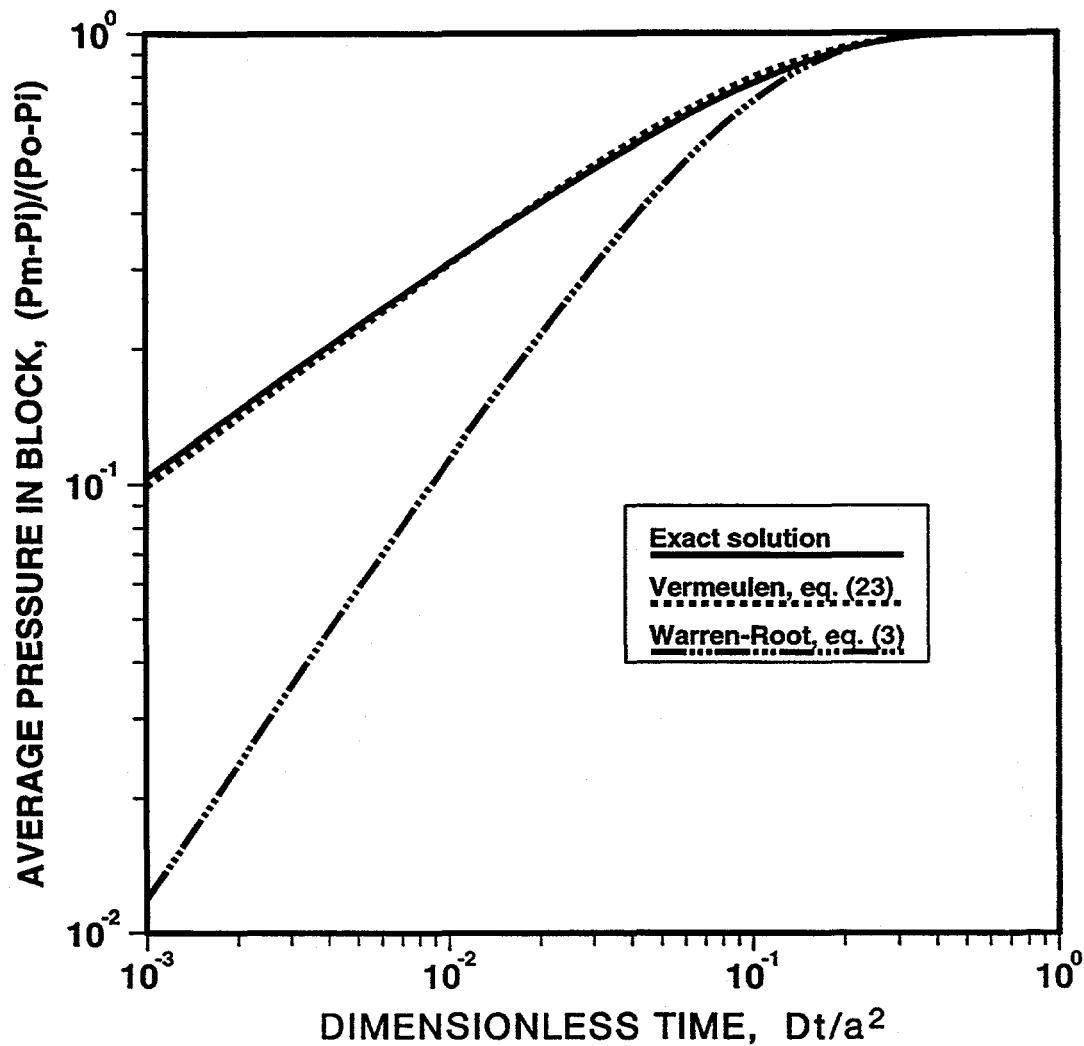
Fig. 5. Normalized mean pressure  $\bar{P}_m$  in a saturated spherical matrix block of radius  $a$  subject to a step-function change in the pressure at its outer boundary from  $P_i$  to  $P_o$ , according to eq. (23), the Warren-Root equation (3), and the exact solution (see Zimmerman et al., 1993). The diffusion coefficient is  $D = k/\phi\mu c$ , and the shape factor for a sphere is  $\alpha = \pi^2/a^2$ .
