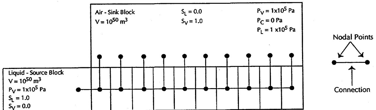
Fig. A2. Schematic diagram of the computational grid used in the TOUGH simulations. The 1 m long slab is broken up into either 20 or 100 equally-sized gridblocks, each with a cross-sectional area of  $1 \text{ m}^3$ . The large boundary gridblock at the left serves as a source of liquid water at  $1 \times 10^5 \text{ Pa}$  pressure, and zero capillary pressure, while the large sink block serves as a sink for air, as described in the text.
