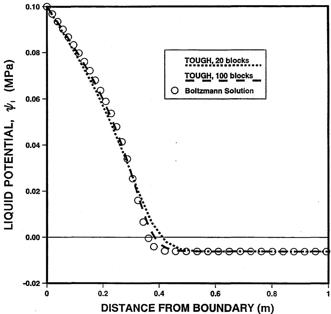
Fig. A3. Potential profiles computed for one-dimensional absorption of water into a slab of Topopah Spring welded tuff. Properties and parameters are listed in Table A1. The elapsed time is  $10^7$  s.
