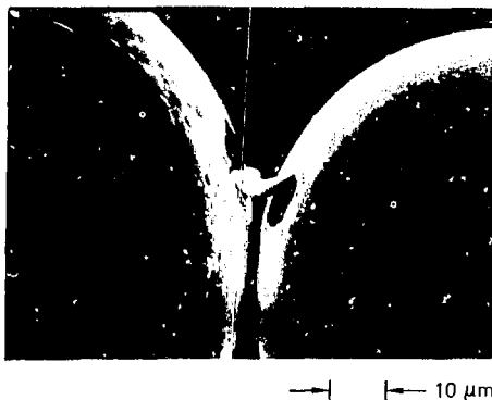
Fig. 4-26. SEM photomicrograph of two gold-coated microspheres showing cold-welding damage spots and torn flap of cold-welded coating.
