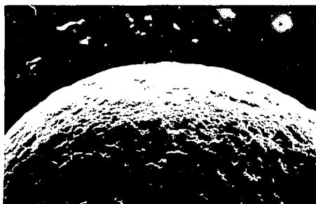
Fig. 4-31. Platinum coated microsphere showing "soft" Class III coating grown with insufficient oxygen doping.
