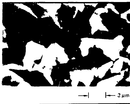
Fig. 4-37. Grain structure in an electroless Au deposit.
