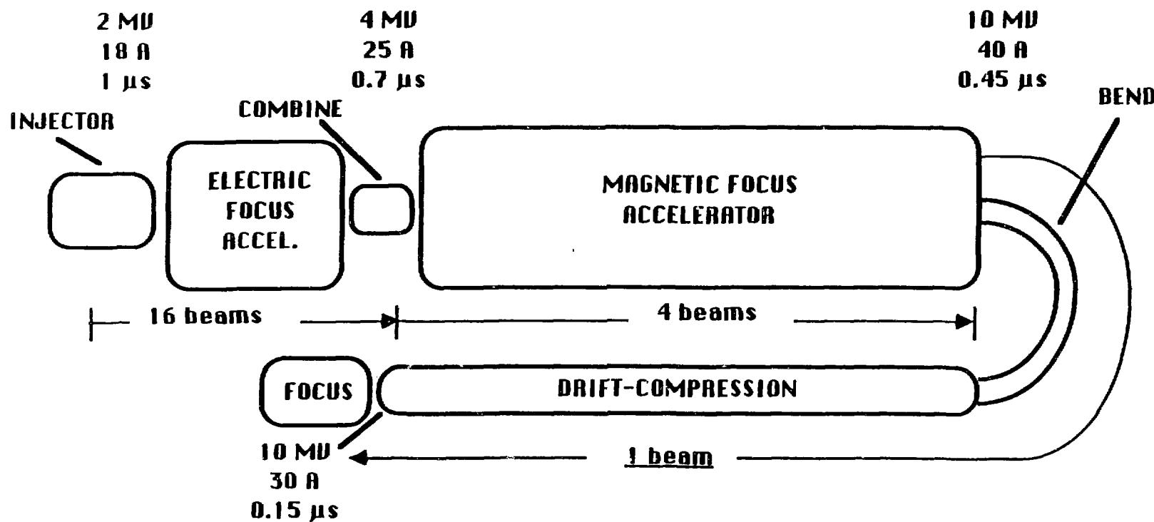
FIG. 1 Schematic of a future Induction Linac Systems Experiment
