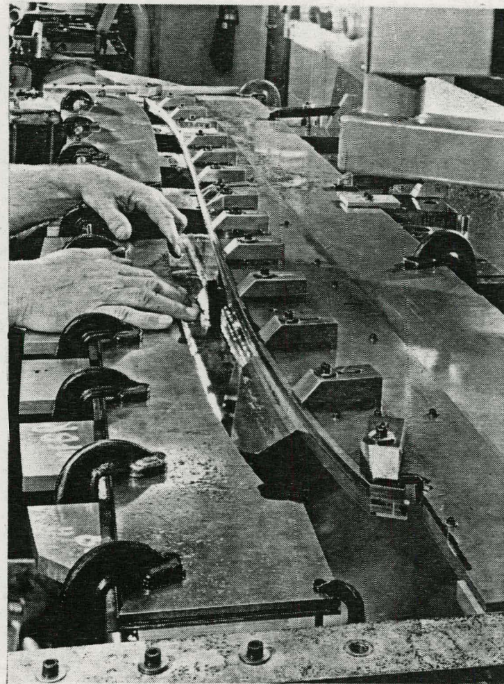
Fig. 12. After completion of stage one and two milling passes on second side, element stock is separated from the rest of the stock.
