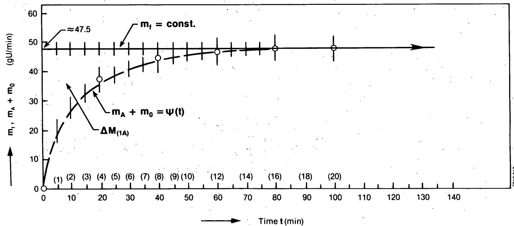
URANIUM MASS RATE VERSUS TIME IN THE 1A COLUMN (RUN HSA-3)
