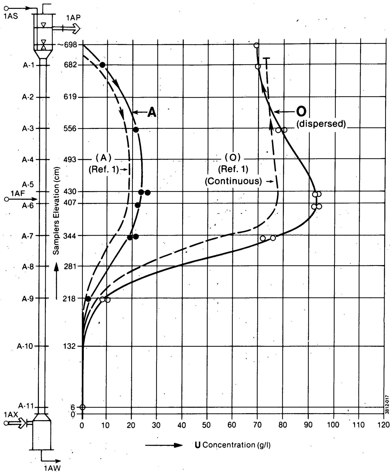
THE 1A (HS) COLUMN EXPERIMENTAL CONCENTRATION PROFILES FOR RUN HSA-1
