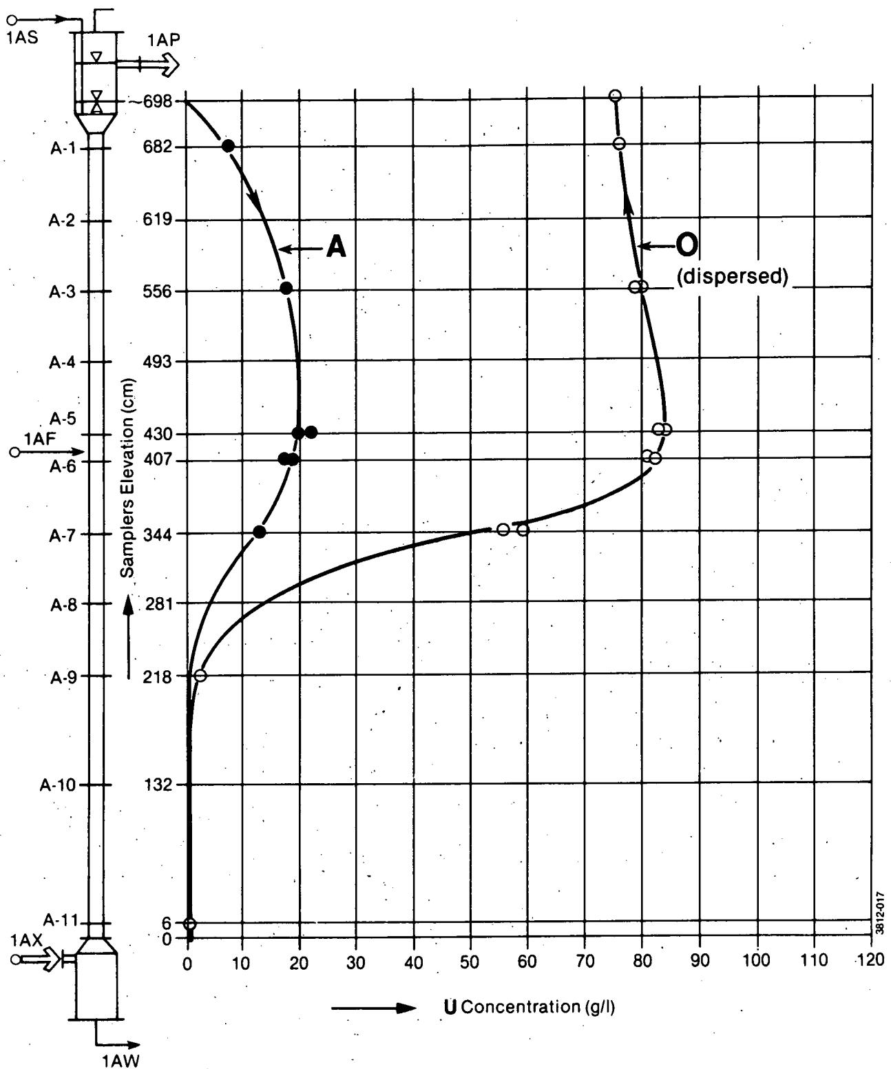
THE 1A (HS) COLUMN EXPERIMENTAL CONCENTRATION PROFILES FOR RUN HSA-3
