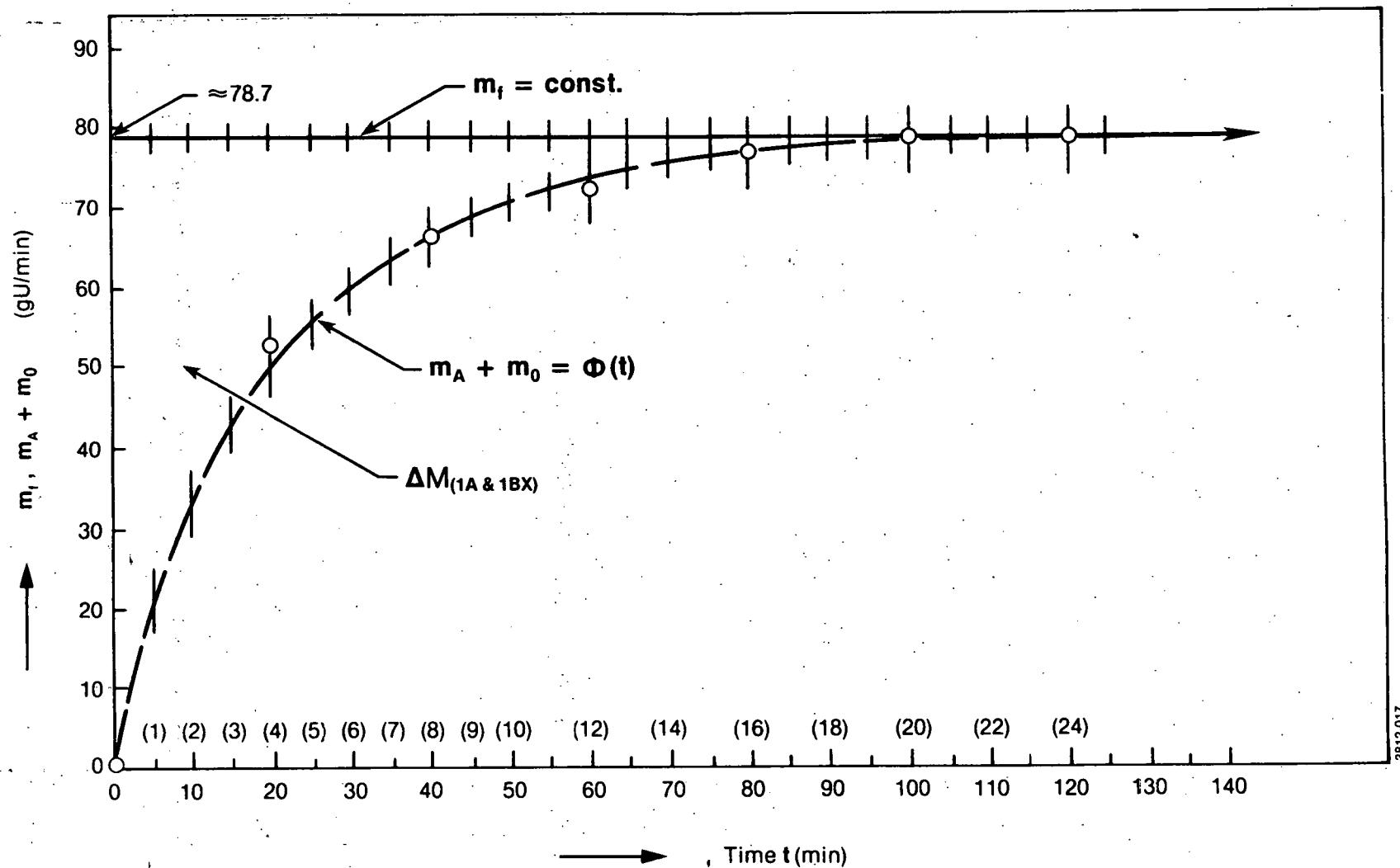
URANIUM MASS RATE VERSUS TIME IN BOTH THE 1A AND 1BX COLUMNS (RUN HSA-1)
