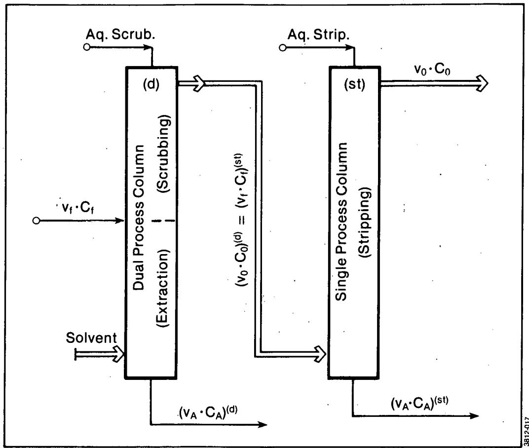
PROCESS CYCLE CONSISTING OF A DUAL AND SINGLE PROCESS COLUMN
