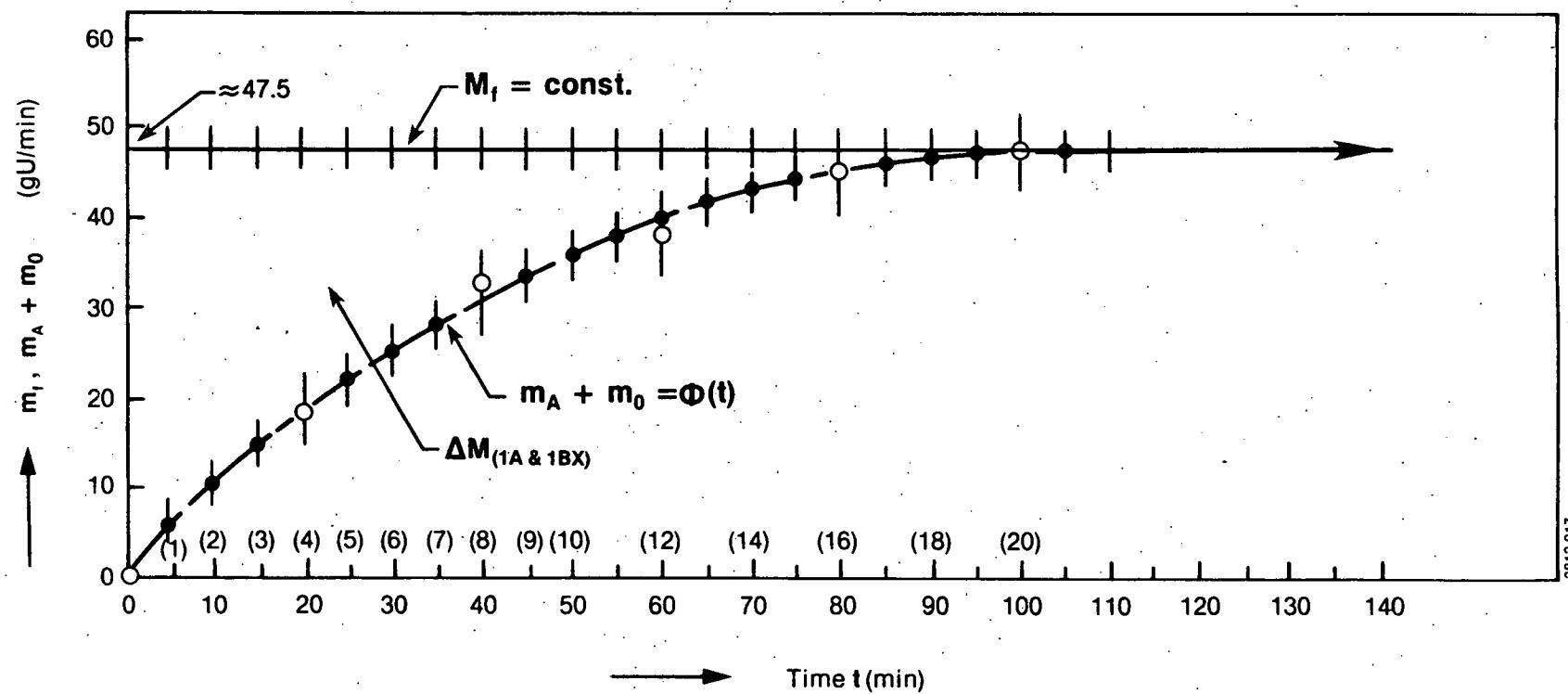
URANIUM MASS RATE VERSUS TIME IN BOTH THE 1A AND 1BX COLUMNS (RUN HSA-3)
