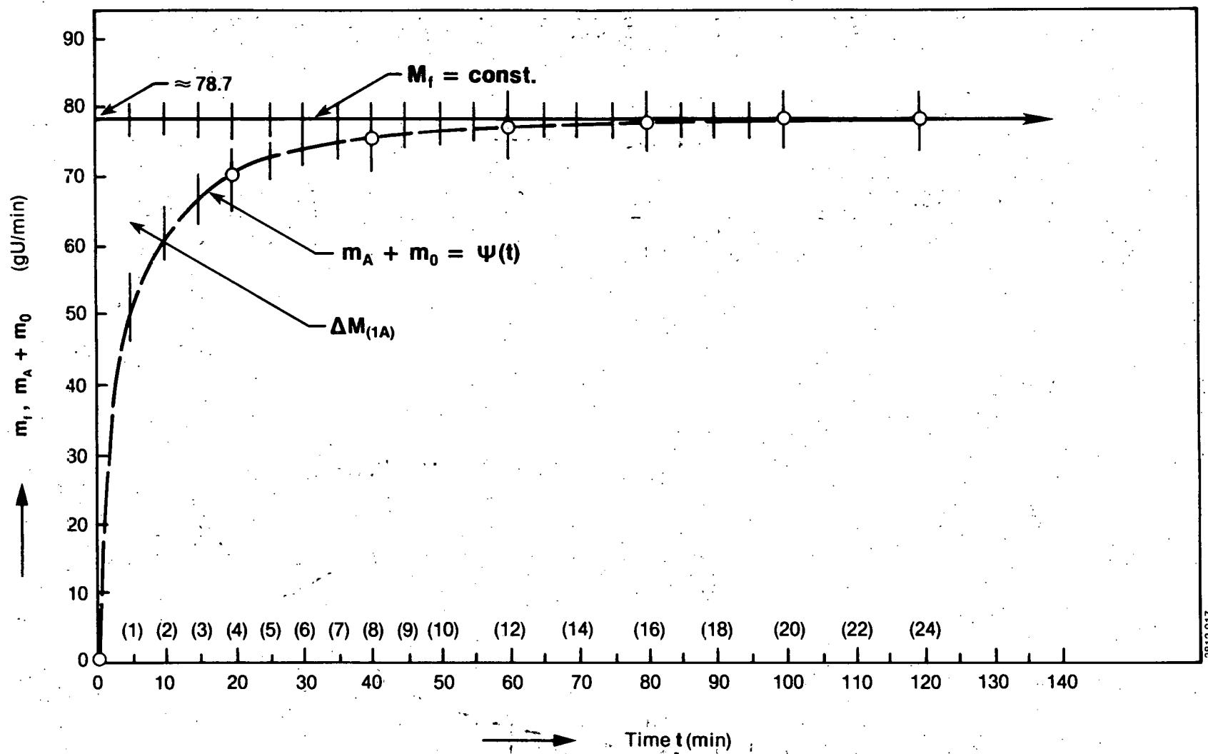
URANIUM MASS RATE VERSUS TIME IN THE 1A COLUMN (RUN HSA-1)
