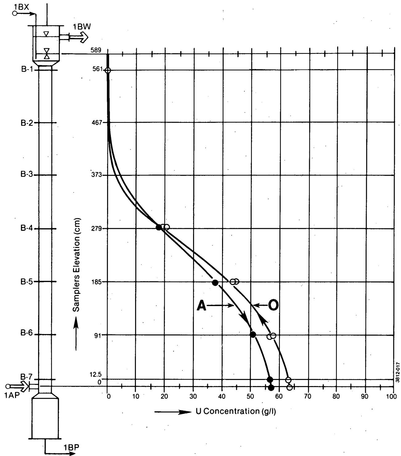
THE 1BX (≡1C) COLUMN EXPERIMENTAL CONCENTRATION PROFILES FOR RUN HSA-2
