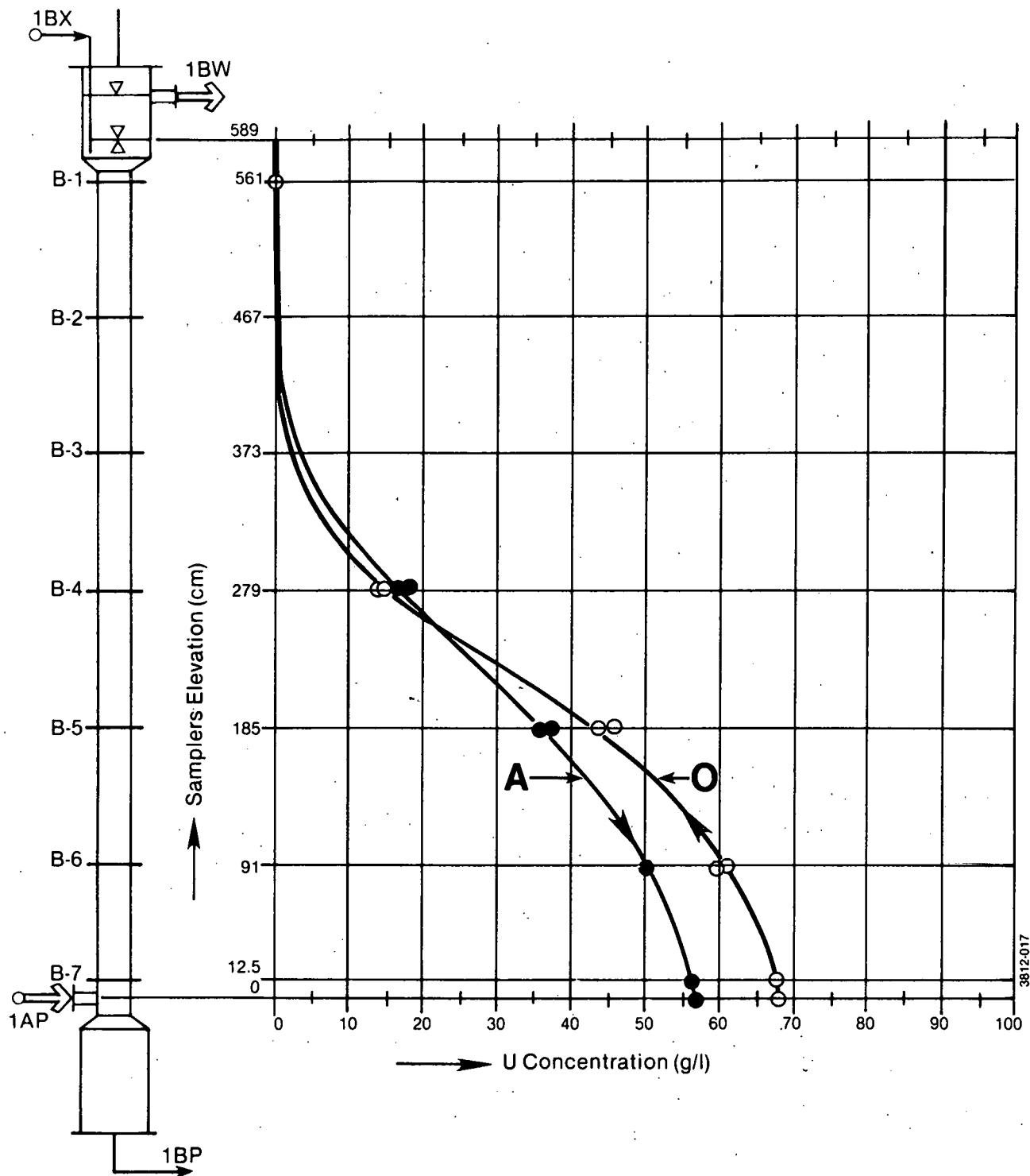
THE 1BX (1C) COLUMN EXPERIMENTAL CONCENTRATION PROFILES FOR RUN HSA-1
