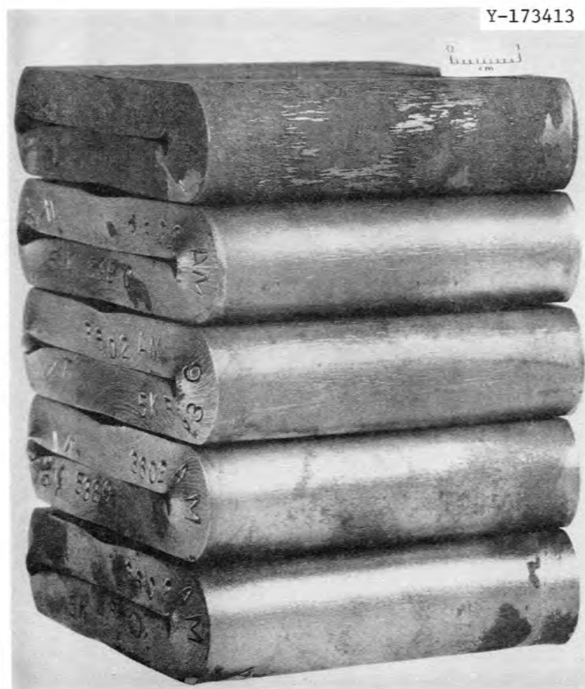
Fig. 5. Response to flattening test of the aged tubes of modified 9 Cr-1 Mo. Normalized and tempered tubes were aged 3000 h at 482, 538, 593, 649, and 704°C (from bottom to top, respectively).
