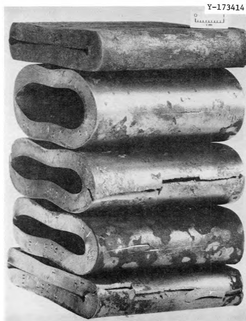
Fig. 6. Response to flattening test of the aged tubes of HT9. Normalized and tempered tubes were aged 3000 h at 482, 538, 593, 649, and 704°C (from bottom to top, respectively).
