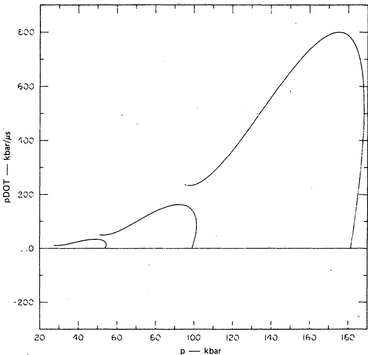
80/12/01. SIMILARITY SOLUTION.  $N=2.75$ ,  $V_1/V_0=.862$
