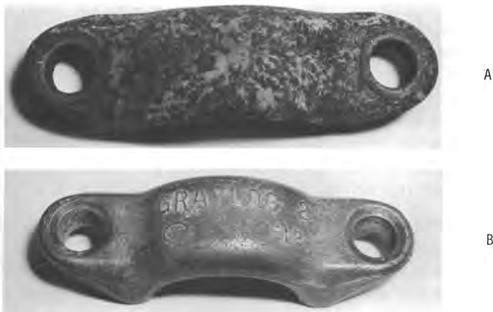
FIGURE 16. Mild Steel Pipe Clamps (A) As-Received and (B) After Removal of Rust and Gross Contamination by 4 h of Vibratory Finishing
