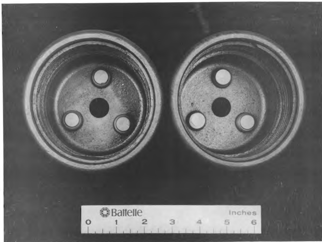
FIGURE 3. Reactor-Process Tube End-Caps After Decontamination by Liquid Honing
