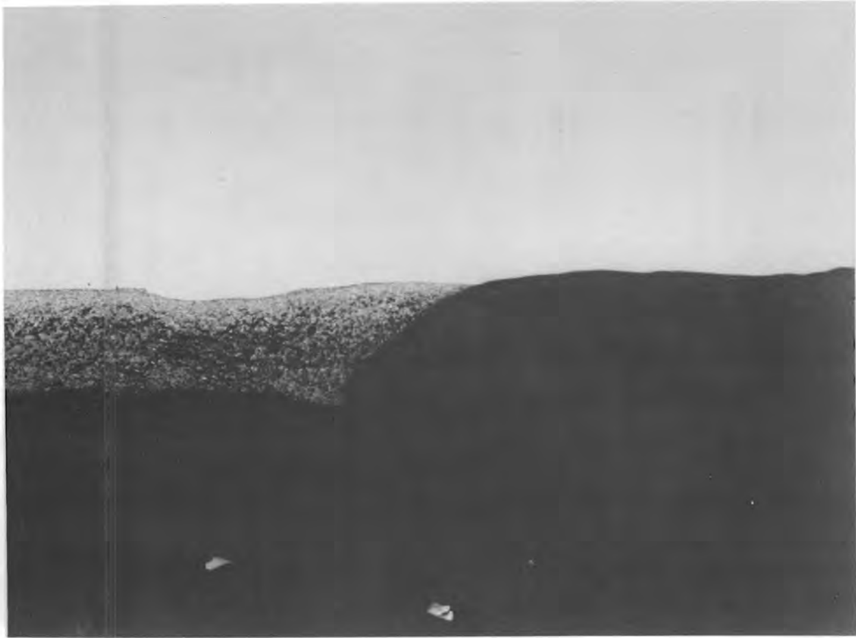
FIGURE 9. Optical Micrograph of Oxidized 304L Stainless Steel Descaled by Electropolishing With Electrolyte #1
