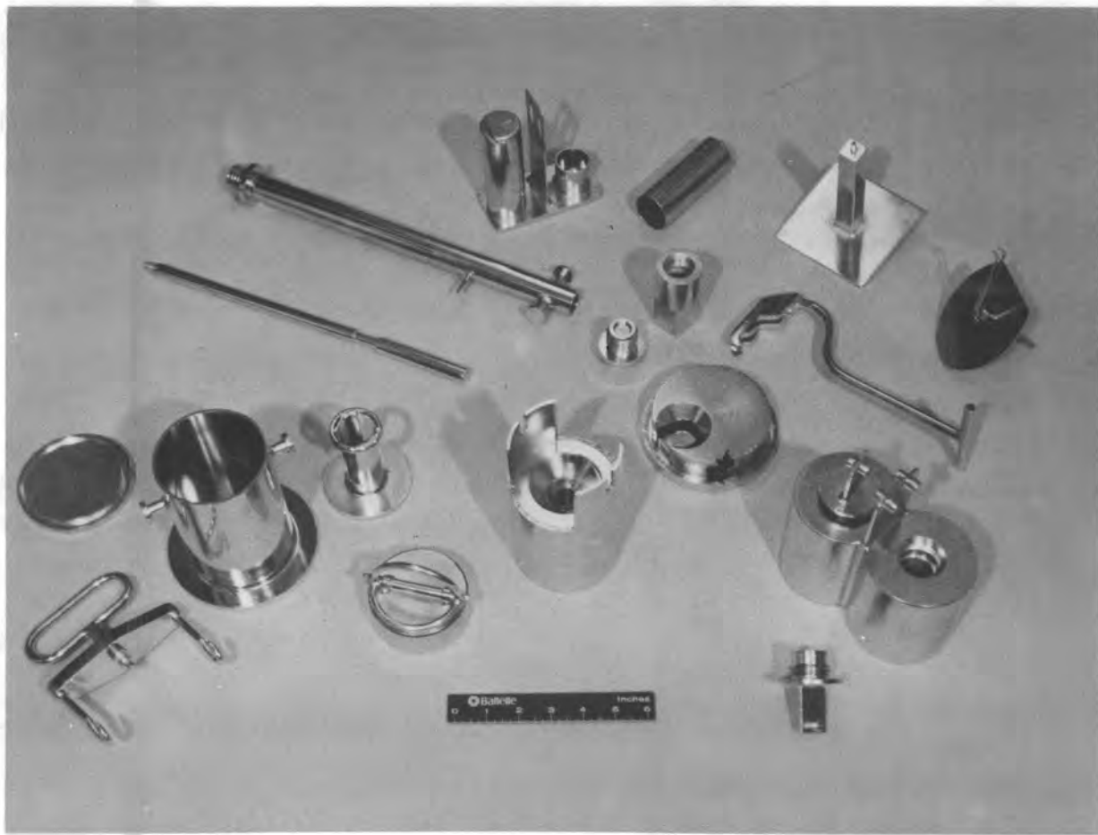
FIGURE 6. Stainless Steel Laboratory Ware Decontaminated by Electropolishing. The highly polished surface facilitated subsequent decontamination using standard swab techniques.
