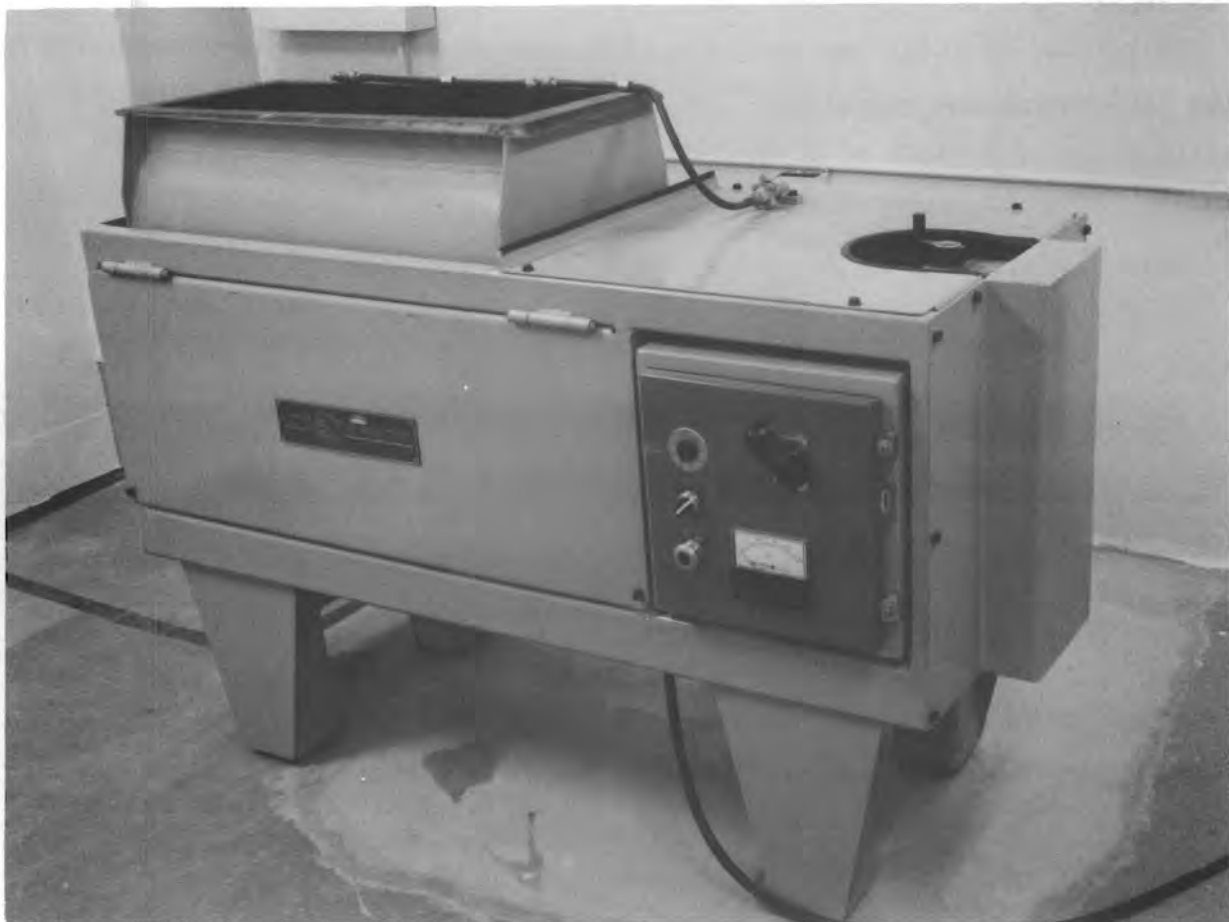
FIGURE 15. Vibratory Finisher With 4-ft 3 Tub Capacity Used in Pretreatment Studies
