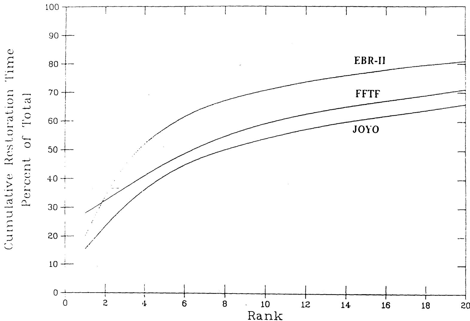
Figure 1. Cumulative restoration time as a function of maintenance critical item rank.
