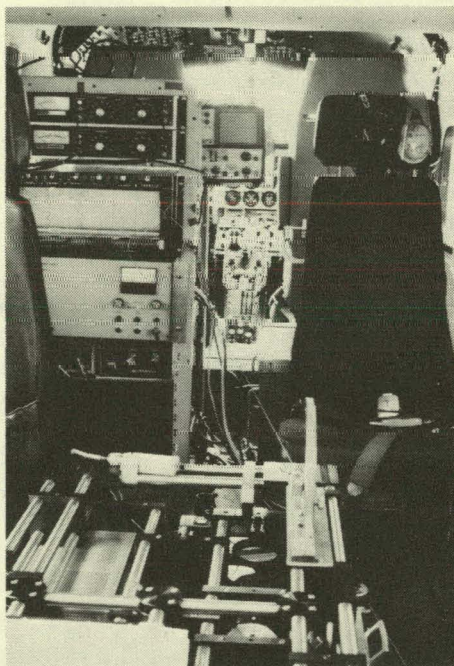
Fig. 3. Differential absorption laser spectrometer installed on DFVLR/Dornier Sky servant
