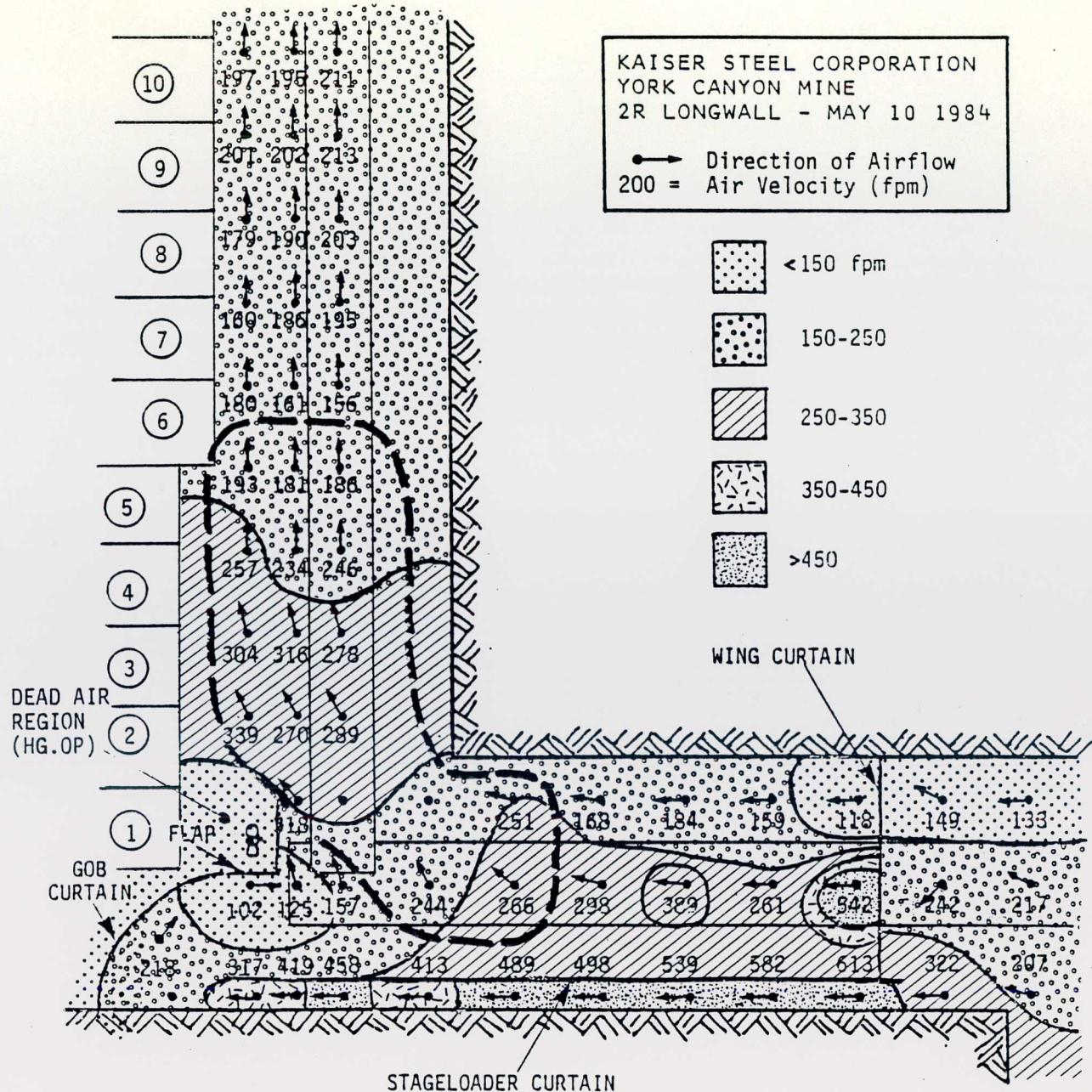
FIGURE 28. - Smoke trace and air velocity survey - wing and gob curtains in place.
