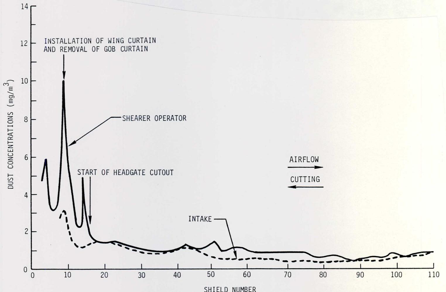
FIGURE 25. - Dust concentration versus shield number; tail-to-head cutting - Kaiser Steel Corporation, York Canyon Mine.
