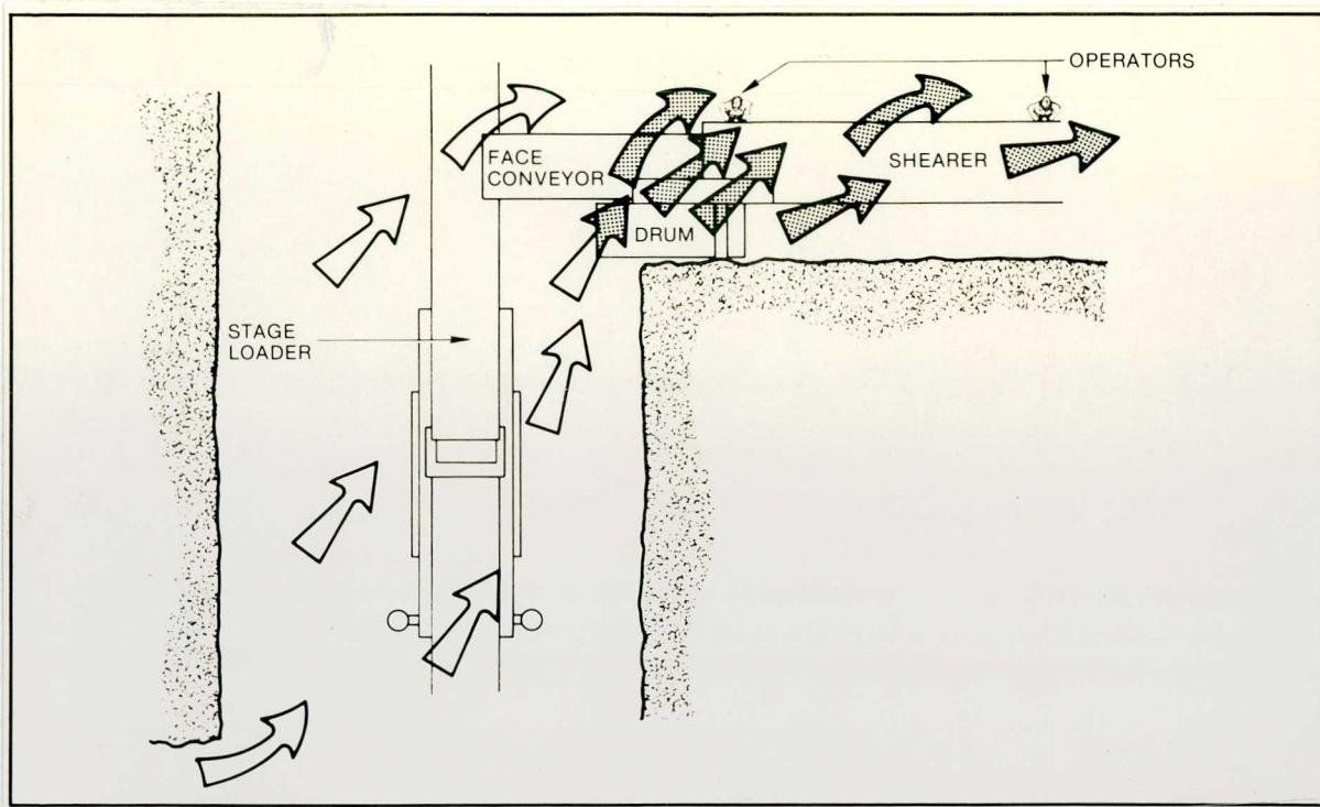
FIGURE 1. - Primary ventilation blows dust from shearer drum over the operators.
