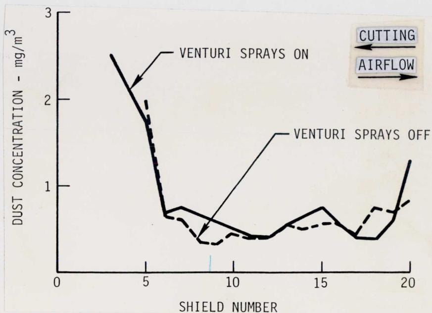
FIGURE 22. - Dust concentrations at headgate shearer operator's position during headgate cutout, tail-to-head cutting - Price River Coal Company.
