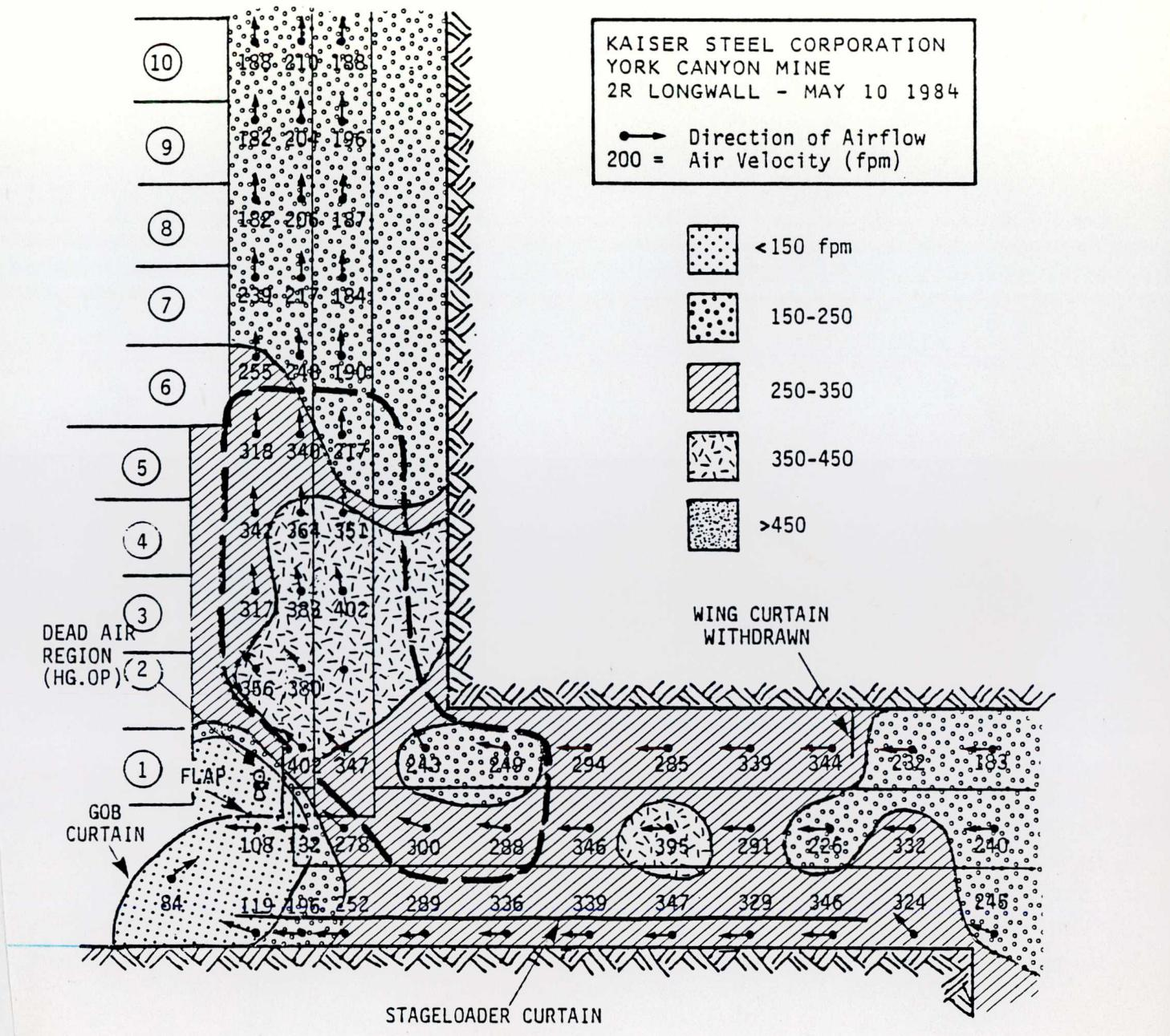
FIGURE 27. - Smoke trace and air velocity survey - wing curtain withdrawn, gob curtain in place.
