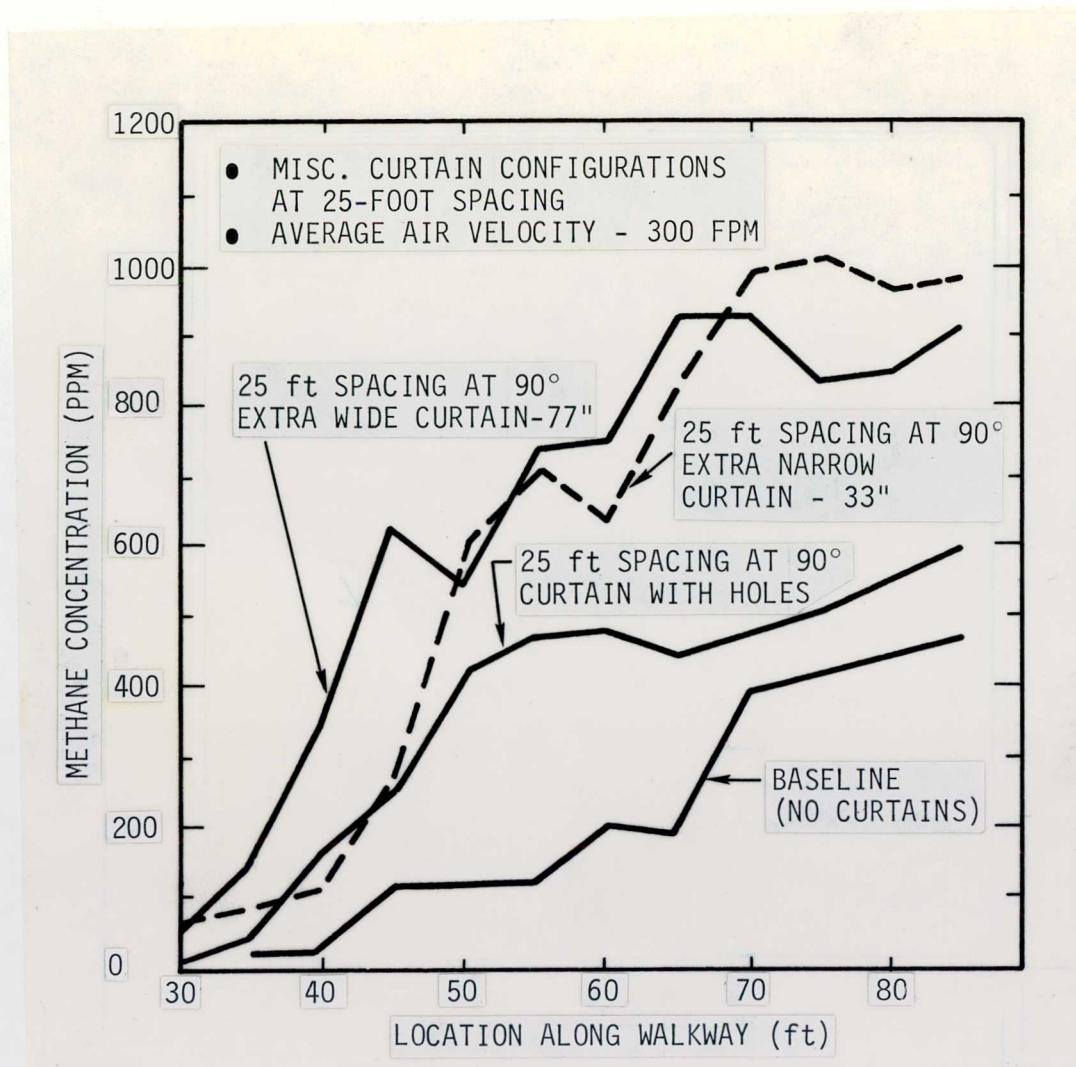
FIGURE 9. - Methane gas concentrations of different curtain configurations along walkway.
