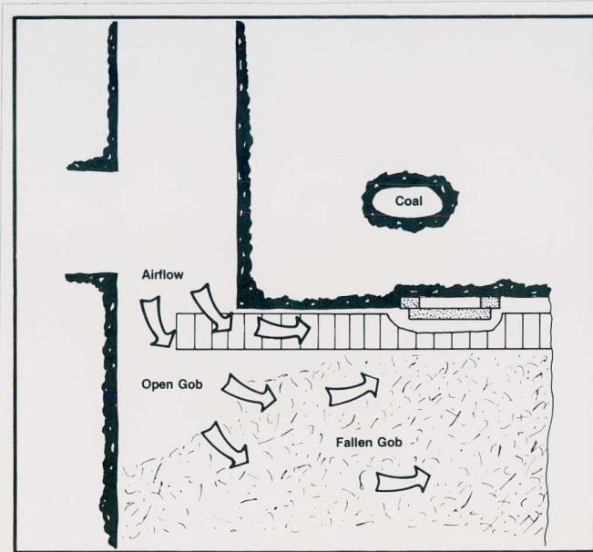
FIGURE 3. - A portion of the ventilation air from the headgate entry leaks into the gob, lowering the airflow along the longwall face.
