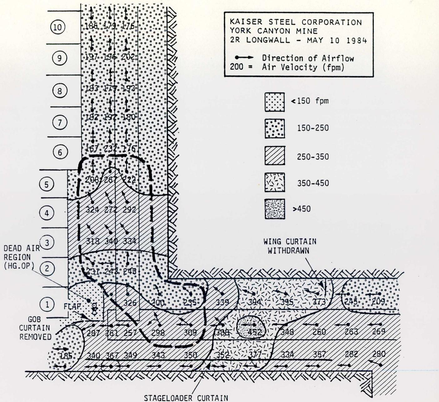
FIGURE 26. - Smoke trace and air velocity survey - wing curtain withdrawn, gob curtain removed.
