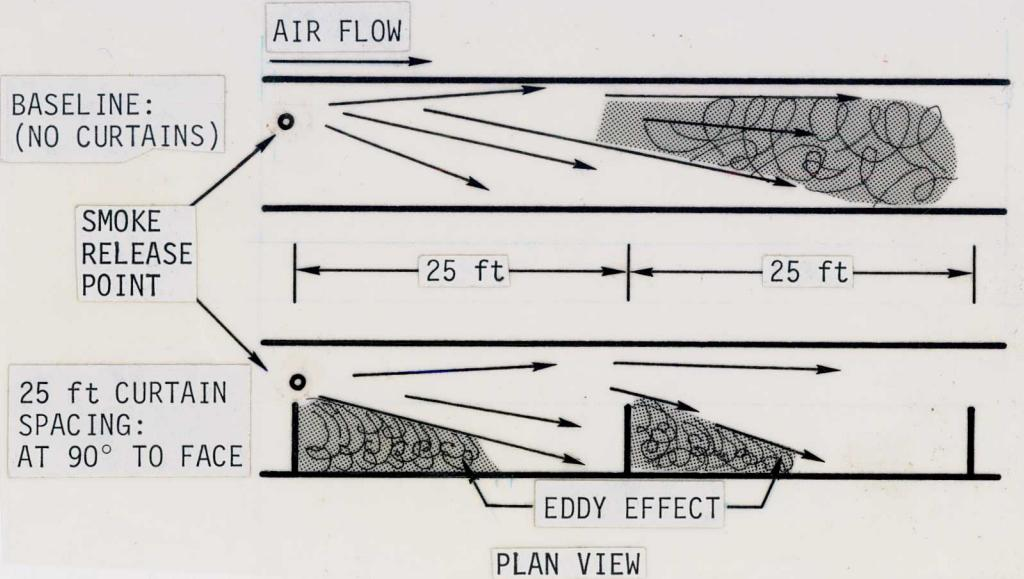
FIGURE 7. - Ventilation map comparing airflows - baseline conditions versus 25-ft curtain spacing.
