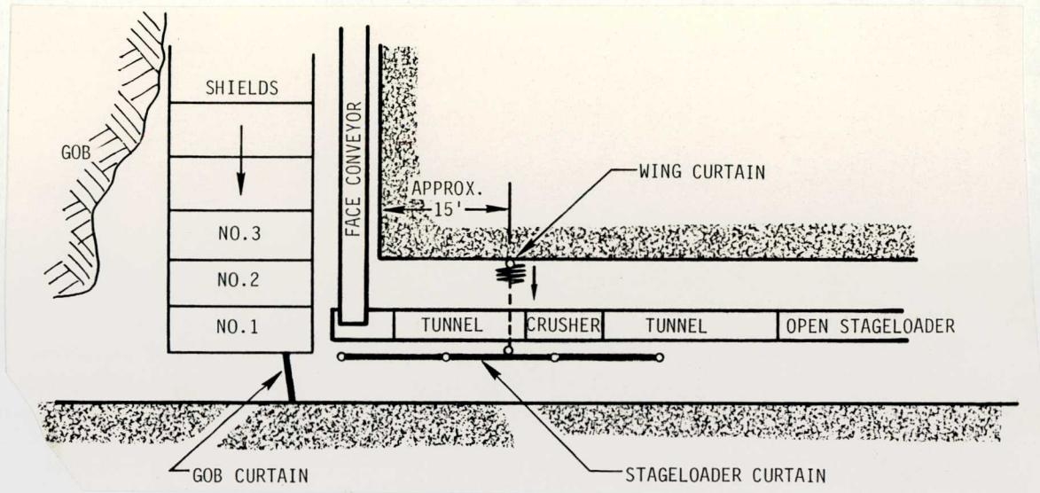
FIGURE 24. - Kaiser's use of a unique wing curtain - gob curtain - stageloader curtain system for headgate cutout dust control.
