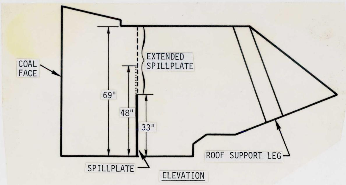
FIGURE 10. - Extended spillplate.
