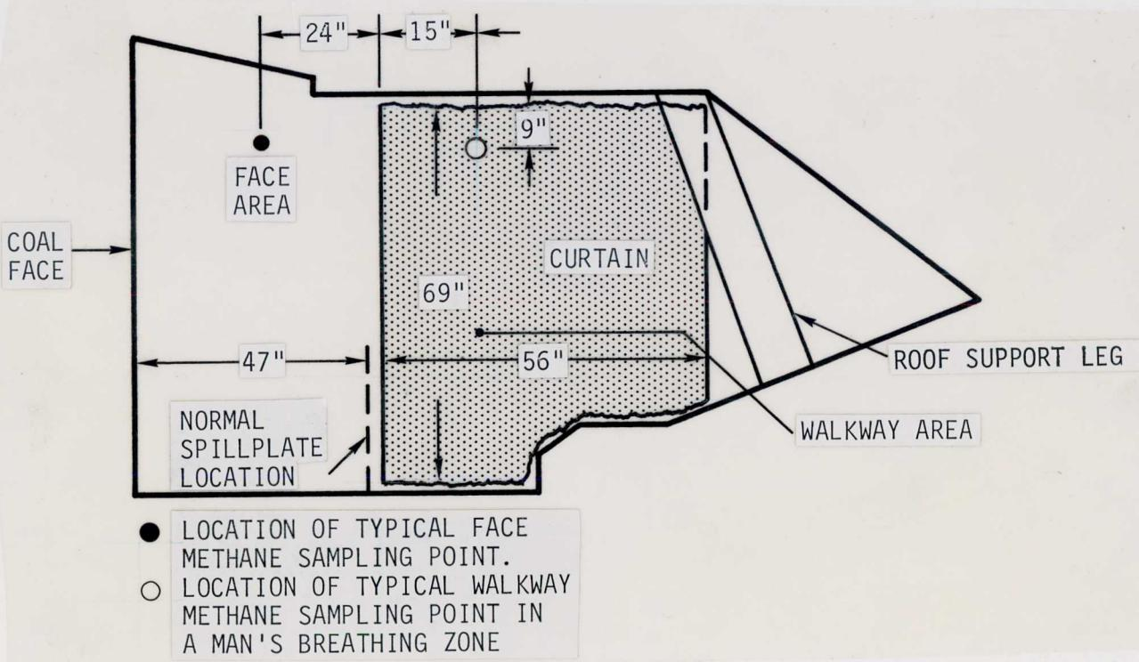
FIGURE 5. - Walkway curtain installation - section view of longwall gallery.
