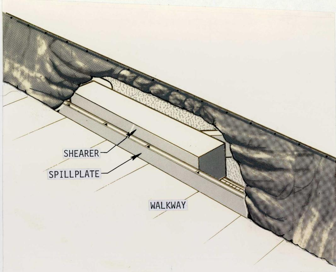
FIGURE 11. - Sketch of "full height" extended spillplate installed in longwall gallery.
