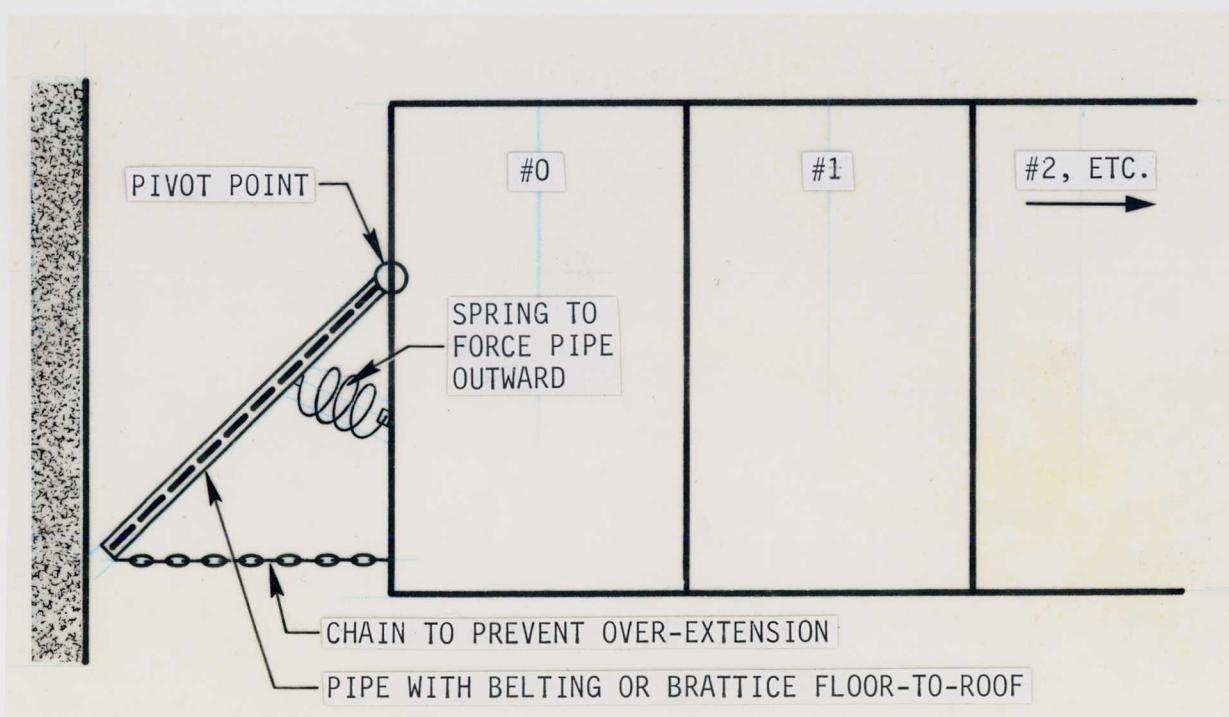
FIGURE 21. - Permanent gob curtain design advancing with first shield support.
