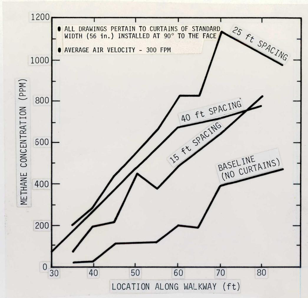
FIGURE 8. - Methane gas concentrations of 90-deg curtain configurations along walkway.
