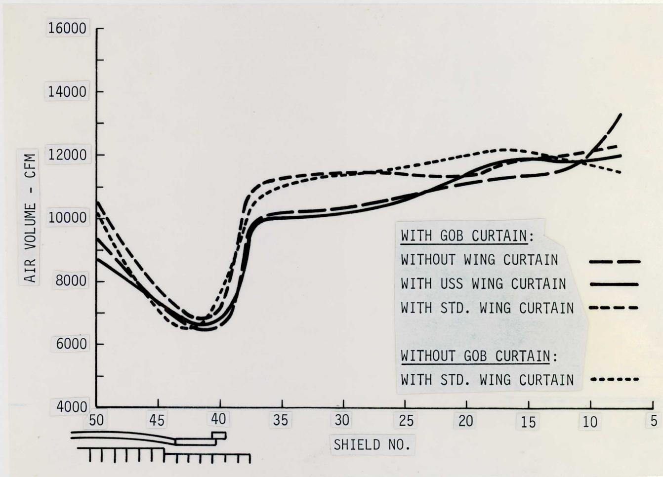
FIGURE 18. - Air volume readings along face.
