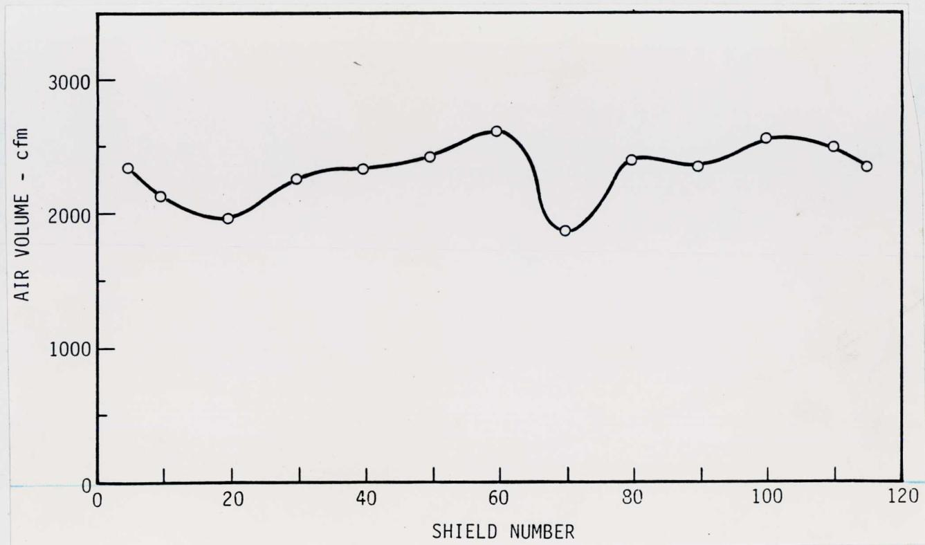
FIGURE 30. - Air volume survey along face - gob curtain in use, wing curtain retracted.
