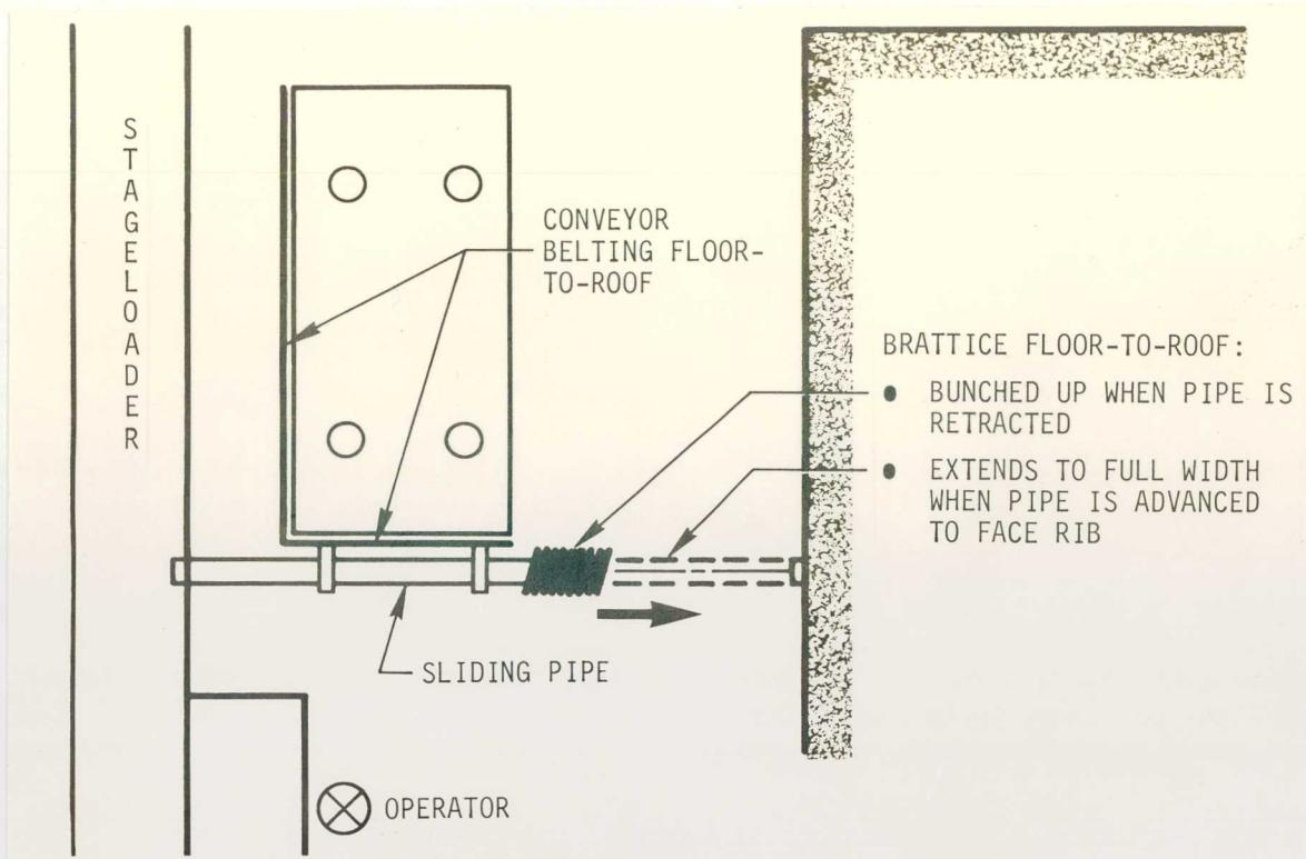
FIGURE 20. - Permanent wing curtain design advancing with buttress chock.
