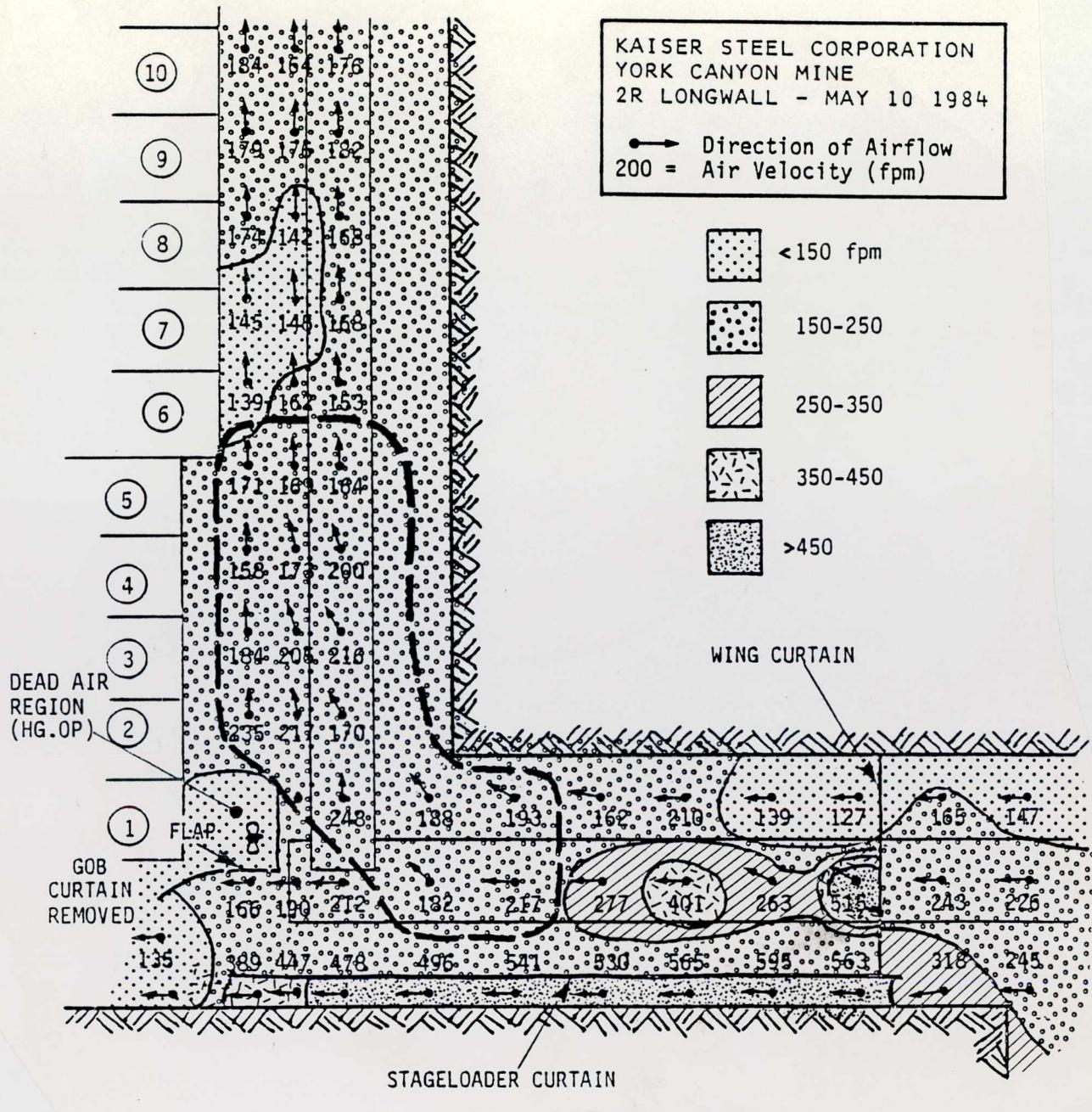
FIGURE 29. - Smoke trace and air velocity survey - wing curtain in place, gob curtain removed.
