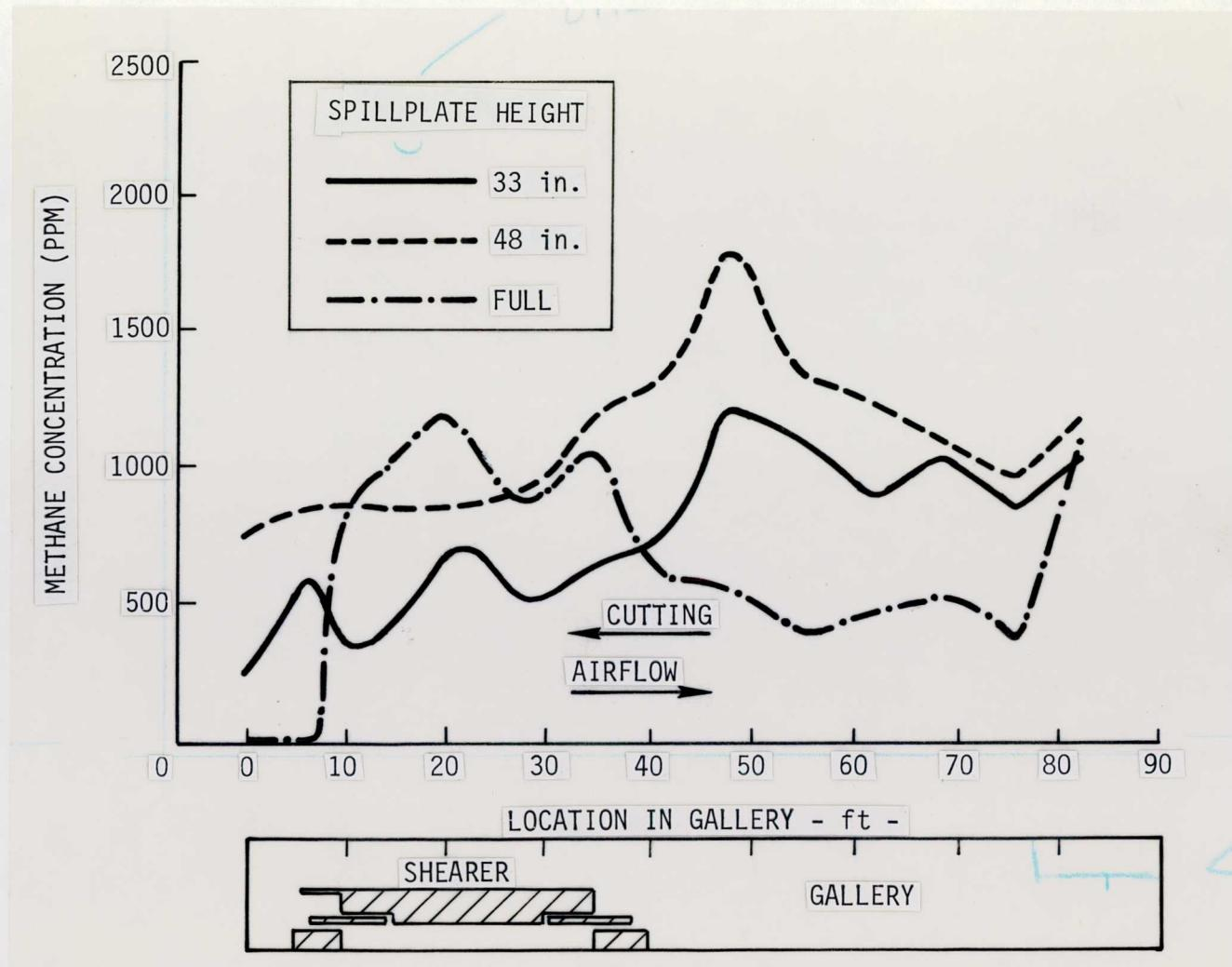
FIGURE 12. - Contamination profiles around shearer with extended spillplates.
