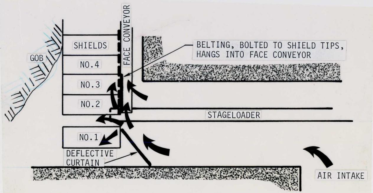
FIGURE 23. - ARMCO's use of brattice and belting to control headgate airflow patterns.
