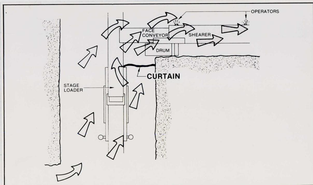
FIGURE 2. - Curtain shields shearer drum from primary ventilation.
