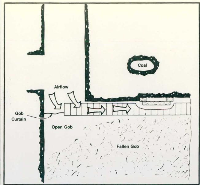
FIGURE 4. - Gob curtain closes gap between shield No. 1 and the adjacent rib, forcing more air along the longwall face.
