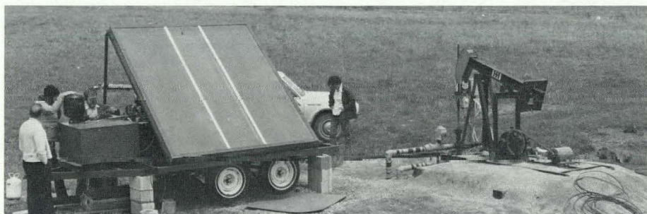
Trailer-mounted preheater includes two heat exchangers, solar panels, a tank, and a heat pump.
