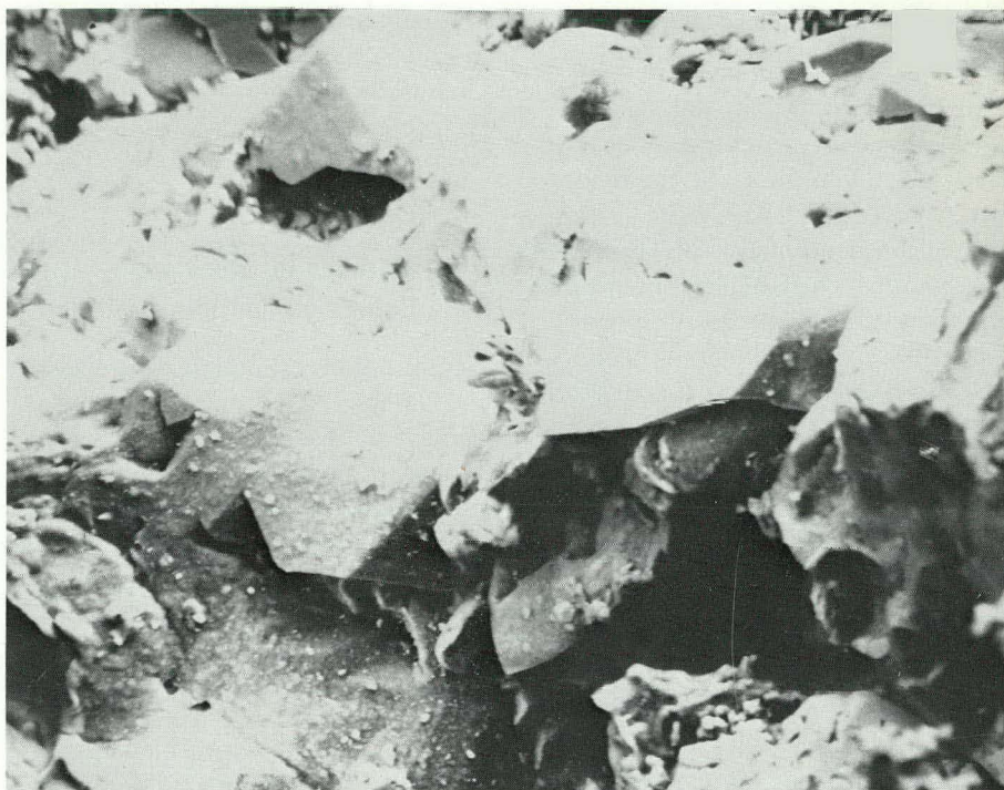
FIGURE B1. Scanning electron micrograph of Berea sandstone. Note pores and clay minerals on and between sand grains.
