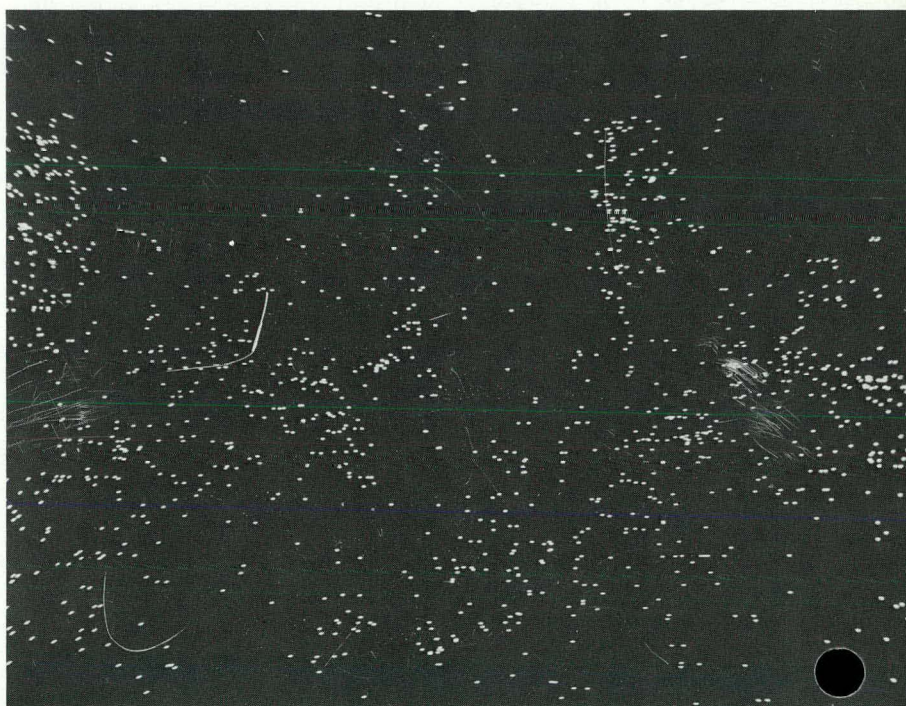
FIGURE B2. X-ray scan of aluminum on the surface of Berea sandstone shown in figure B1.
