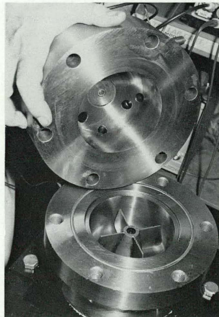
This closeup shows details of the fuel combustion assessment rig being used in the first step of the coal slurry fuel screening process.
