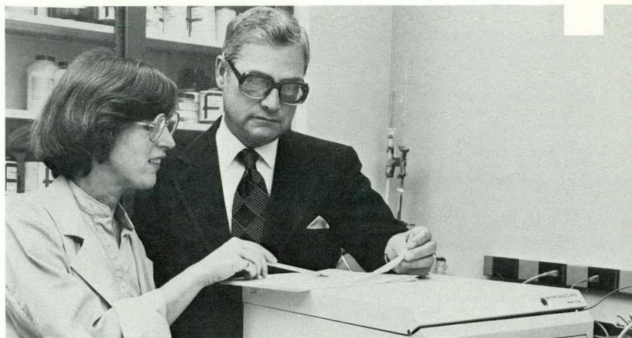
Edward J. Lievens, Jr., new acting director of BETC, familiarizes himself with BETC laboratory work by reviewing results of molecular weight determinations with Bonnie Gall, research chemist. These determinations for a high-residue-guar fracturing fluid gel were made by size occlusion chromatographic equipment (foreground) as part of the Western Gas Sands Project studies. Fracturing fluid gels are being examined to determine (1) how much damage they cause to sandstone formations and hydraulic fractures, and (2) how easily they can be removed from a fracture once the fracture has been propped open.
