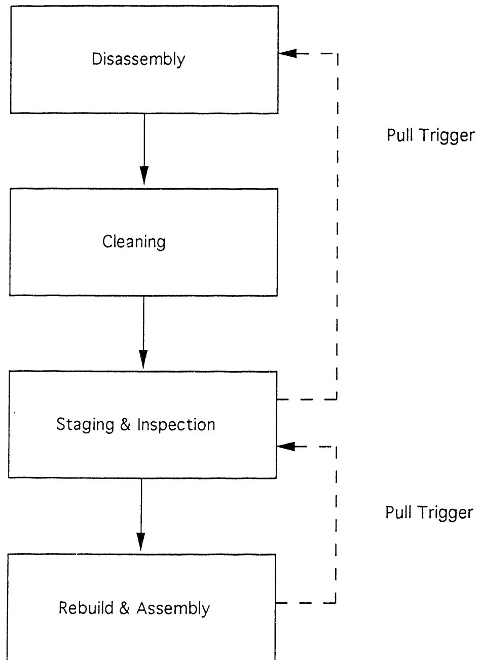
Figure 1. Material Flow and Pull Linkages
