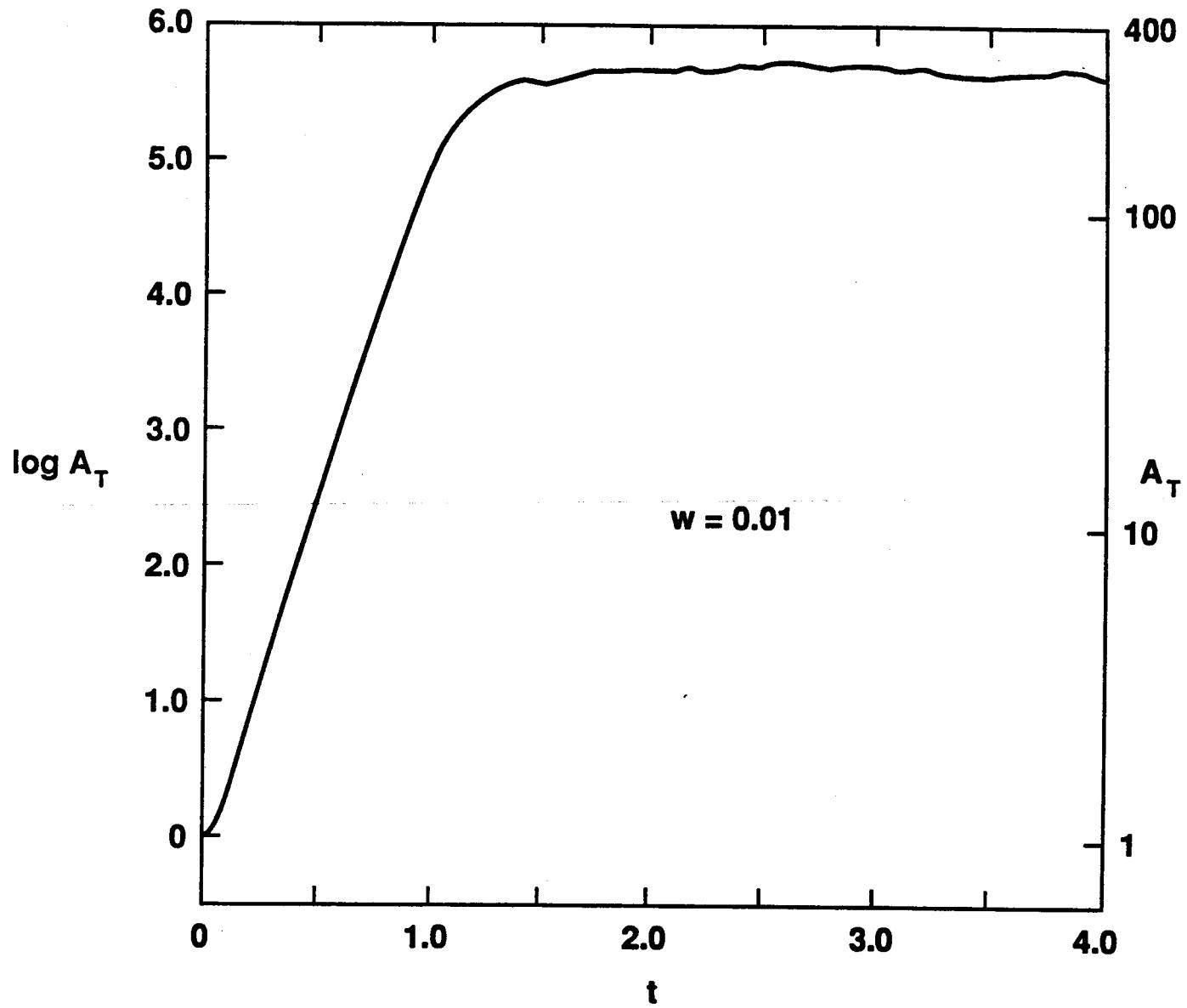
Figure 2: Natural Logarithm of Flame Sheet Area (Per Initial Area) Against Time.
