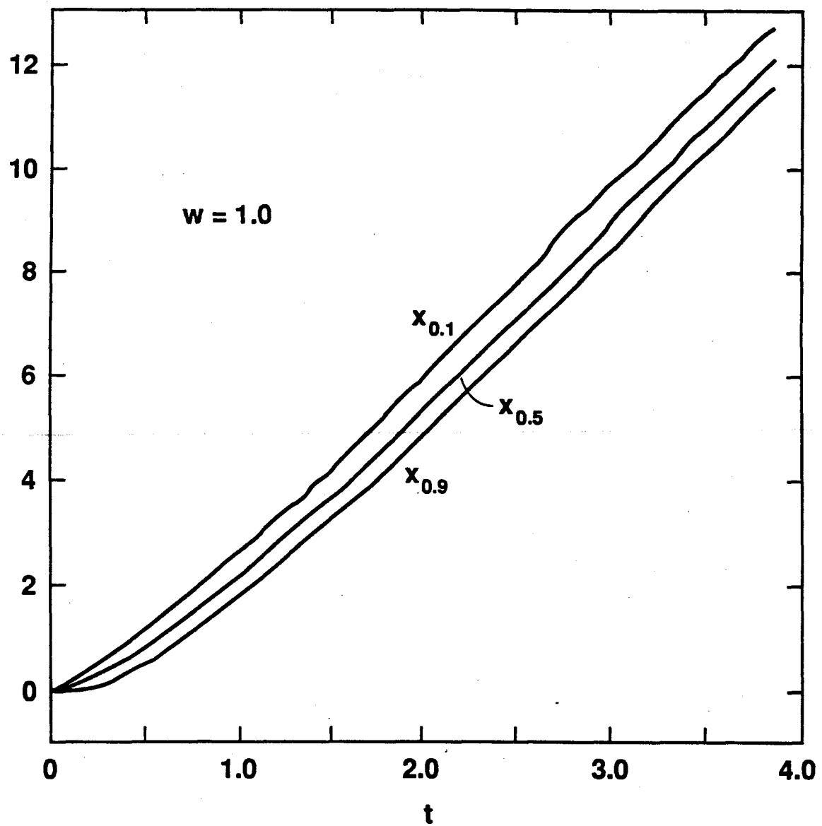
Figure 5: Loci of Points  $x_{0.1}(t)$ ,  $x_{0.5}(t)$ ,  $x_{0.9}(t)$  at Which the Mean Progress Variable is 0.1, 0.5 and 0.9 respectively. Propagation Speed  $w=1.0$ .
