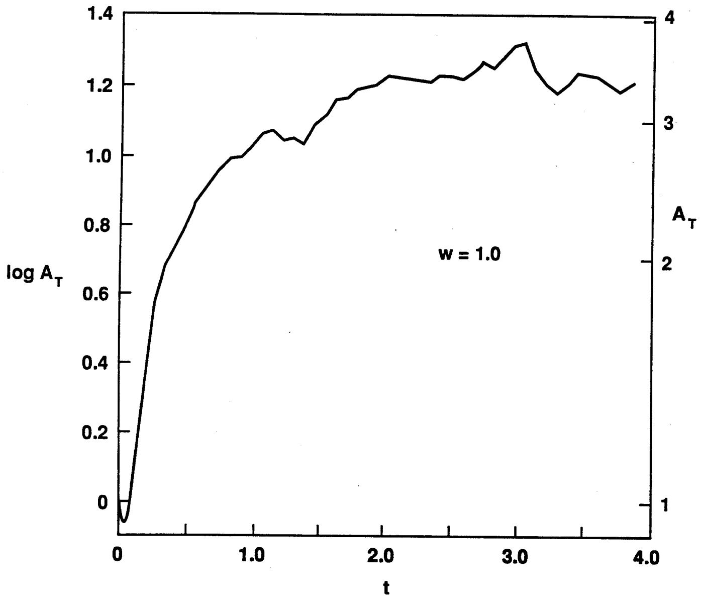
Figure 4: Natural Logarithm of Flame Sheet Area (Per Initial Area) Against Time.
