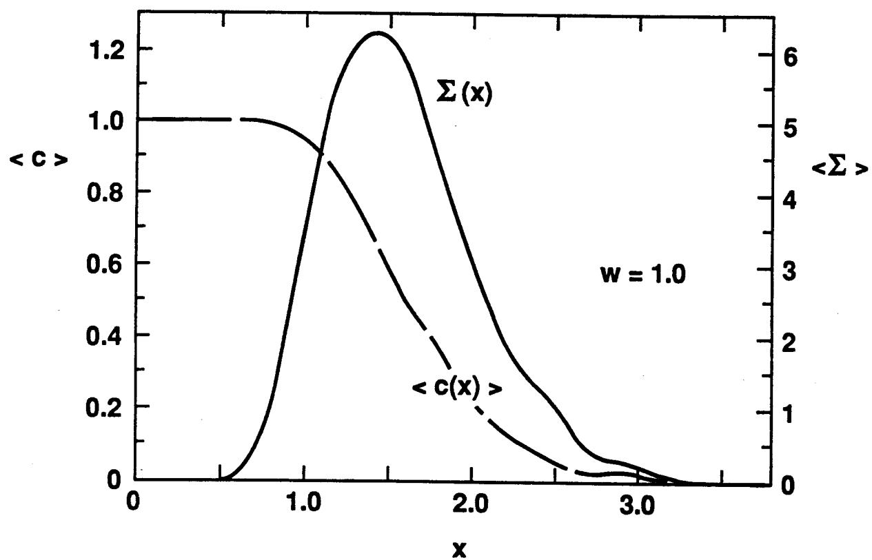
Figure 6: Profiles of Mean Progress Variable and Surface-to-Volume Ratio. (The Origin of  $x$  has been Shifted.)
