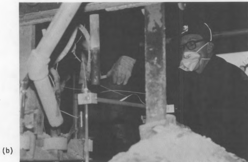
FIGURE 4.35. Voltage Probe Measurements a) Photograph of voltage probes and b) Photograph of voltage probe measurement in progress
