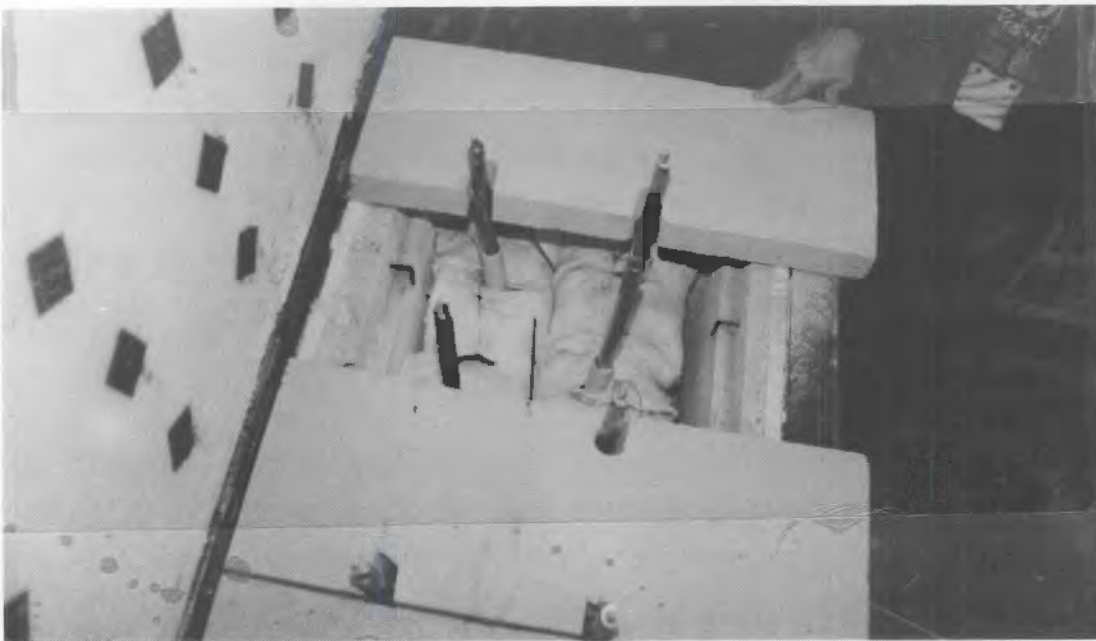
FIGURE 4.6. Photograph of Cermet Anodes in the Preheat Furnace
