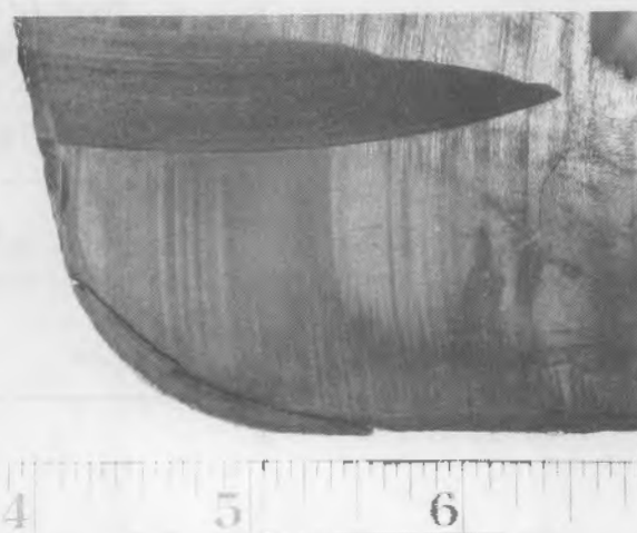
FIGURE 5.12. Photographs of Exterior and Interior of Anode F2 after Testing in the Pilot Cell
