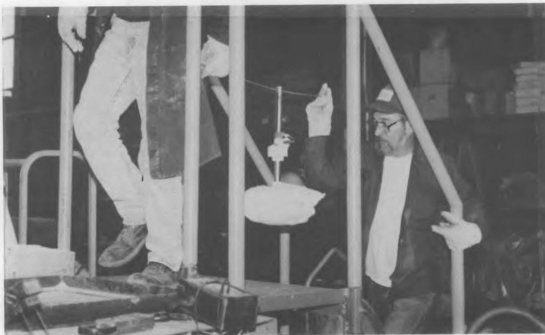
FIGURE 4.7. Transferring a Cermet Anode to the Pilot Cell
