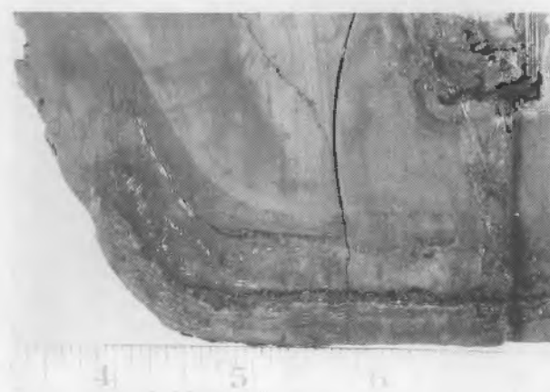
FIGURE 5.10. Photographs of Exterior and Interior of Anode E1 after Testing in the Pilot Cell
