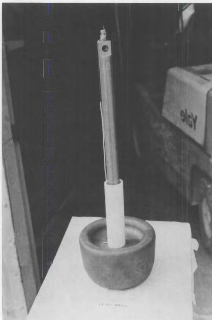
FIGURE 2.6. Photograph of an Assembled Cermet Anode and Connector Rod
