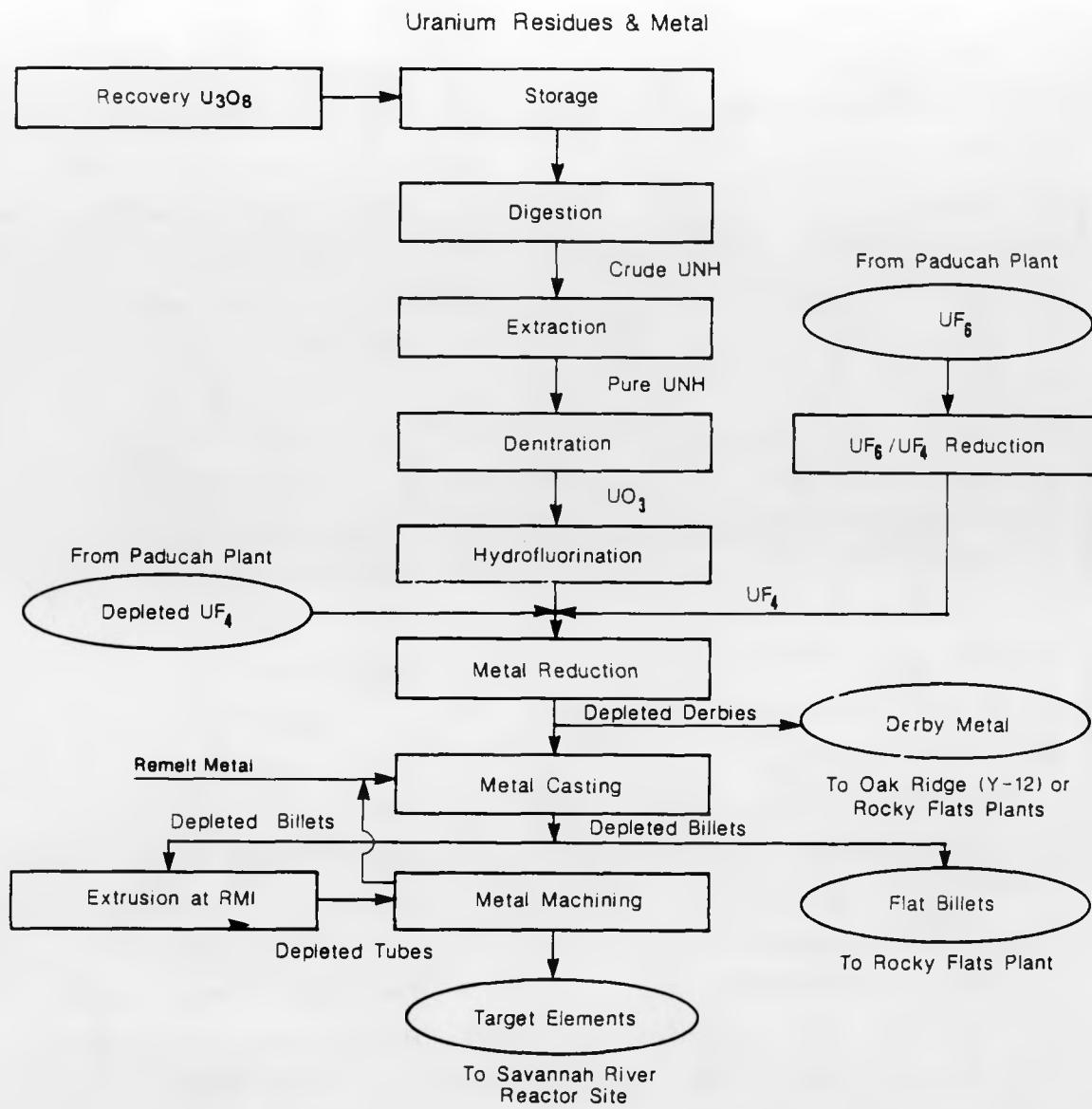
Figure 1-5. Schematic Diagram of the FMPC Process
