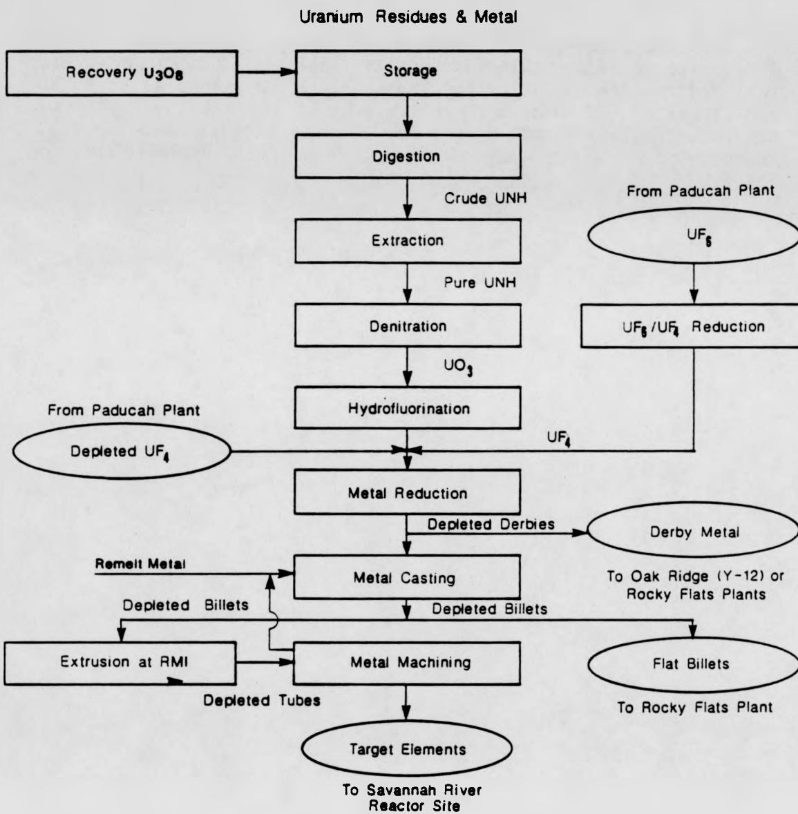
Figure 14-1. Flow of Uranium Compounds and Metal at FMPC
