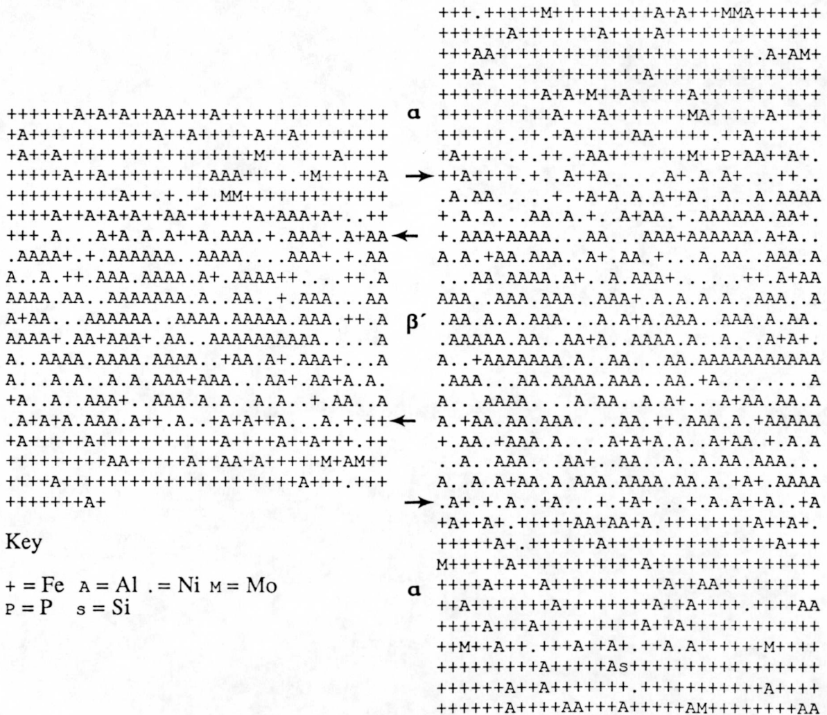
Fig. 5. Character plots of the Fe- 10% Ni- 15% Al- 1% Mo alloy. No segregation of molybdenum to the precipitate matrix interface was evident.
