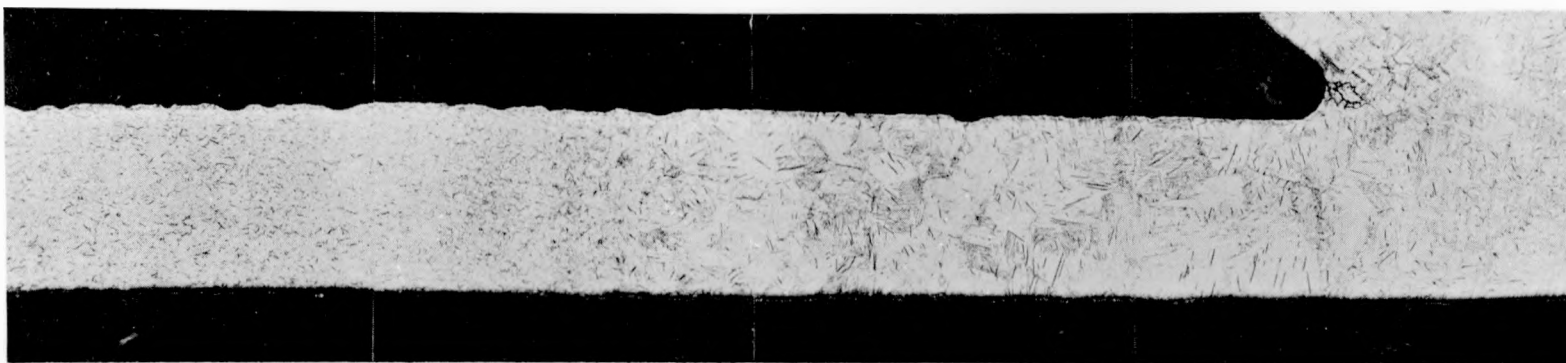
Figure 27. Hydride Concentrations in Alpha and Beta Phase Transition Region in the Upper End Cap. X56
