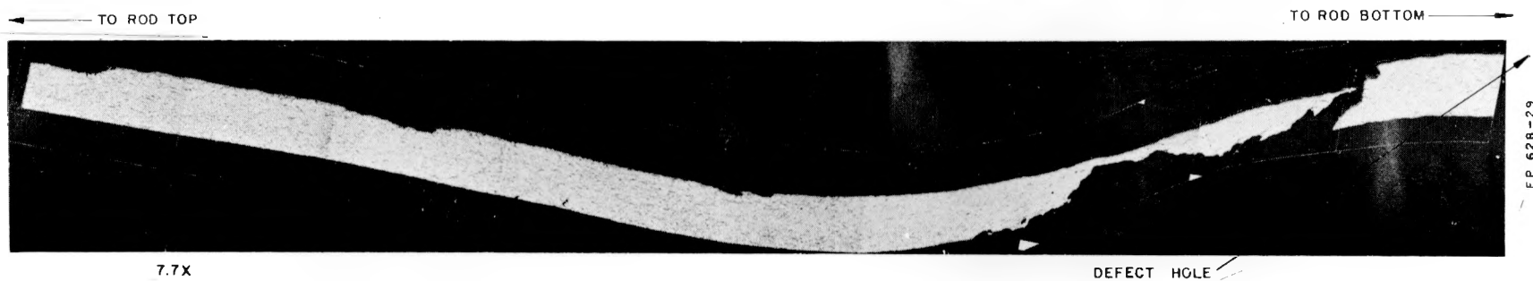
Figure 29. Etched Structure of the Clad in the Plenum Region Where the Rupture Occurred. X26
