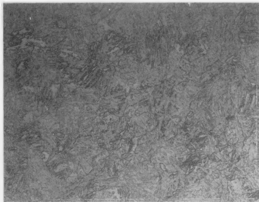
Fig. 9b. Microstructure of Plane B of the A508-4B steel. 400X magnification.
