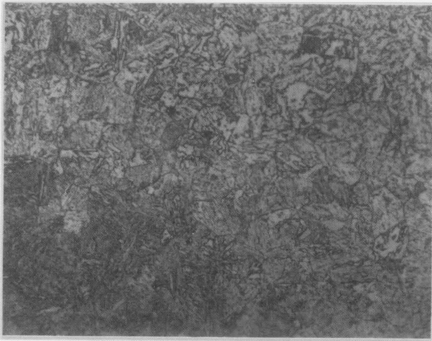
Fig. 8c. Microstructure of Plane C of the A508-4A steel. 400X Magnification.
