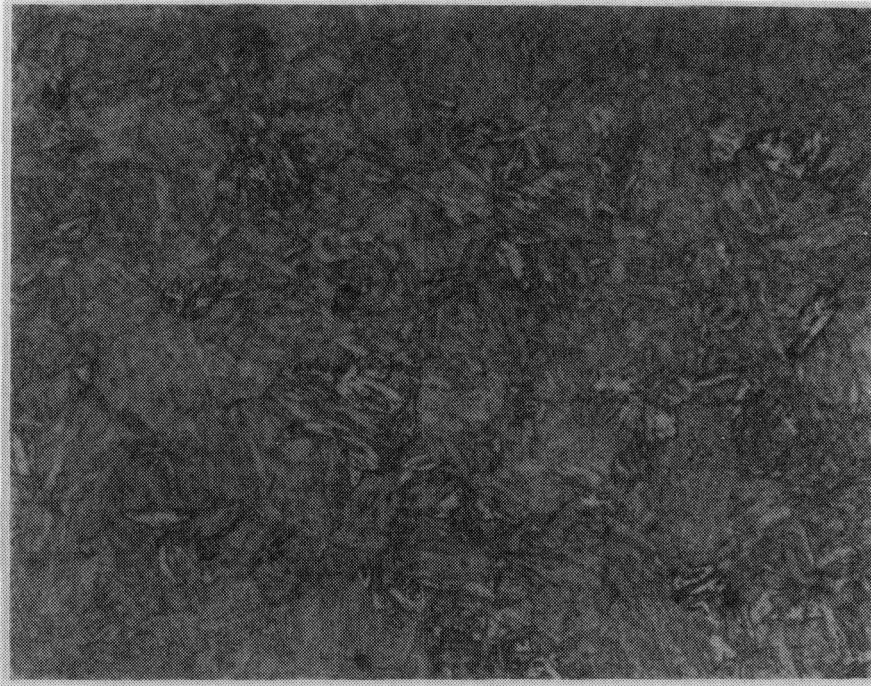
Fig. 8e. Microstructure of Plane E of the A508-4A steel. 400X Magnification.
