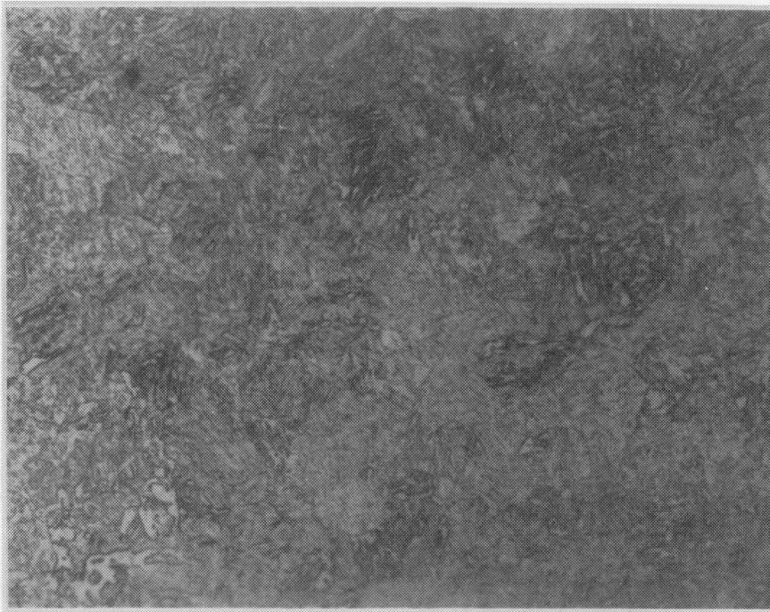
Fig. 8d. Microstructure of Plane D of the A508-4A steel. 400X Magnification.
