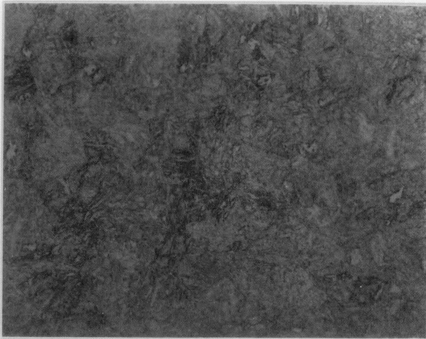
Fig. 8b. Microstructure of Plane B of the A508-4A steel. 400X magnification.
