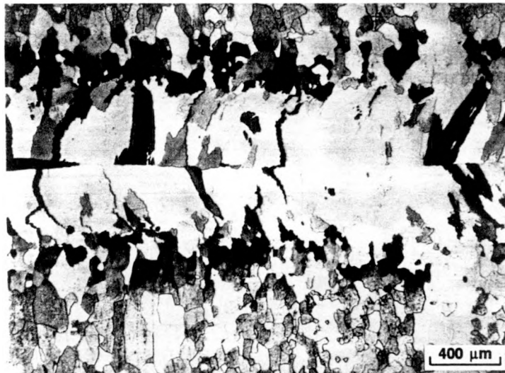
Fig. 1 Fusion zone microstructure of alloy FA-41.
