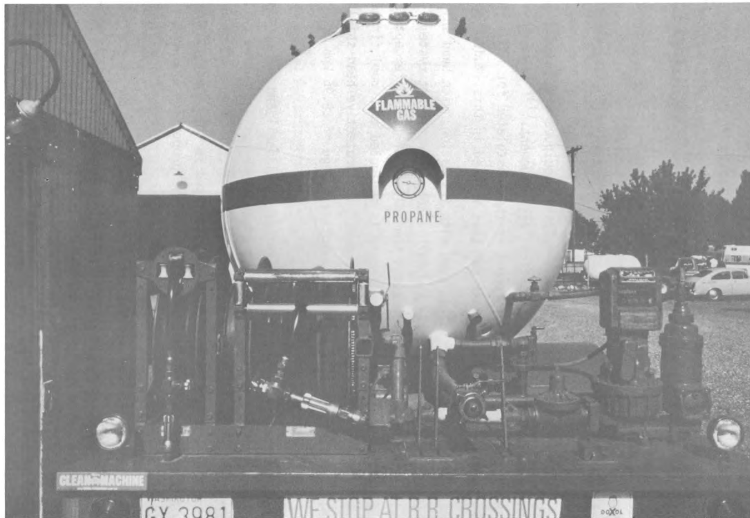
FIGURE B.4. Propane Bobtail Piping Details
