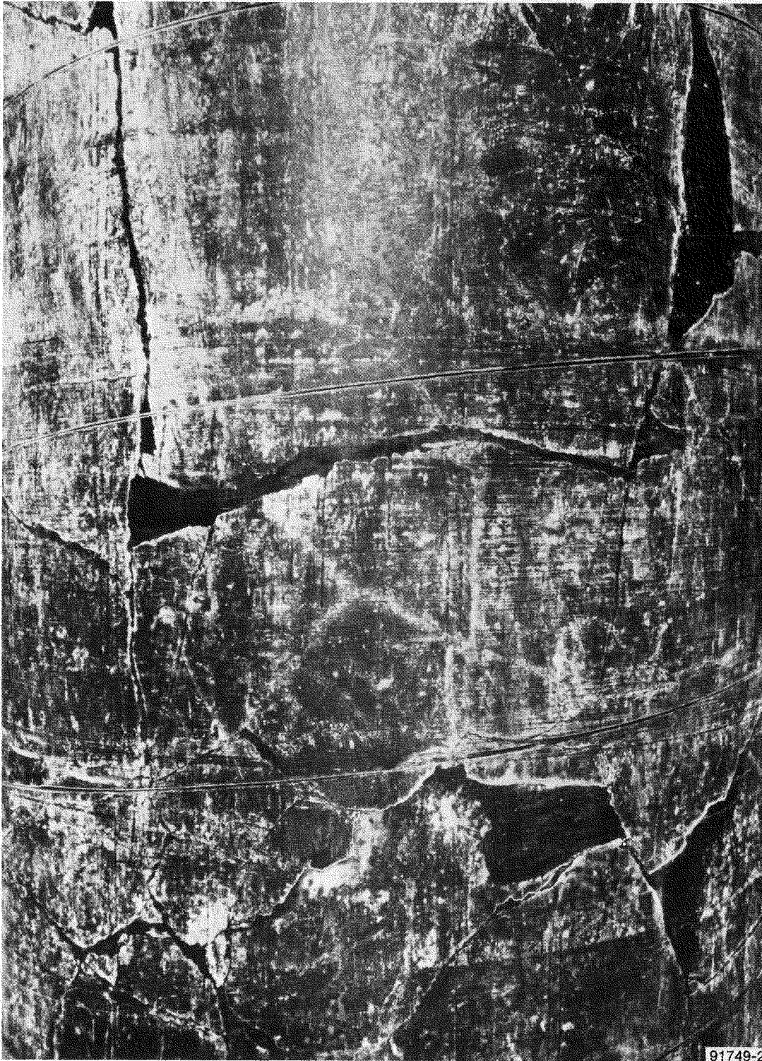
FIGURE 18. Impression Sleeve from Full-Scale Heater Test #2 Main Heater Hole (approximately 23 inches [59 centimeters] long).
