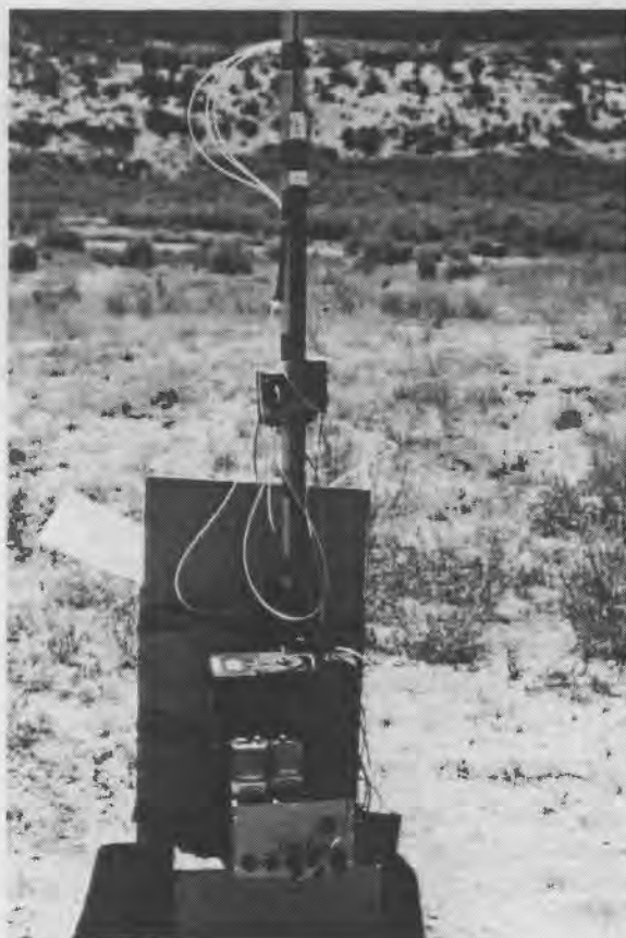
Figure 13. Sampling station of the type used in the 1982 Brush Creek experiments. The Brush Creek stations differed slightly from the one pictured here by having five, instead of three, sampling pumps. The signal encoder, receiver, and sampling pump controller are sitting on a concrete block in front of the cane pole which supports the vertical receiving antenna. The sampling pumps are attached to the cane pole, with inlets at the 1-1/2-m level. The outlet tubes from the pumps go to the cardboard box which contains the individual sampling bags.
