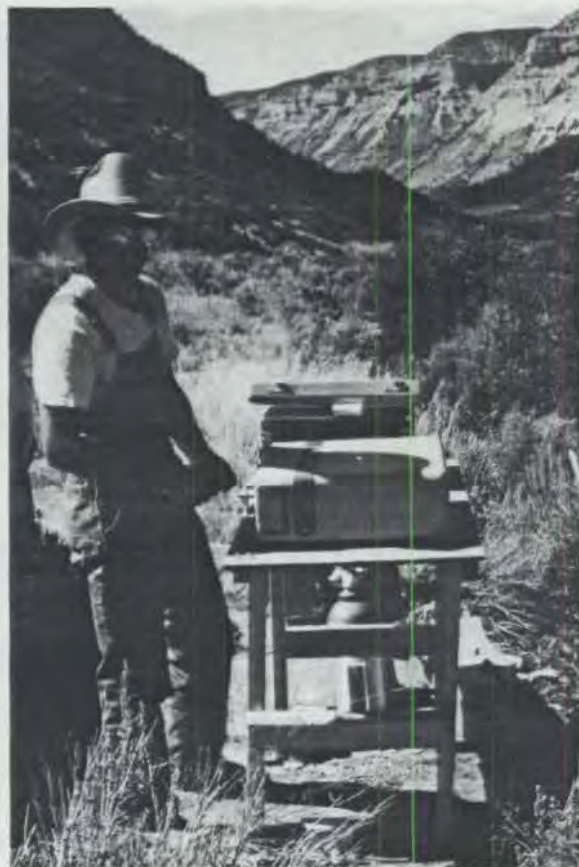
Figure 23. Site GC1 on the west sidewall of Brush Creek. The field portable gas chromatograph and strip chart recorder were operated in the open from wooden table tops by EPA chromatographers.
