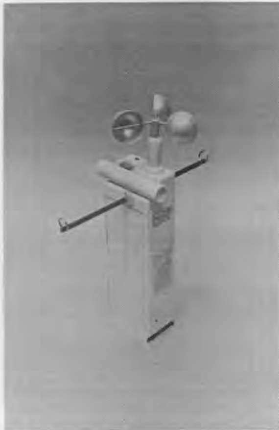
Figure 16. Tethersonde® battery-powered airborne sensor and telemetry package.
