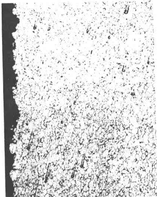
Figure E-2 Micrographs of 347 and 316L Parent Metal Tensile Specimens With \text{HNO}_3 -HF Acid Treatment After 8 Month Air and 9 Month Molten Salt Exposure at 580^\circ\text{C} ( 1075^\circ\text{F} )
