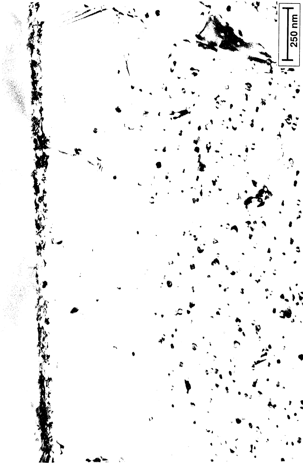
Figure 13. Helium-bearing plate (3.5 mm below weld overlay). Bubble-free zone adjacent to an incoherent twin boundary.
