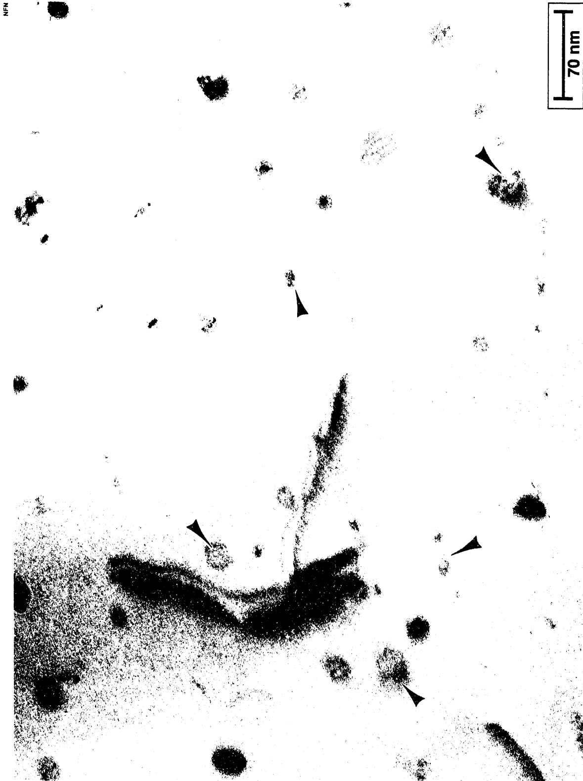
Figure 12. Helium-bearing plate (3.5 mm below weld overlay). Helium bubbles (at arrows) associated with dislocation loops.
