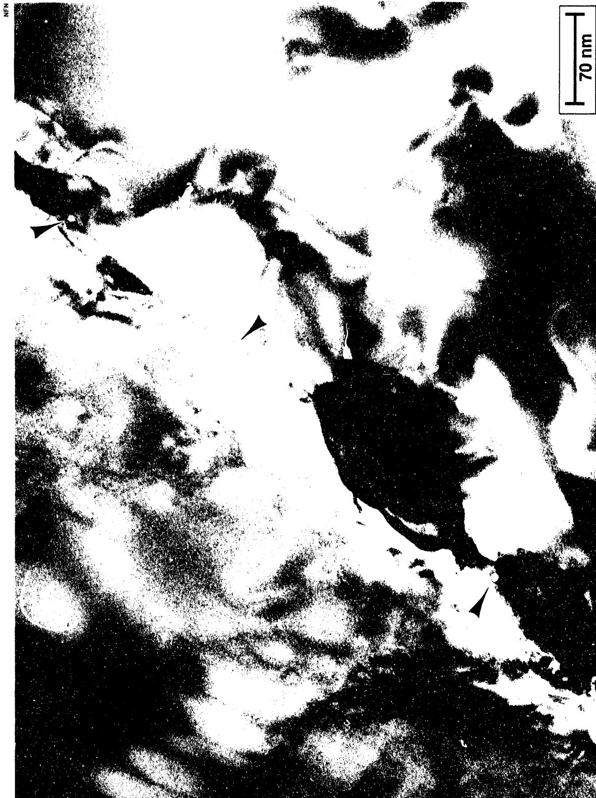
Figure 17. Helium-bearing plate (2.3 mm below weld overlay). Helium bubble distribution on a grain boundary. Several large bubbles have been arrowed. The dark particles on the boundary are carbide precipitates.
