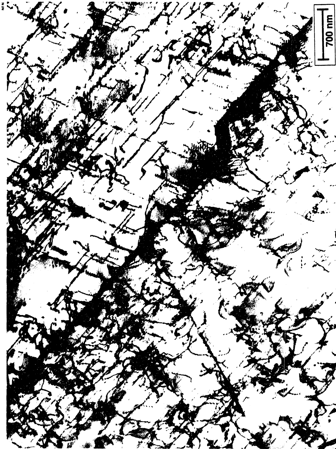
Figure 5. As-received plate with weld overlay. Increased dislocation density in the vicinity of a coherent twin boundary at ~1 mm below an overlay.
