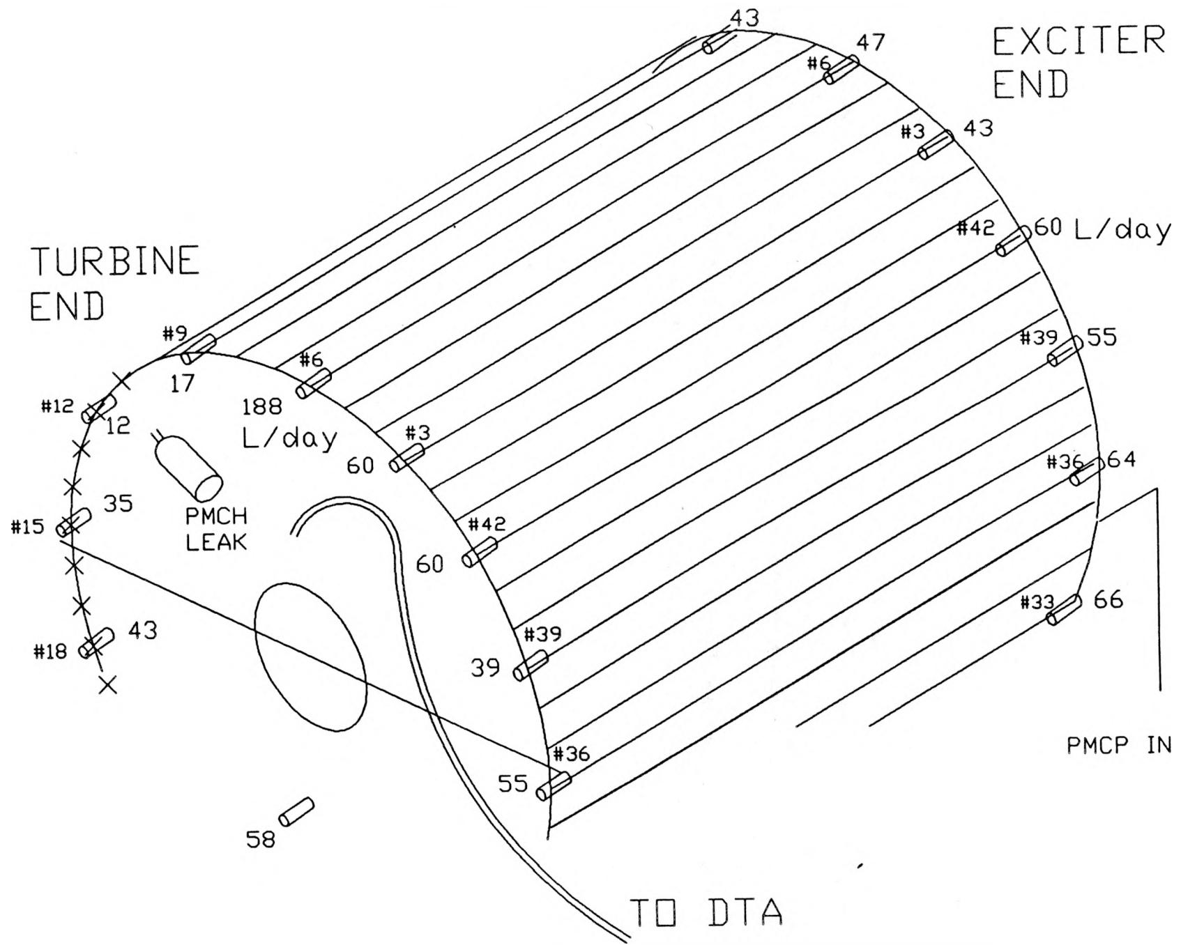
Figure 1: Experimental Setup
