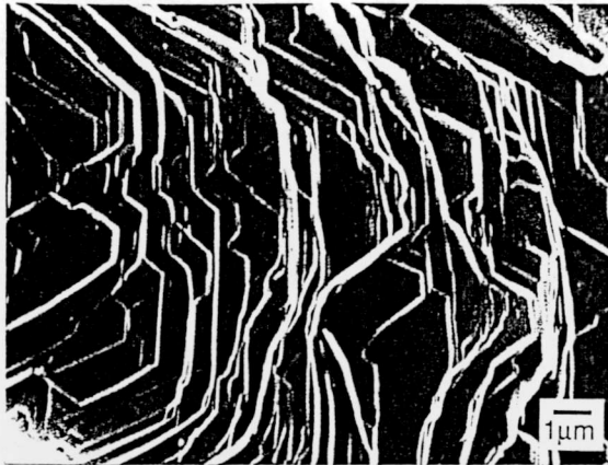
Figure 1. Scanning electron micrograph showing sheet-like nature of boric acid crystals on the wear scar of a boric acid pin.
