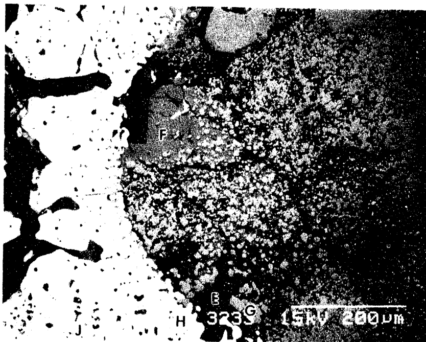
Figure 114. Region of corroded Inconel showing the \text{AlF}_3 grain boundary phase (A).
