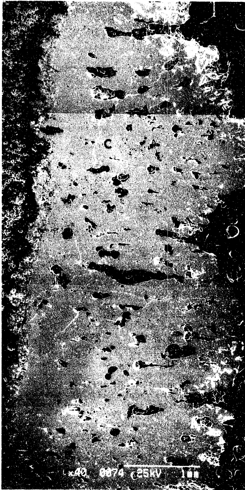
Figure 61. The Cerrox coating on the bottom of Anode C1 is thick and continuous.
