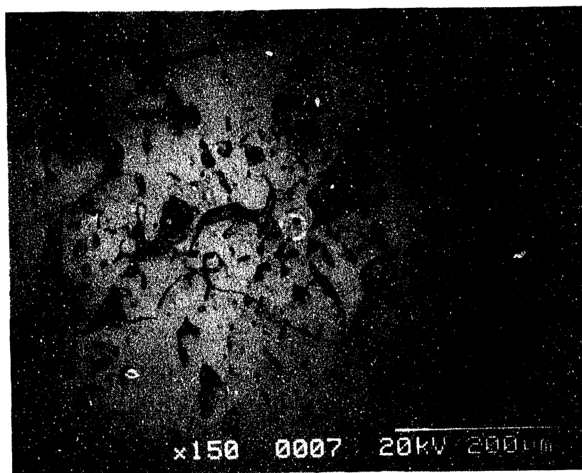
Figure 67. A close-up of the "sawtooth" pattern within the coating on Anode A2.
