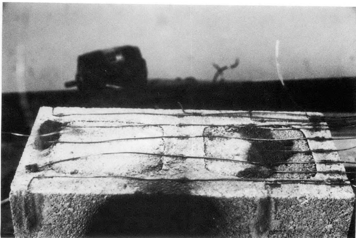
Figure 7. Thermocouples embedded in concrete block, ready to be installed in structure two
