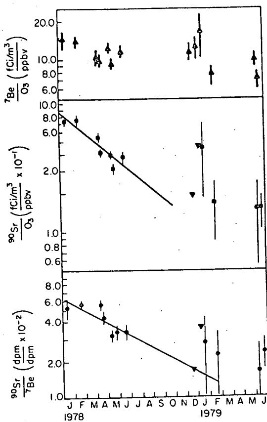
Fig. 19.  $^{7\text{Be}}/\text{O}_3$ ,  $^{90\text{Sr}}/\text{O}_3$  and  $^{90\text{Sr}}/^{7\text{Be}}$  ratios measured in stratospheric samples ( $\text{O}_3 > 200 \text{ ppbv}$ ) collected at 10 to 12 km. Estimated uncertainties are indicated by vertical bars. Solid lines are regression fits to exponential decay curves for the 1978 measurements as explained in the text.
