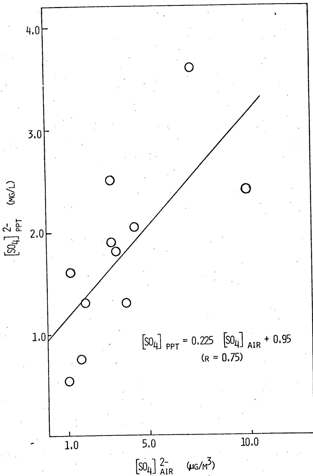
Fig. 25. Relationship of atmospheric particulate  $SO_4^{2-}$  -  $[SO_4]^{2-}$  air - and atmospheric precipitation  $SO_4^{2-}$  -  $[SO_4]^{2-}$  PPT - concentration at Whiteface Mountain (1979).
