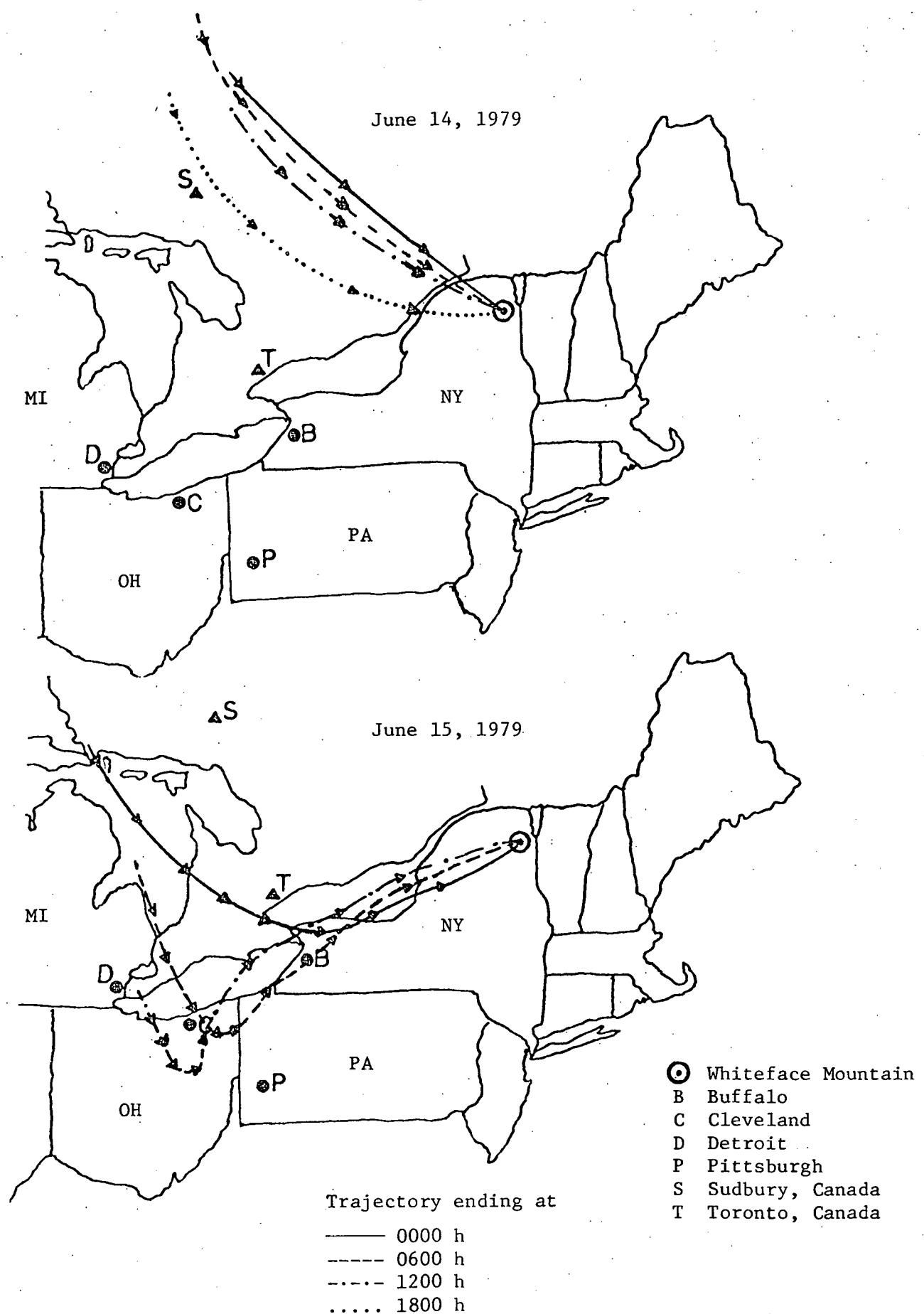
Fig. 9. Backward surface (0.4-1.4 km) trajectories for air arriving at Whiteface Mountain on June 14 and 15, 1979. Each arrow head represents a 6-h interval.
