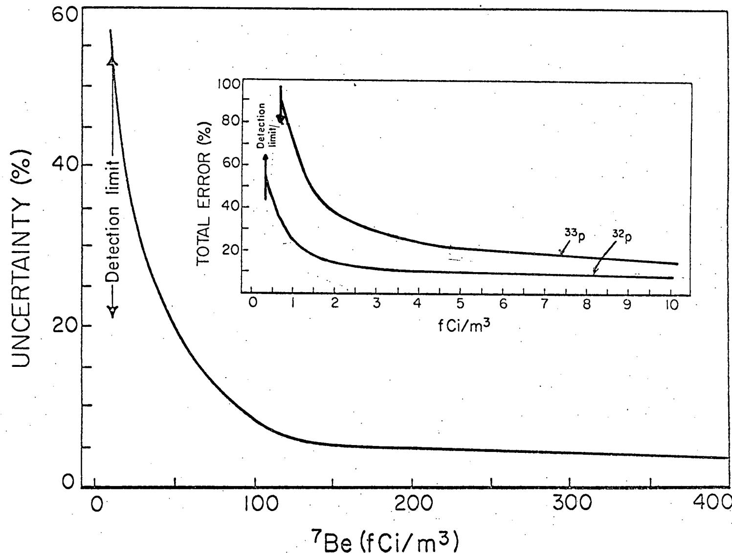
Fig. 2. Estimated uncertainties in  $^{7}\text{Be}$ ,  $^{32}\text{P}$  and  $^{33}\text{P}$  concentrations measured in 24-h high-volume air samples (Average total air volume sampled  $\approx 1800$  standard  $\text{m}^3$ ).
