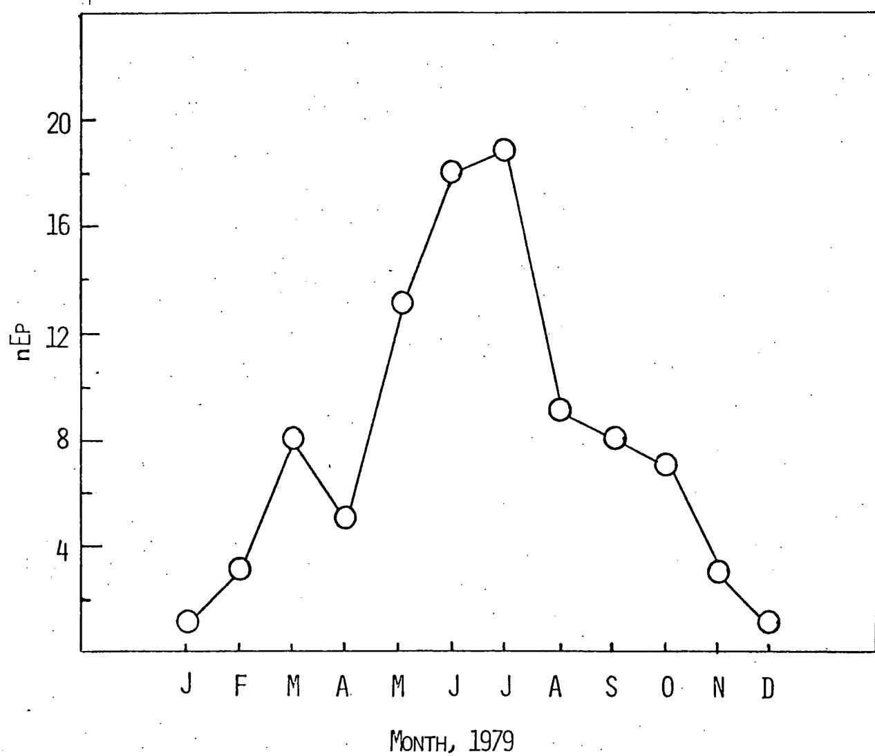
Fig. 22. Frequency (nEp) of monthly occurrences of episodic cases with  $\text{SO}_4^{2-}$  concentrations  $\geq 5 \mu\text{g}/\text{m}^3$  and greater.
