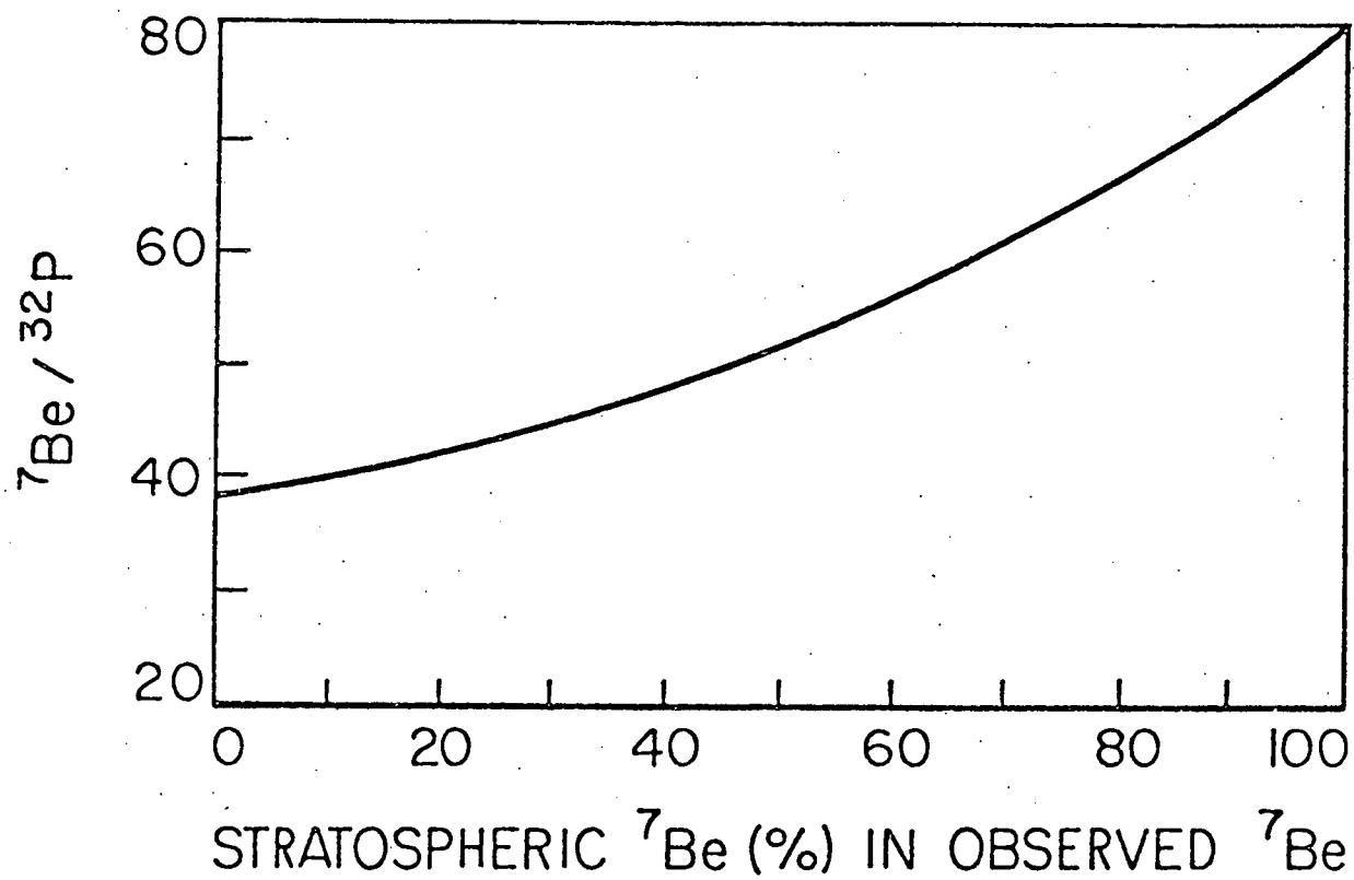
Fig. 6.  $^{7\text{Be}}/^{32\text{P}}$  activity ratio for mixed stratospheric ( $^{7\text{Be}}/^{32\text{P}} = 80$ ) and tropospheric ( $^{7\text{Be}}/^{32\text{P}} = 38$ ) air masses as a function of the % of the resultant  $^{7\text{Be}}$  concentration originating in the stratosphere.
