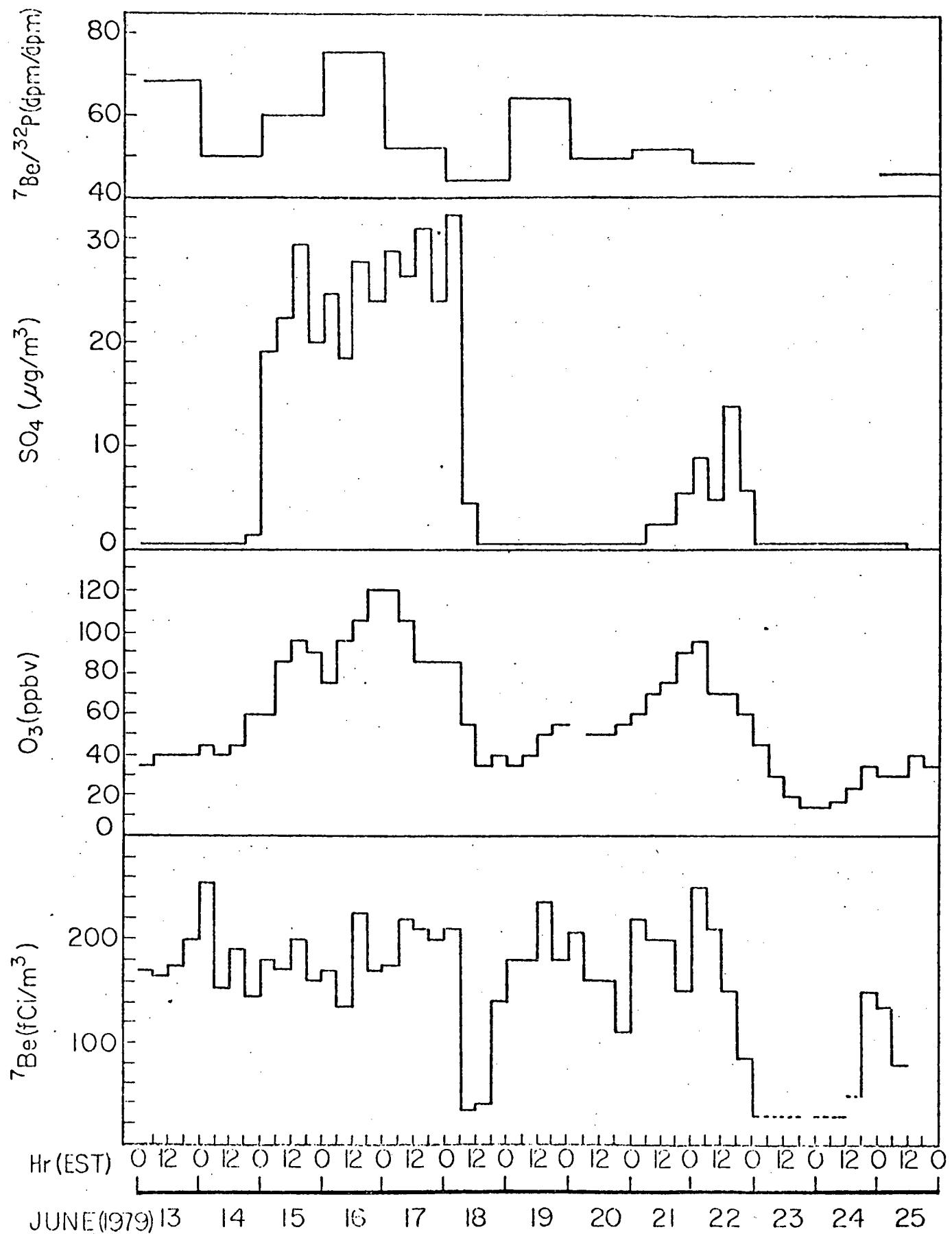
Fig. 8. 6-h  $^{7\text{Be}}$ ,  $\text{O}_3$  and  $\text{SO}_4^{2-}$  concentration and 24-h  $^{7\text{Be}}/^{32\text{P}}$  ratios measured at Whiteface Mountain between June 13 and 25, 1979.
