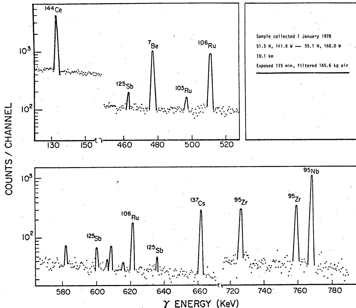
Fig. 4. Representative Ge(Li)  $\gamma$  spectrum of a stratospheric air sample collected by NASA's Global Atmospheric Sampling Program. Significant peak intensities are highlighted by solid curves, and radionuclides assigned.
