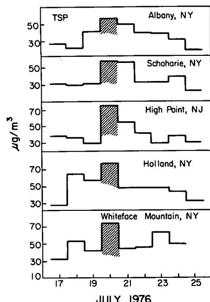
Fig. 3. Total solid particulate measurements during July 1976 in upstate New York and New Jersey. Shading designates the day of peak concentrations (July 20).
