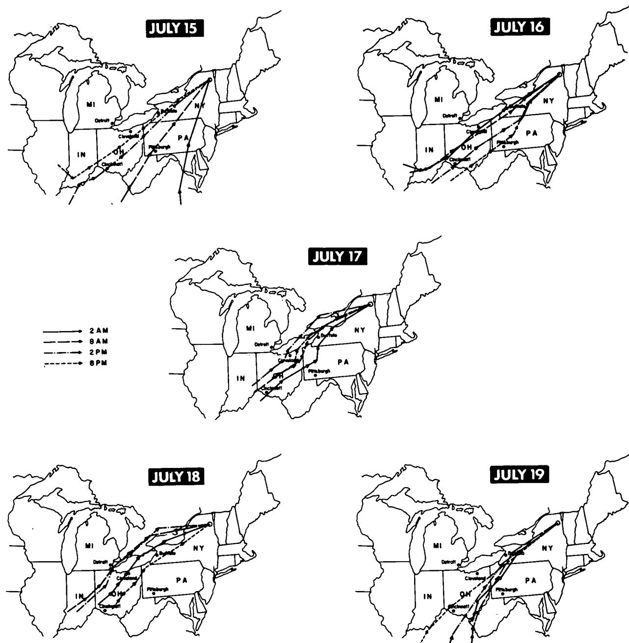
Fig. 2. Trajectories of air masses reaching Whiteface Mountain on July 15-19, 1975. Each arrow indicates a 12-hour movement of the air mass.
