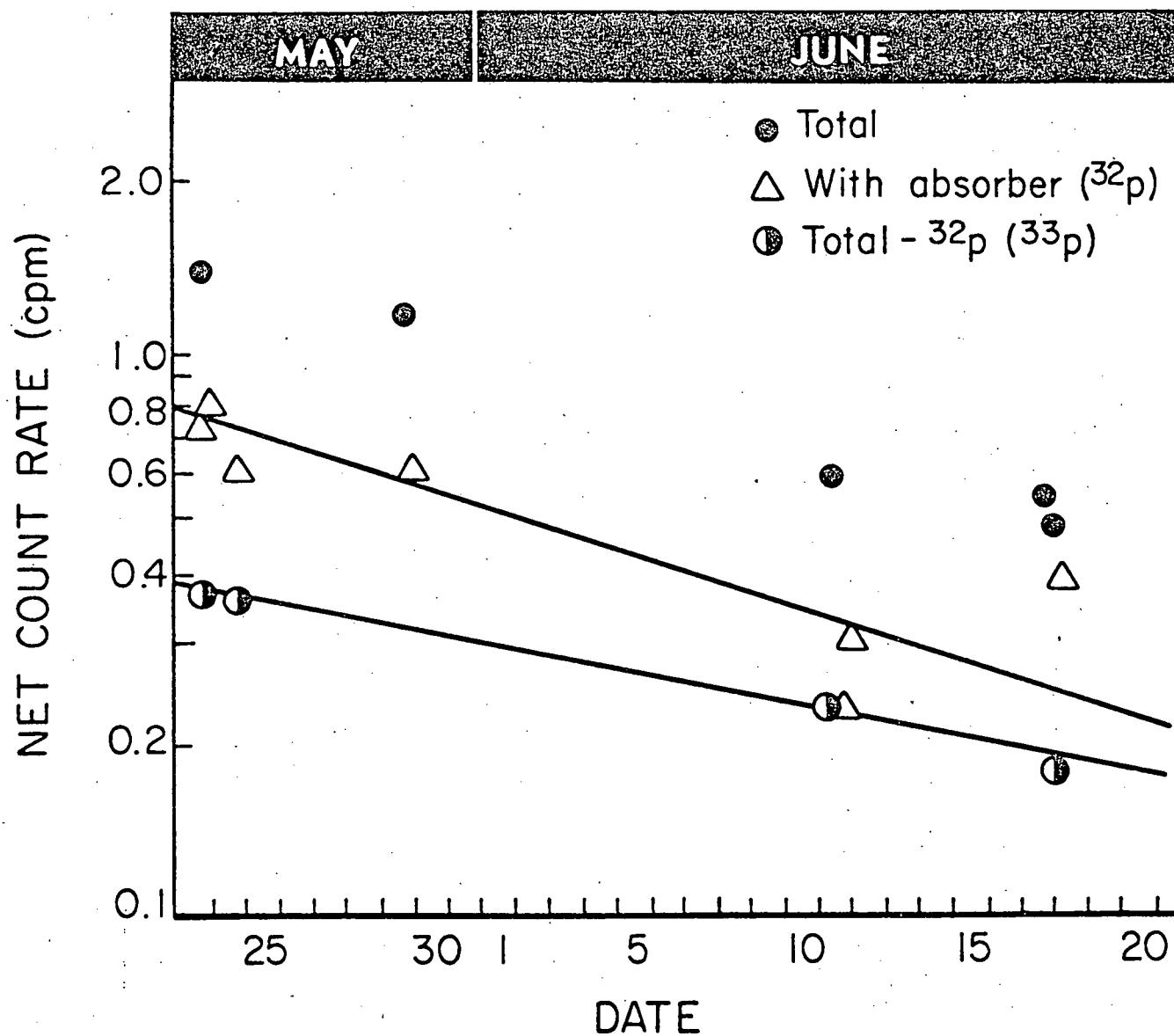
Fig. 3. Representative decay curve fits to  $^{32}\text{P}$  and  $^{33}\text{P}$  counting data from 24-h high-volume air samples. The upper and lower lines respectively correspond to 14.3- and 25-d decay.
