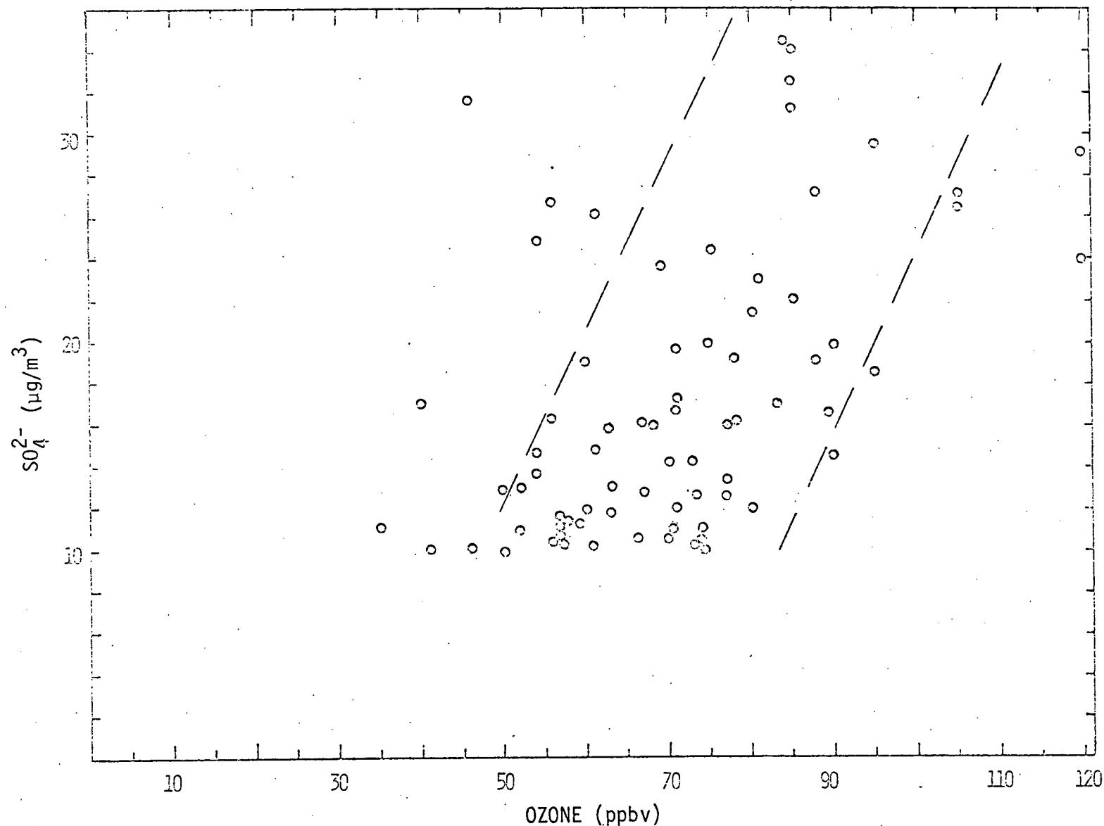
Fig. 7. Relationship between  $\text{O}_3$  concentration in ambient air versus  $\text{SO}_4^{2-}$  concentration in air particulates at Whiteface Mountain showing that for  $\text{SO}_4^{2-}$  concentration  $> 10 \mu\text{g}/\text{m}^3$ ,  $\text{O}_3$  concentration exceeds 50 ppbv. The dashed lines are drawn parallel to the best least squares fit for the points encompassed in the field.
