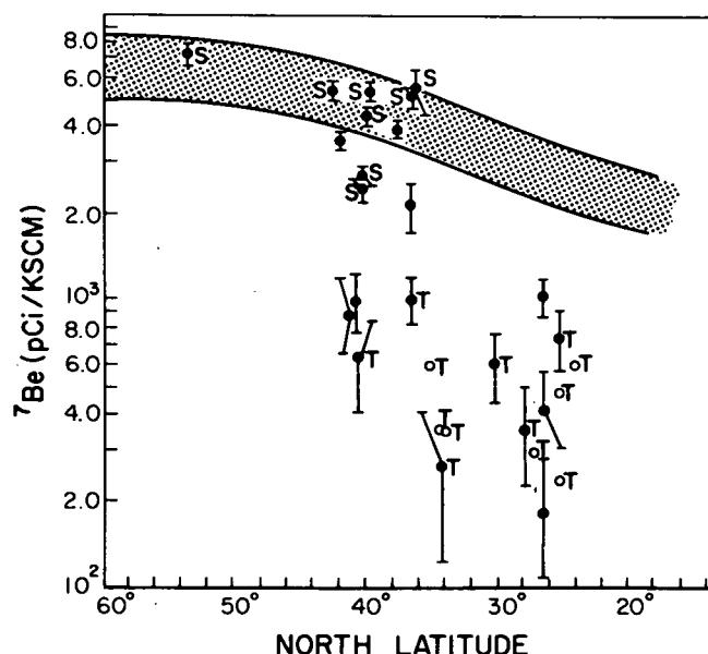
Figure 1.  $^{7}\text{Be}$  concentrations at 10 to 12 km altitude versus average latitude. Uncertainties are shown as vertical bars; open circles correspond to upper-limit measurements. The designations S and T indicate stratospheric and tropospheric samples respectively, as explained in the text. The shaded curve is the theoretical  $^{7}\text{Be}$  saturation activity for a stable atmosphere at 10- to 12 km altitude (Lal and Peters, 1967).
