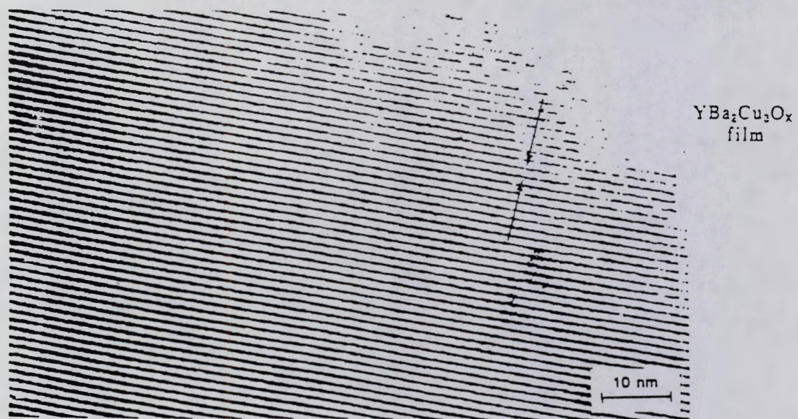
Figure 5. High magnification TEM shows the lattice spacing of the YBa 2 Cu 3 O x thin film.
