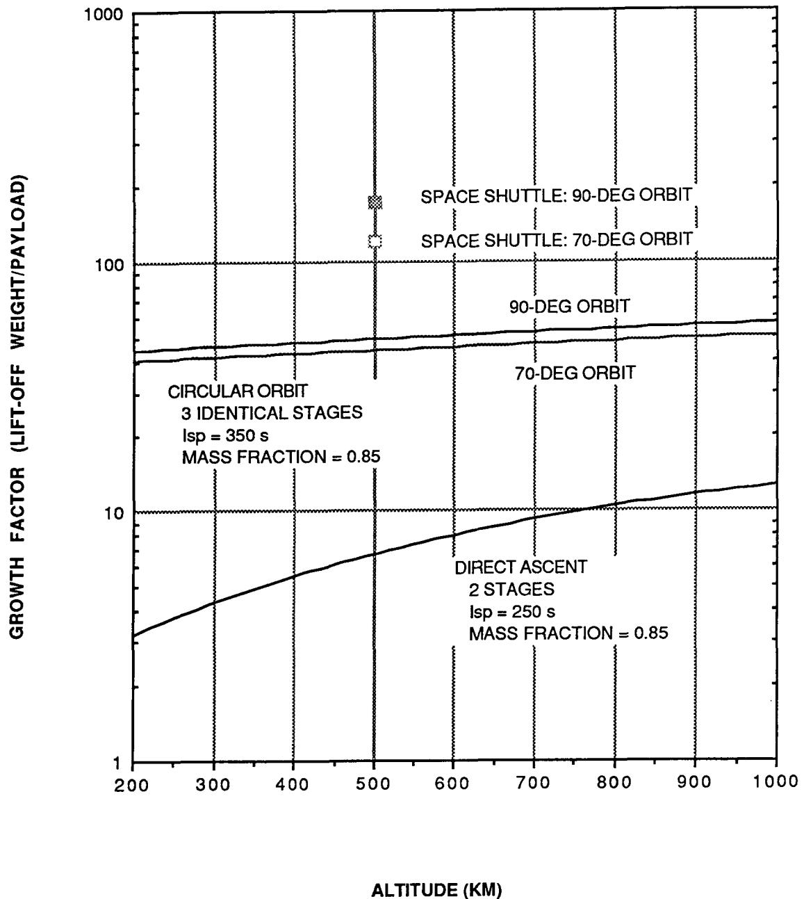
**FIG. A-3 ROCKET WEIGHT RATIO**
