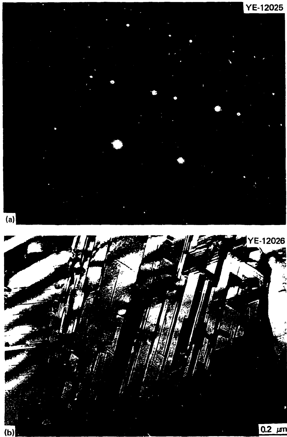
Fig. 6. Transmission Electron Micrograph of Coating SC472, Showing a Heavily Faulted Grain (Below) and the Diffraction Pattern from This Region (Above). The streaks in the diffraction pattern result from the high stacking fault density.
