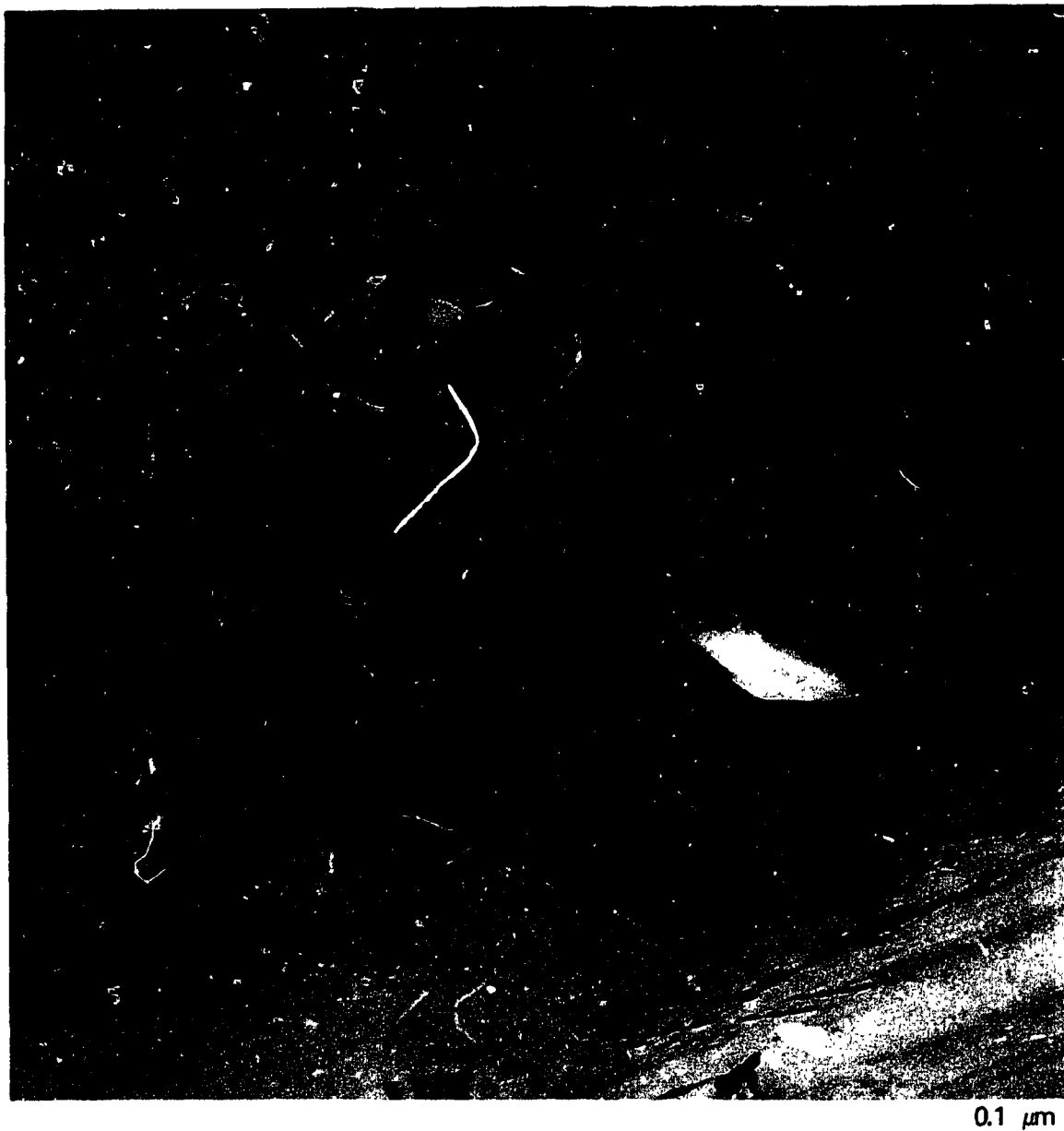
Fig. 5. High-Magnification Transmission Electron Micrograph of Coating SC476 Showing Small Cavities Along a Grain Boundary.
