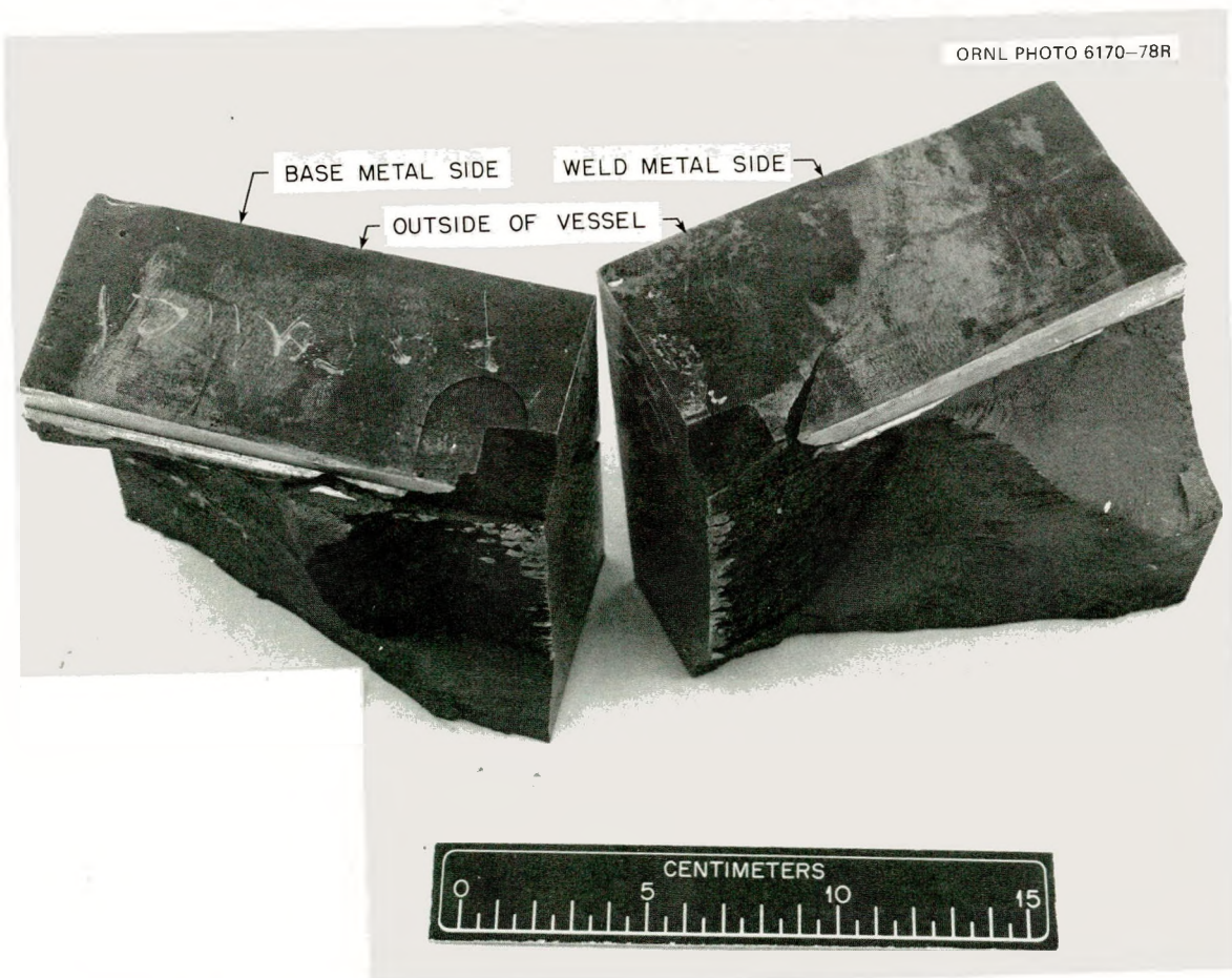
Fig. 5.4. V-7B fracture surfaces in slab Q exposed by splitting the chilled slab.
