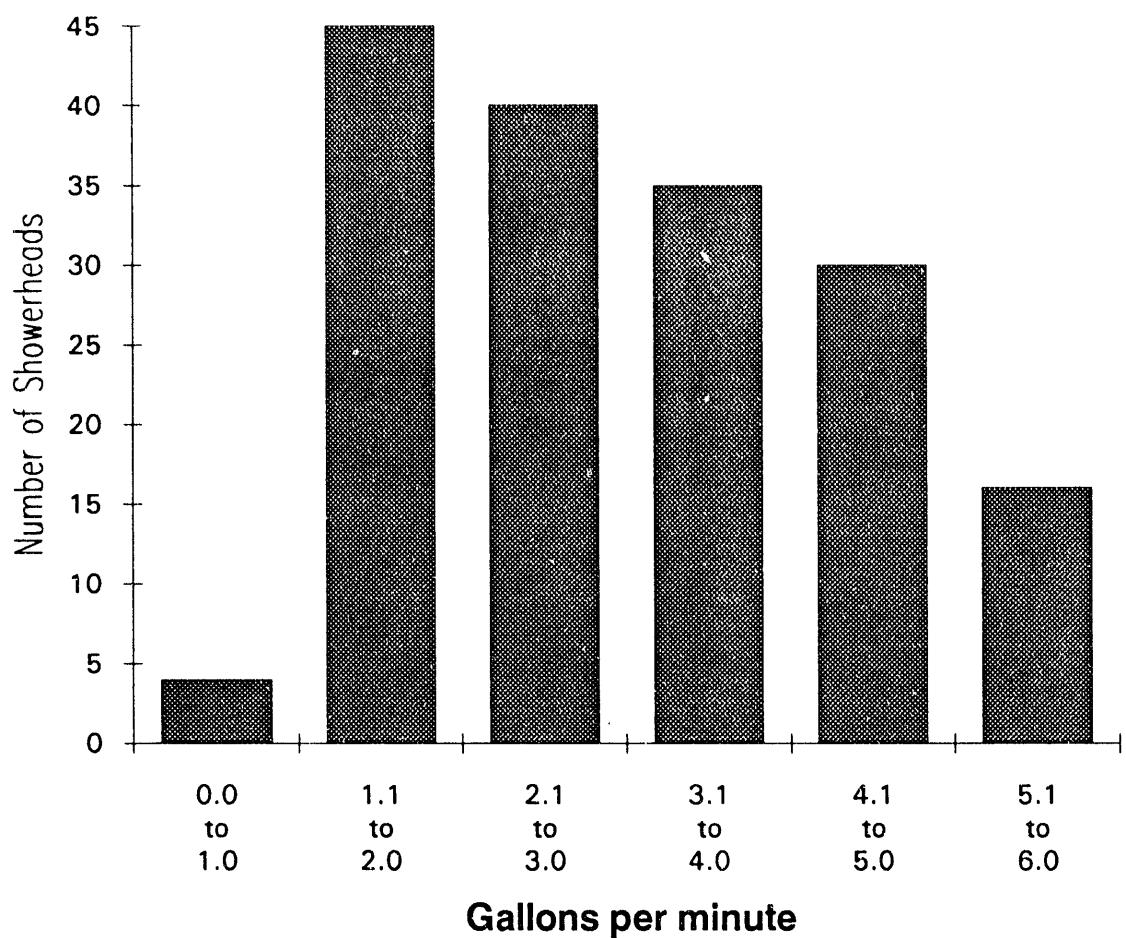
**Figure 1. Flow Rates for Preretrofit Showerheads**
