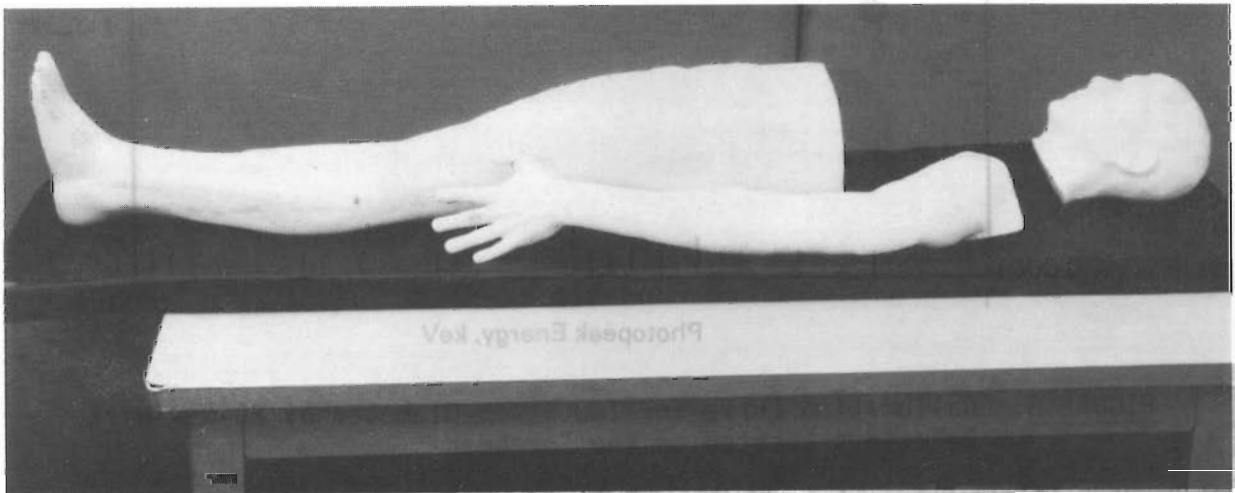
FIGURE 9. Head, Leg, and Arm Phantoms Constructed of Tissue-Equivalent Polyurethane
