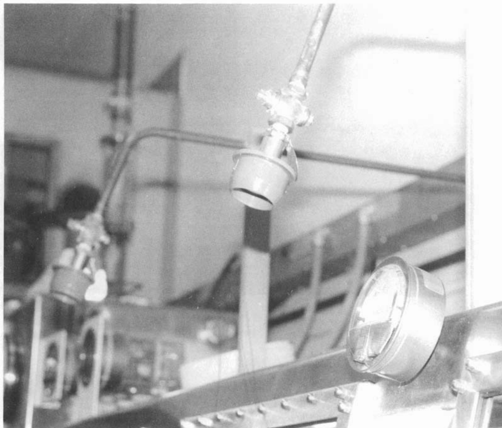
FIGURE 8. Fixed Head Air Sampling Lines in Position Above a Glove Box
