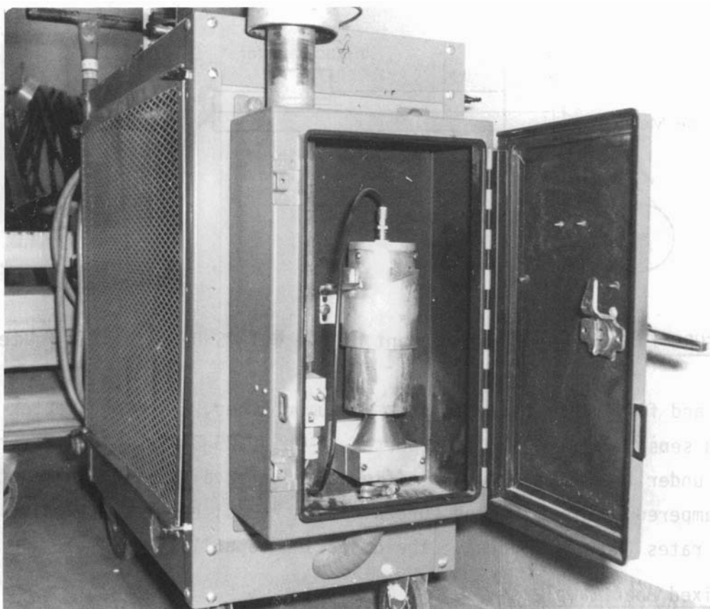
FIGURE 6. Portable Impactor-Type Alpha CAM with Light-Tight Box Door Open
