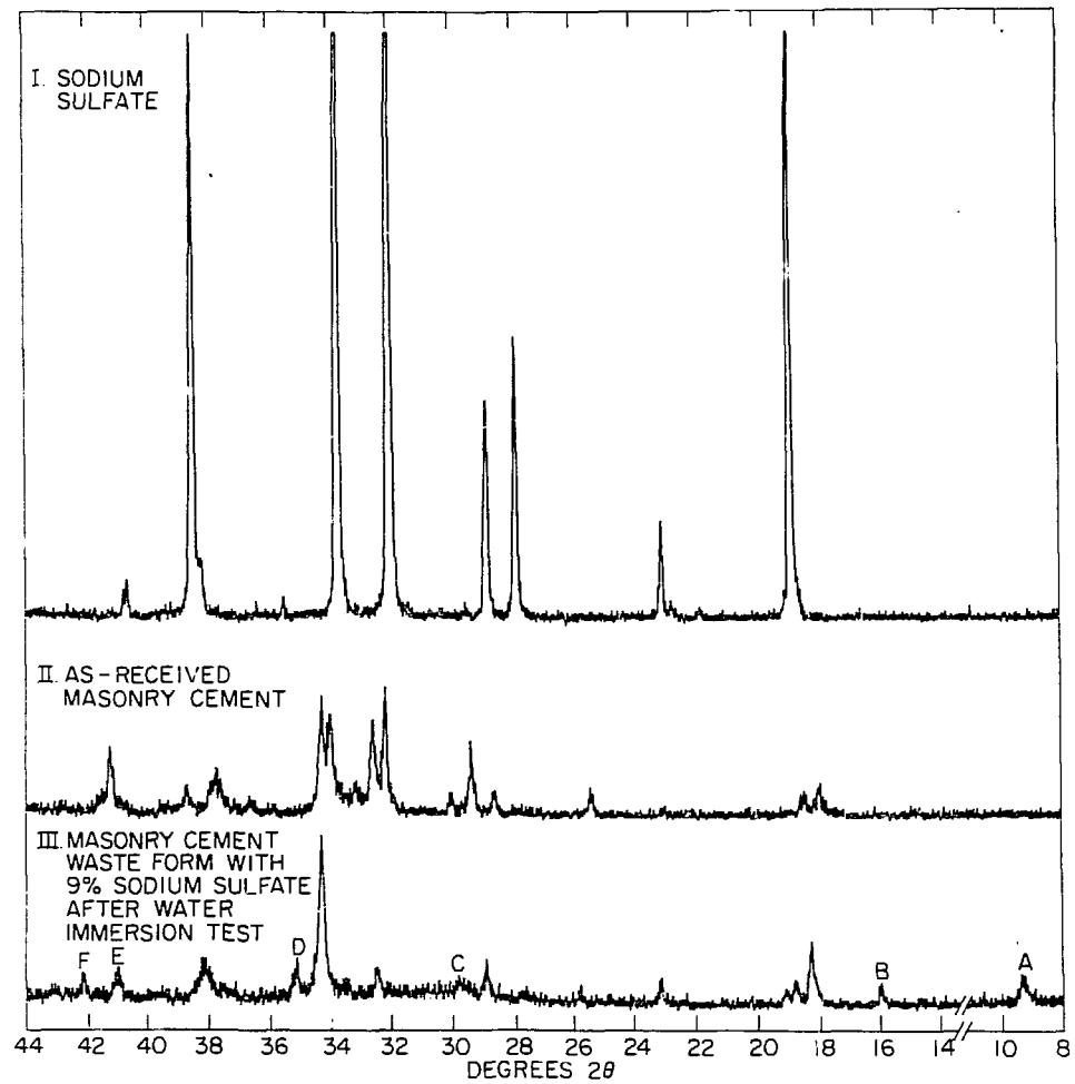
Fig. 3 X-ray diffractograms comparing different components of masonry cement-sodium sulfate waste form. Peak A, B, C, D, E, F of spectrum III are typical of calcium aluminum sulfate hydrate.
