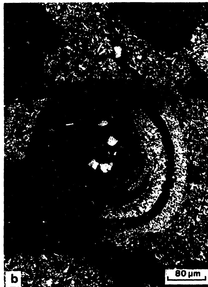
Fig. 22. Optical micrographs of Triso-coated \text{PuO}_{1.81} particles irradiated to 63% FIMA. (a) Bright field; (b) polarized light.
