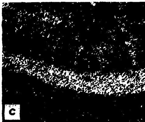
Fig. 9. X-ray displays of Triso-coated UC_2 plus Mo-Ru-Pd particle (batch OR-2809) polished to midplane after being heated at 1873 K for 50 h in a 27.8 K/mm temperature gradient. (a) Backscattered electron image of breached SiC layer; (b) Ru L_\alpha ; (c) Pd L_\alpha ; (d) U M_\alpha .
