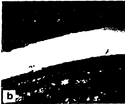
Fig. 5. Triso-coated \text{UO}_2 plus Mo-Ru-Rh particle (batch OR-2806) polished to midplane after being heated at 2008 K for 215 h in a 27.8 K/mm temperature gradient. (a) Optical micrograph; (b) back-scattered electron image of SiC layer; (c) Ru L_\alpha x rays; (d) Rh L_\beta x rays.
