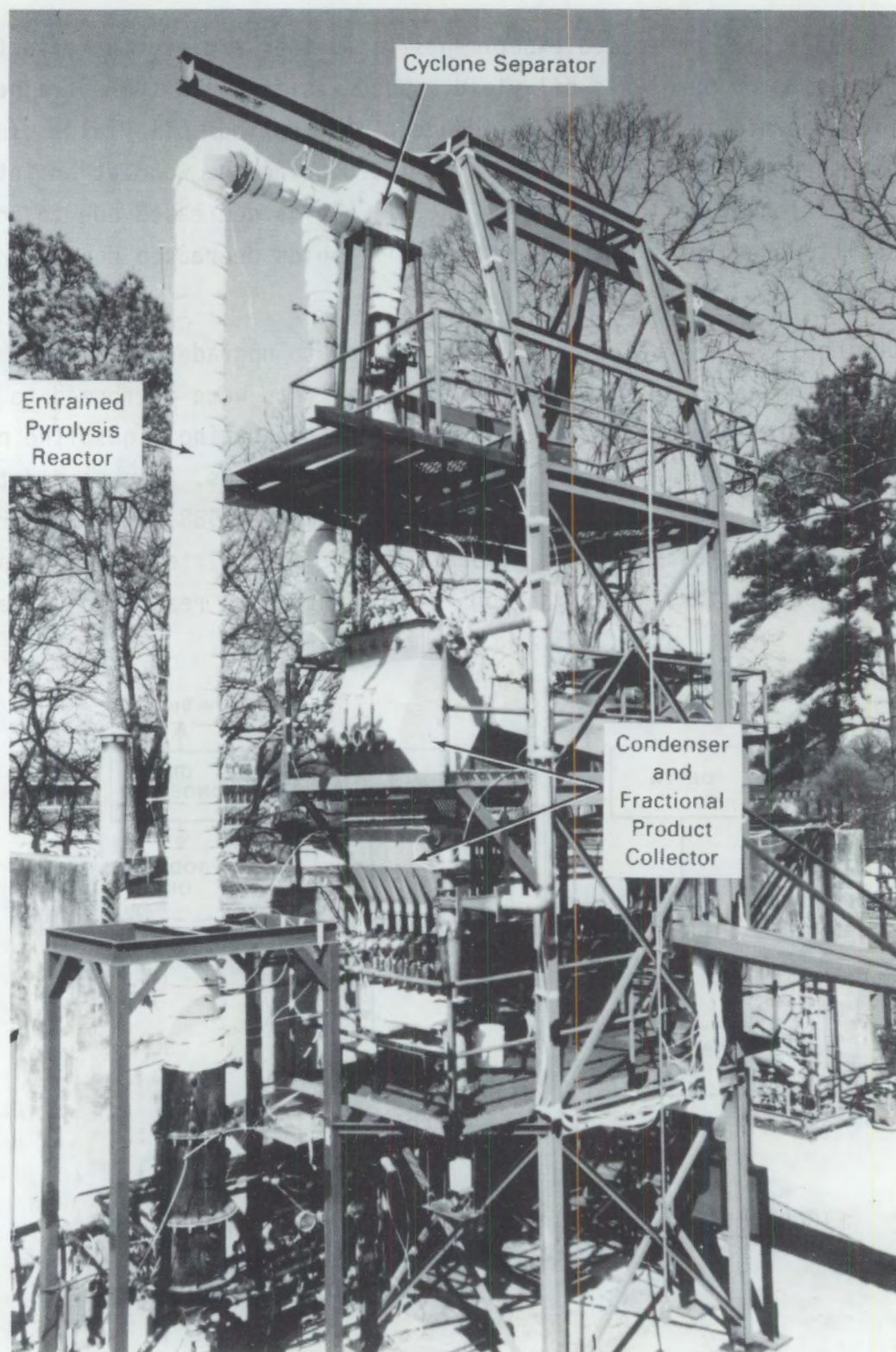
FIGURE 12. View of Georgia Tech Research Corporation Pyrolysis Reactor
