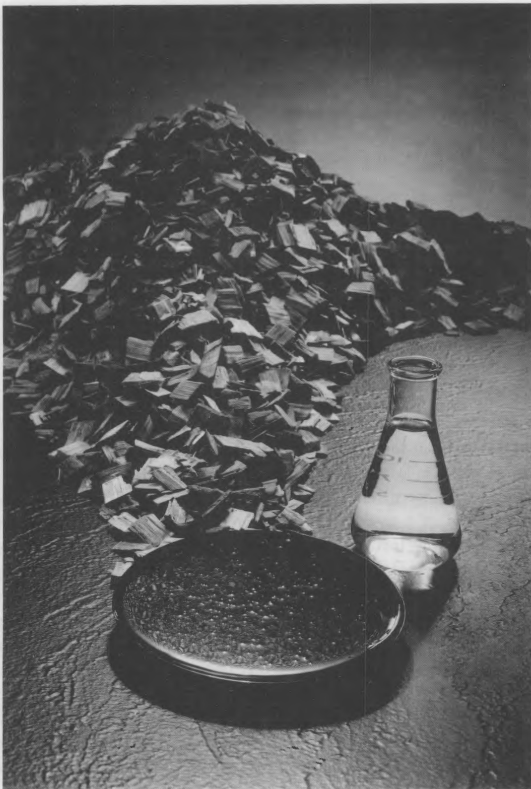
FIGURE 7. Biomass is Converted First to a Biocrude Oil and Then Upgraded to Gasoline Hydrocarbons
