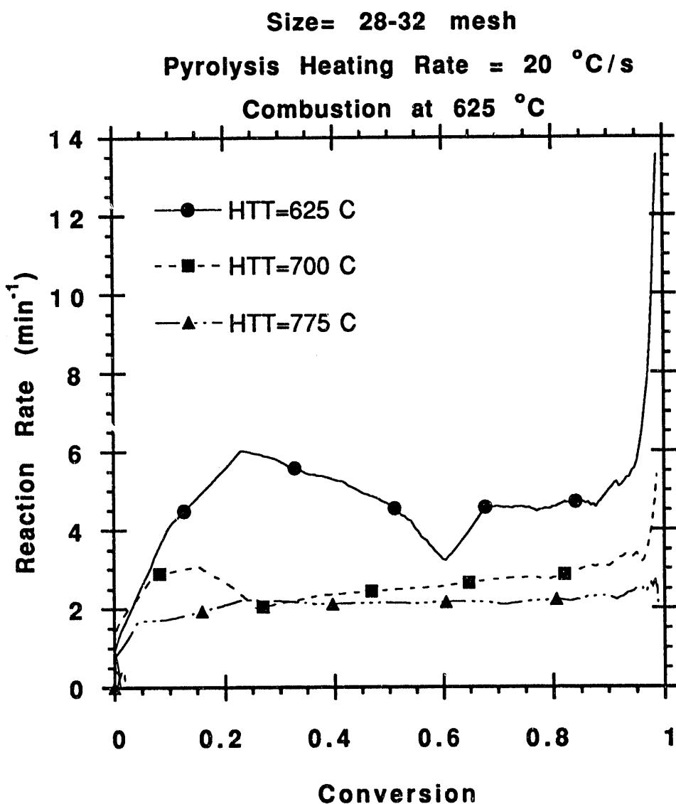
Figure 7: Reaction rate  $R_s$  vs. conversion patterns for combustion at 625 °C of chars produced at various heat treatment temperatures and a pyrolysis heating rate of 20 °C/s. Coal particle size was in the 28-32 mesh range for all samples.
