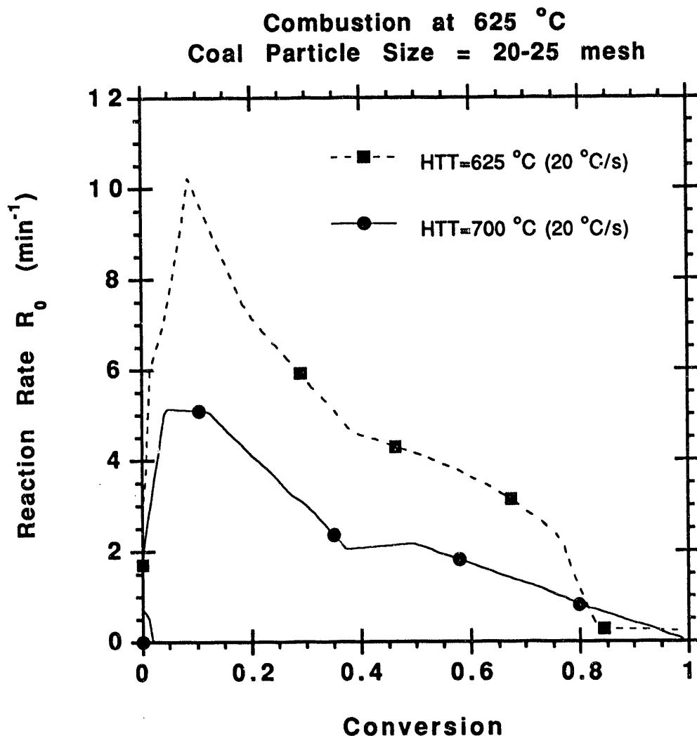
Figure 9: Reaction rate  $R_0$  vs. conversion patterns for combustion at 625 °C of chars produced at two heat treatment temperatures and a pyrolysis heating rate of 20 °C/s. Coal particle size was in the 20-25 mesh range for both samples.
