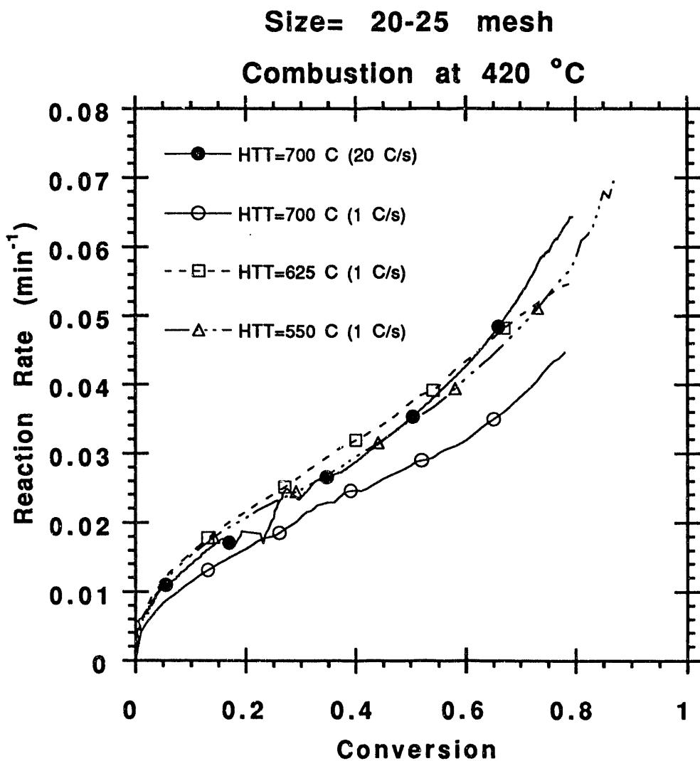
Figure 2: Intrinsic reaction rates for chars produced at various pyrolysis heating rates and heat treatment temperatures from coal particles in the 20-25 mesh size range.
