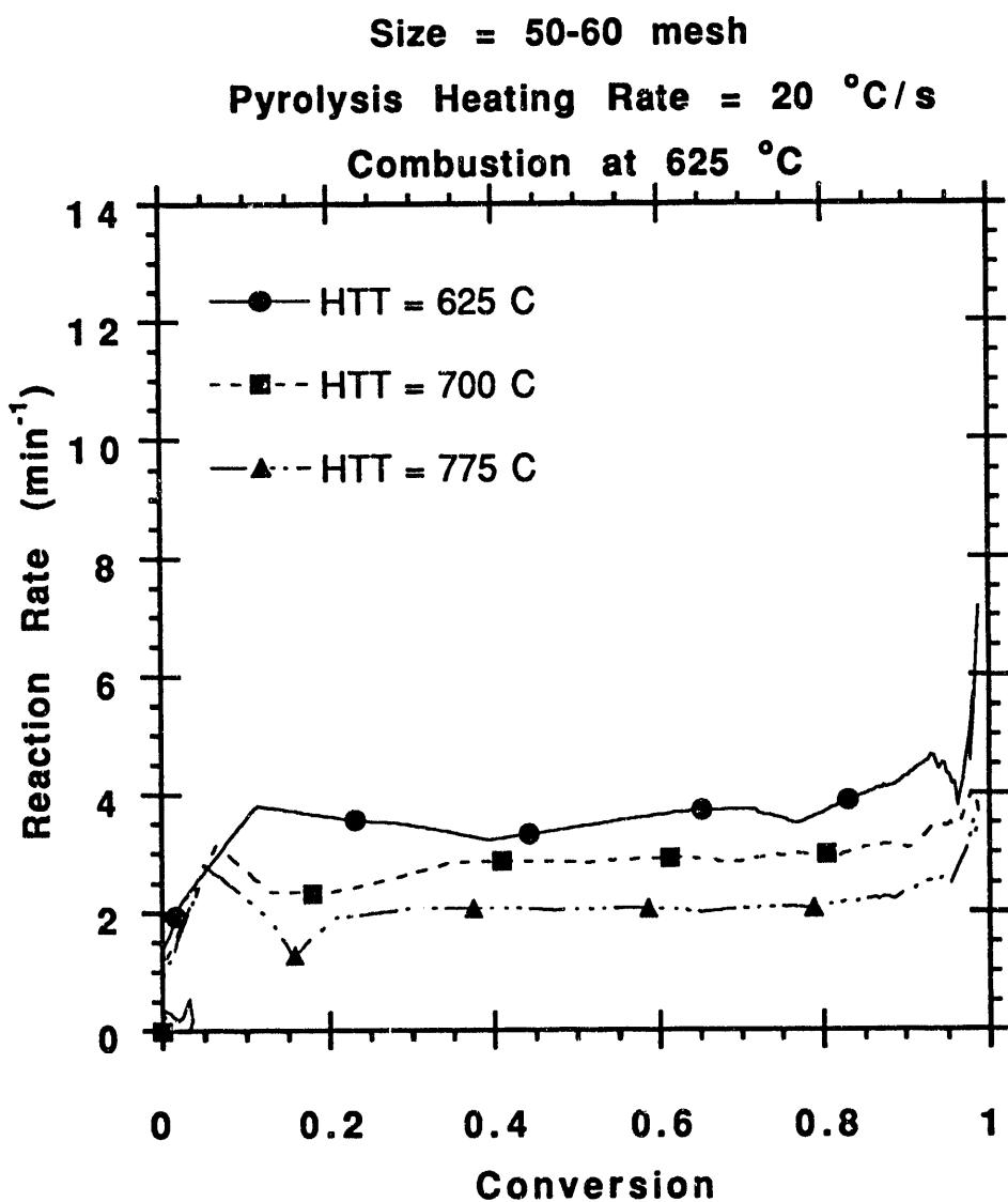
Figure 6: Reaction rate  $R_s$  vs. conversion patterns for combustion at 625 °C of chars produced at various heat treatment temperatures and a pyrolysis heating rate of 20 °C/s. Coal particle size was in the 50-60 mesh range for all samples.
