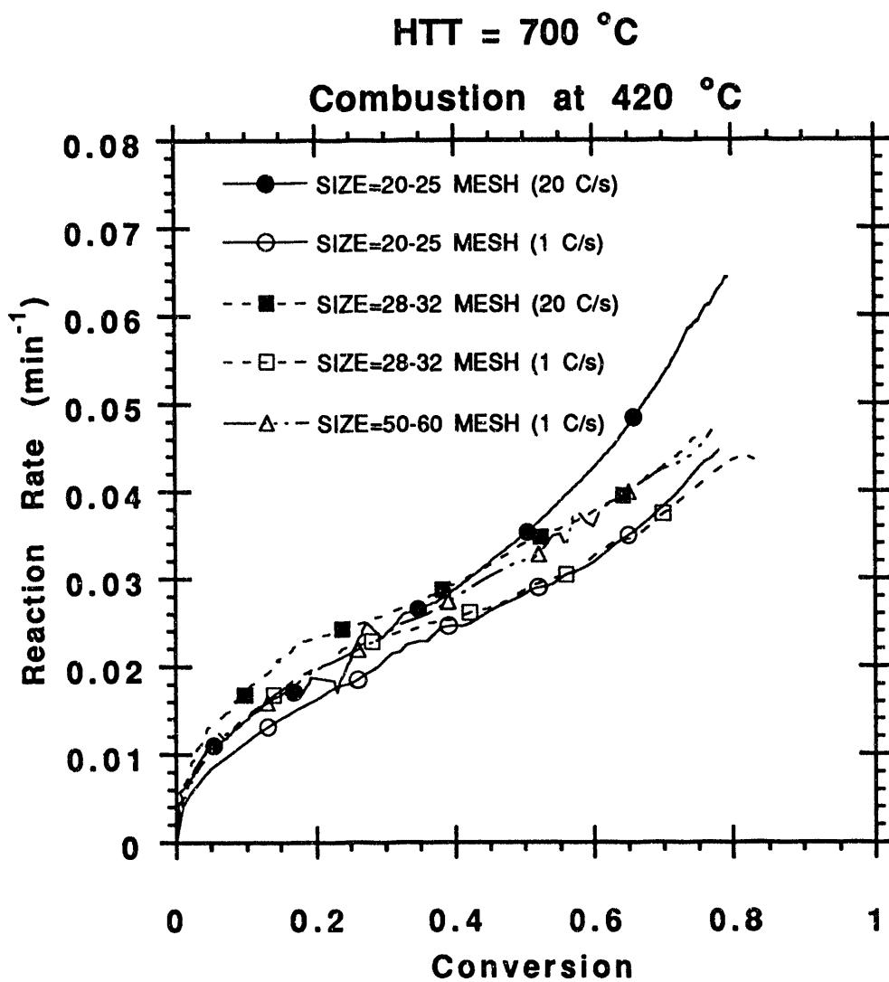
Figure 1: Intrinsic reaction rates for chars produced at various pyrolysis heating rates from coal particles of three different sizes. Heat treatment temperature for all runs is 700 °C.
