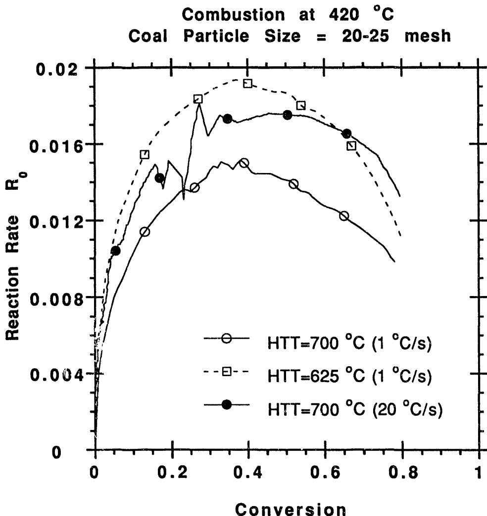
Figure 3: Reaction rate  $R_0$  vs. conversion patterns for chars produced at various pyrolysis heating rates and heat treatment temperatures from coal particles in the 20-25 mesh size range.
