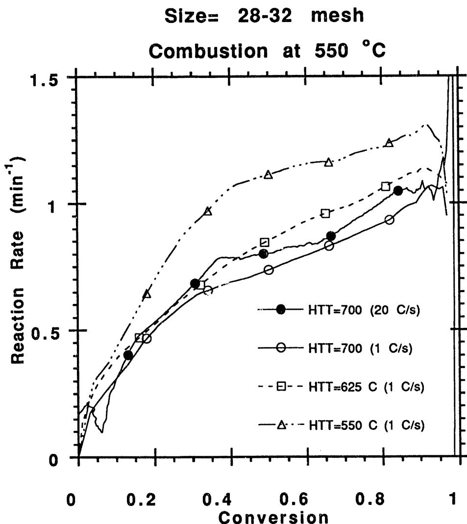
Figure 5: Reaction rate  $R_s$  vs. conversion patterns for combustion at 550 °C of chars produced at various pyrolysis heating rates and heat treatment temperatures. Coal particle size was in the 28-32 mesh range for all samples.
