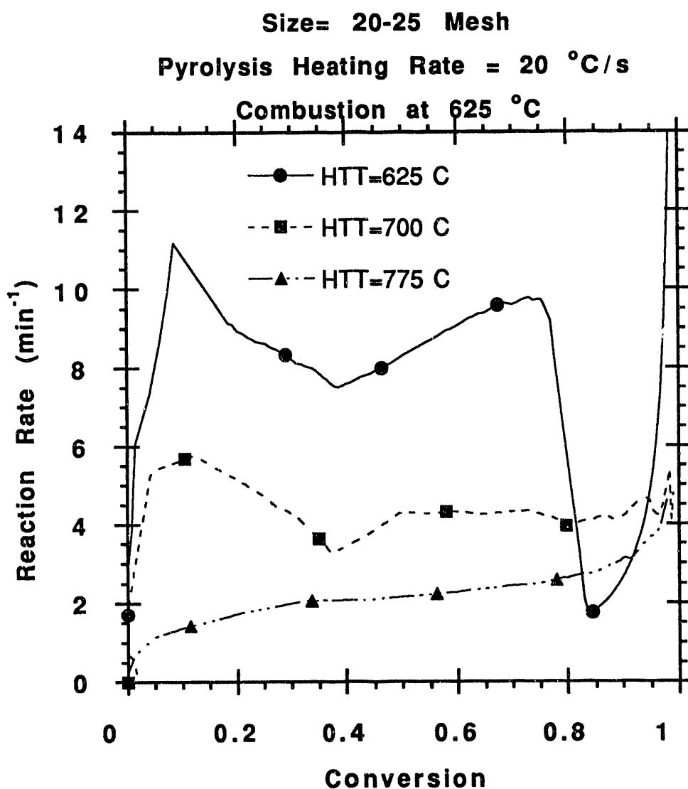
Figure 8: Reaction rate  $R_s$  vs. conversion patterns for combustion at 625 °C of chars produced at various heat treatment temperatures and a pyrolysis heating rate of 20 °C/s. Coal particle size was in the 20-25 mesh range for all samples.
