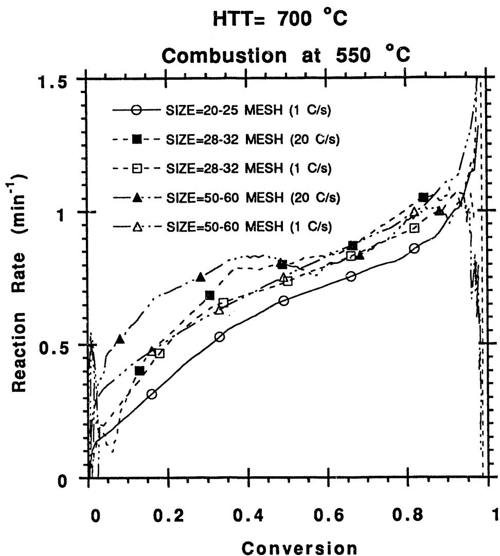
Figure 4: Reaction rate  $R_s$  vs. conversion patterns for combustion at 500 °C of chars produced at various pyrolysis heating rates from coal particles of three different sizes. Heat treatment temperature for all chars was 700 °C.
